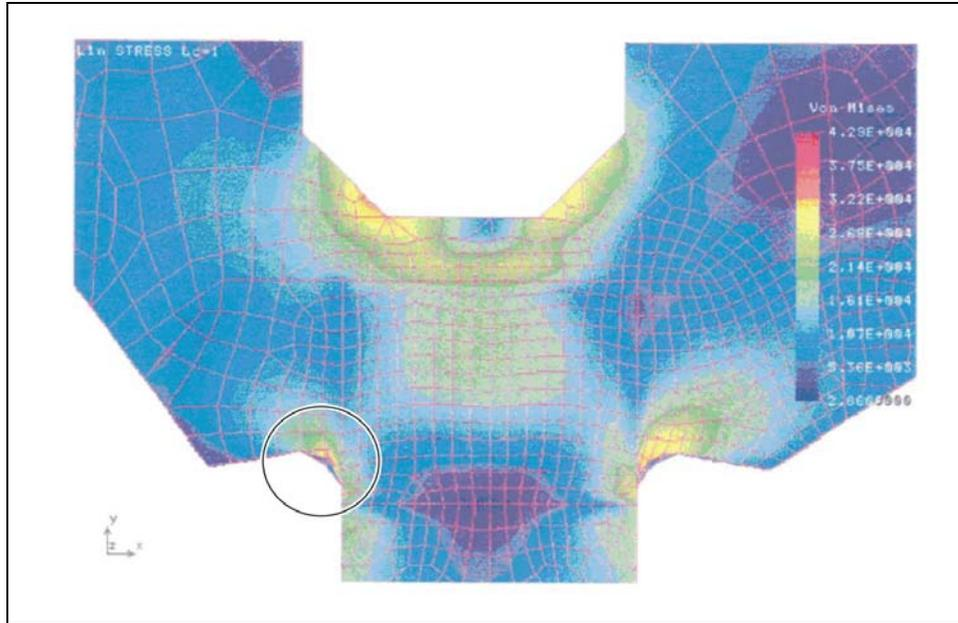
**Figure 4.** Stress in Transverse Bulkhead, Beam Sea, Sea State 5
