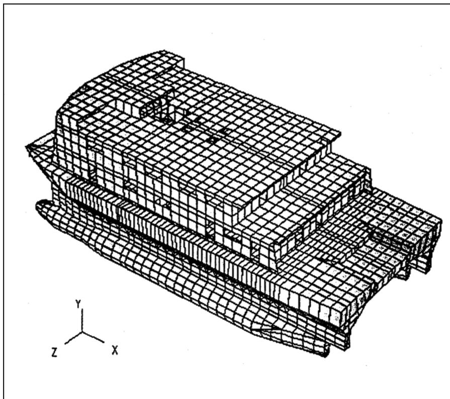
**Figure 5.** Global 3-D Finite Element Model
