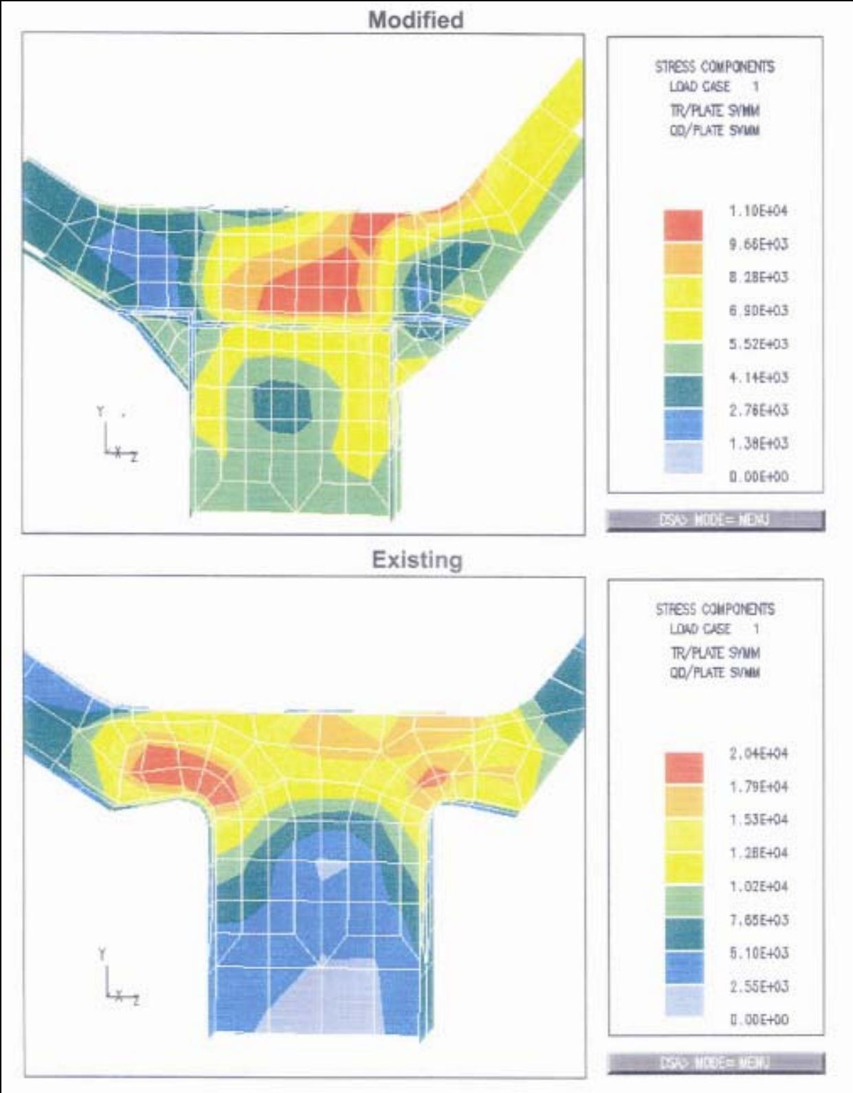
**Figure 7.** Haunch/Strut Stress with/without Fairing
