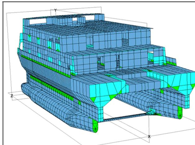
**Figure 8.** Global Model with Strut Installed
