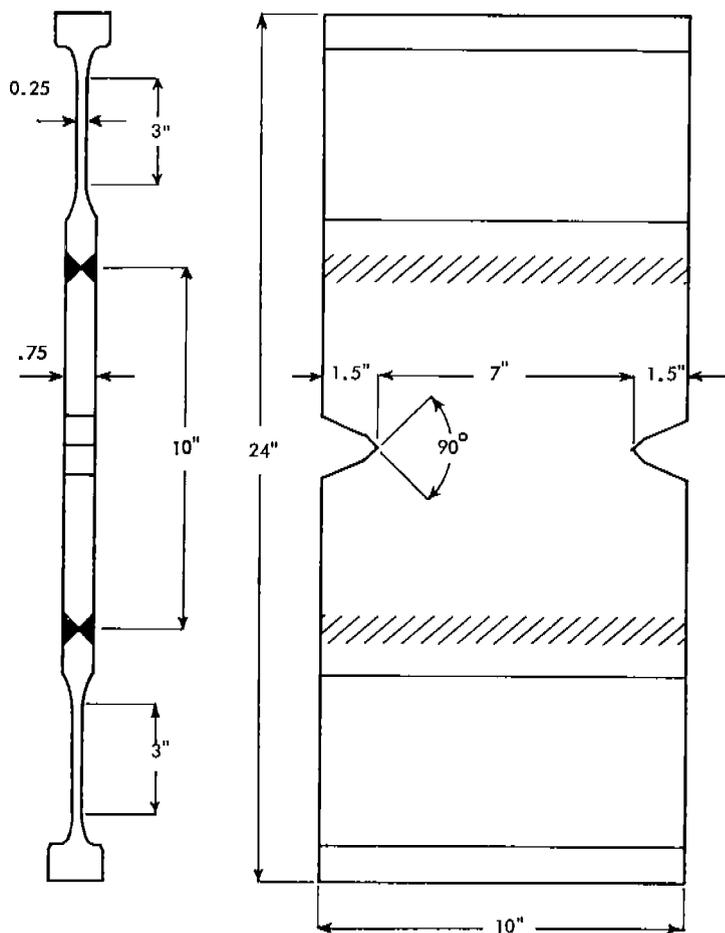
Fig. 1 10-in. test plate with plastic hinges
