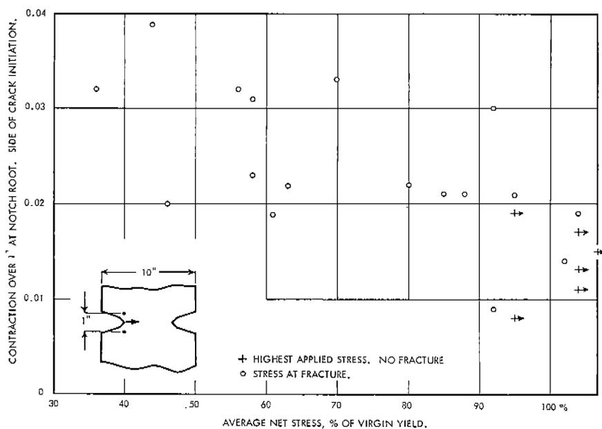
Fig. 8 Brittle-fracture results of longitudinally precompressed plates
