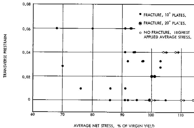
Fig. 9 Brittle-fracture results of transversely prestrained plates
