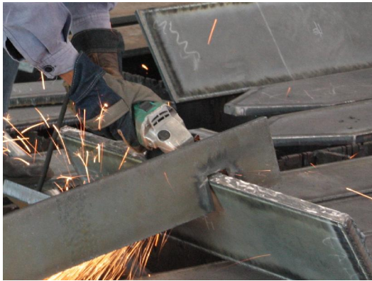
(a) Manual grinding (pre-treatment) for edges before sending to the edge rounding machine
