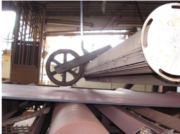
(a) Steel plate on roller conveyor
