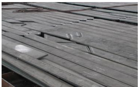
(a) Flange and web plates cut from steel plates for T-shape stiffeners Figure 5 Stiffeners used for ship structure
