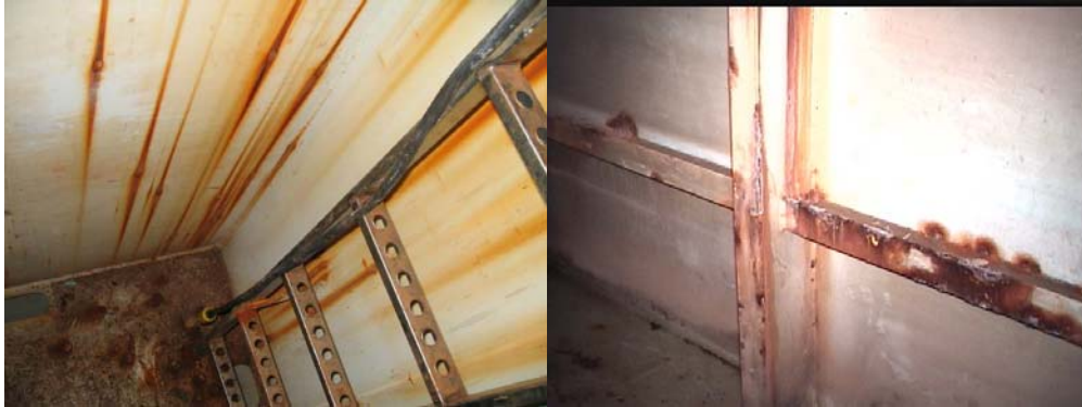
Figure 1 – Legacy Polyamide Epoxy Coatings Previously Favor for Navy Ship Tank Applications (approximately five years service)
