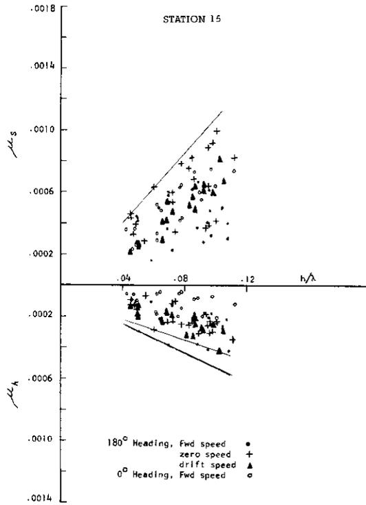
FIG. 63. BENDING MOMENTS VARIATION WITH WAVE HEIGHT. MODEL 2681-1. BOTH HEADINGS AND ALL WAVE LENGTHS AND SPEEDS.
