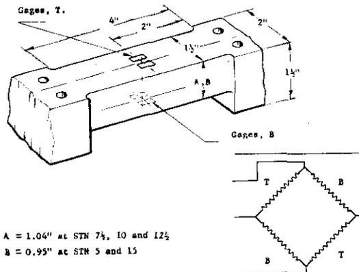
The four gages together formed a full Wheatstone Bridge circuit registering bending strains only.
