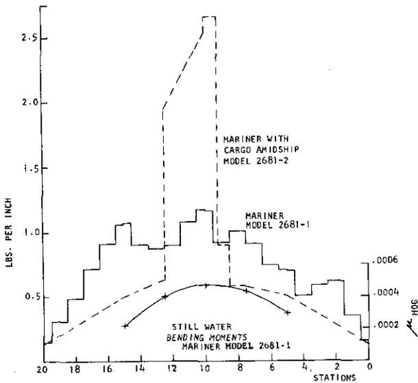
FIG. 5. WEIGHT DISTRIBUTION AND STILL WATER BENDING MOMENTS
