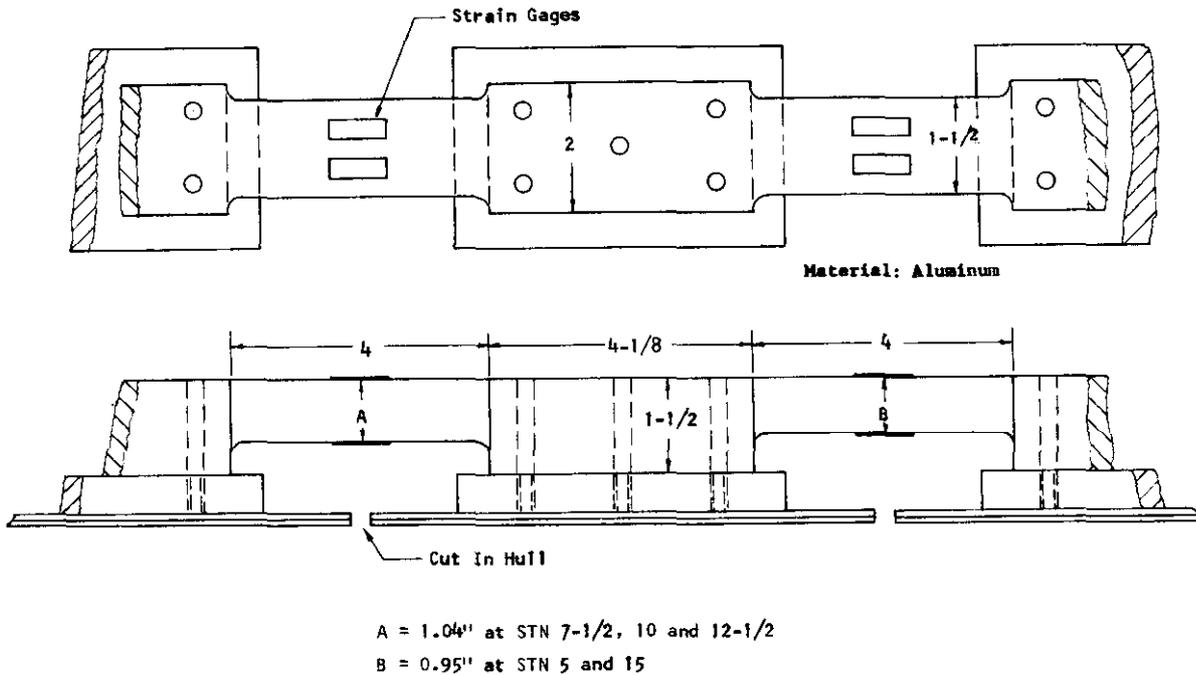
FIG. 4. STRUCTURAL BEAM
