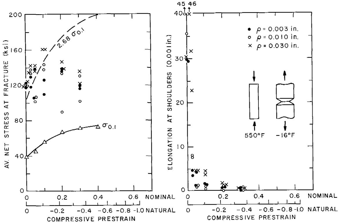
Fig. 11 Bars Axially Precompressed At 500°F, Grooved And Tested At - 16°F.
