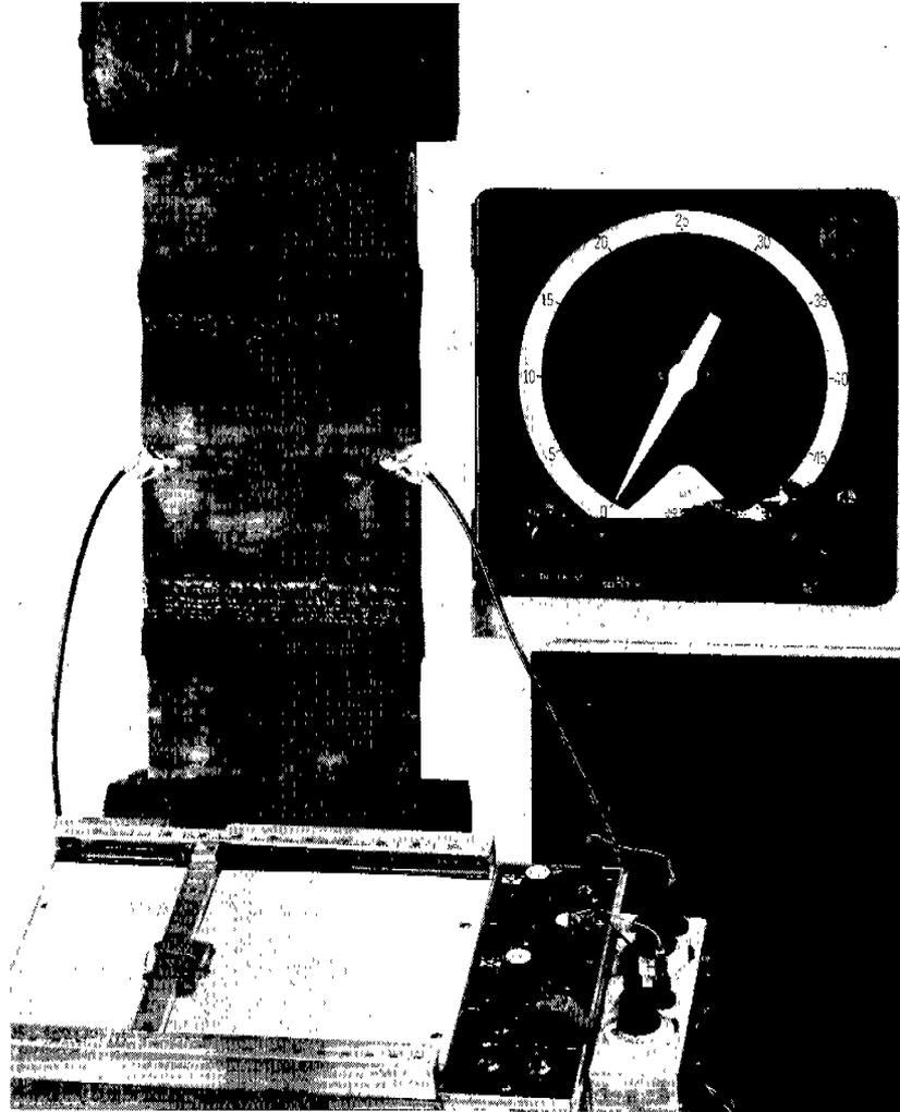
*Fig. 2 Notched Plate With Extensometers And Autographic Equipment.*
