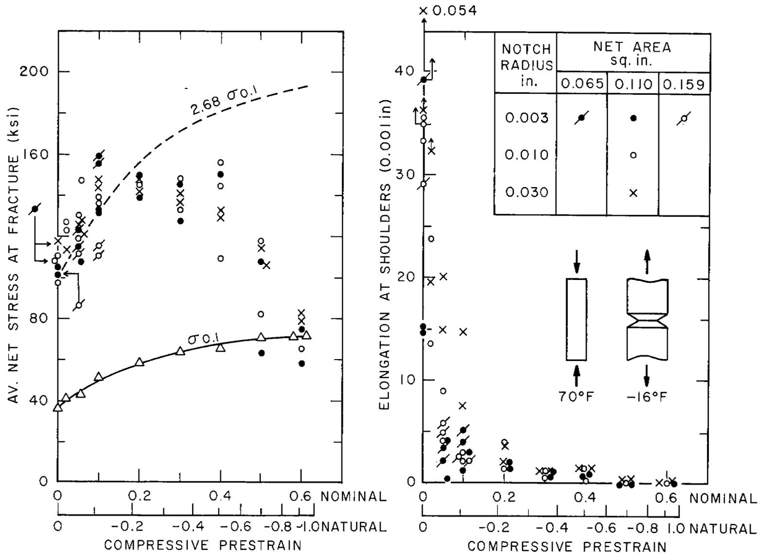
Fig. 8 Bars Axially Precompressed At 70°F, Grooved And Tested At -16°F.
