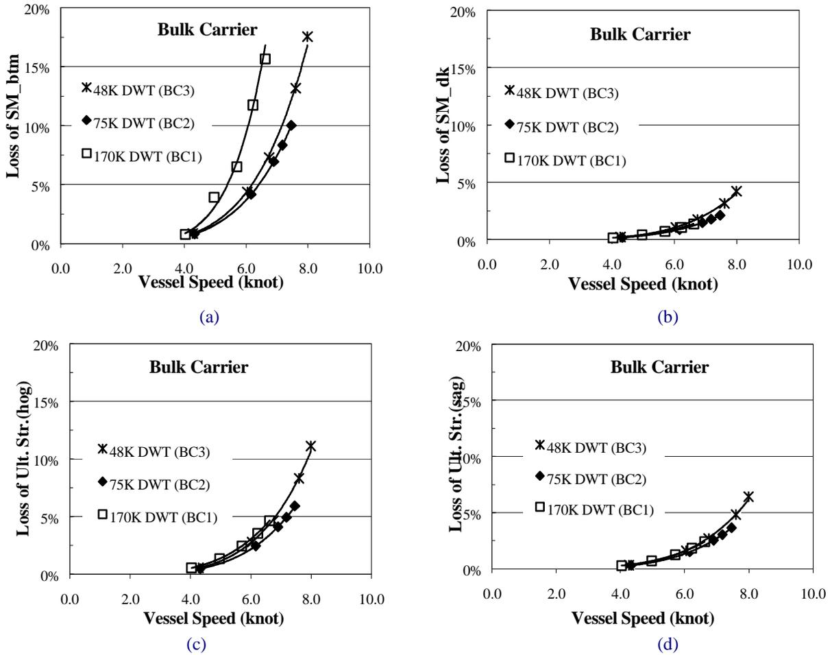
Figure 5 Bulk carriers: loss of hull-girder strength versus ship's speed
