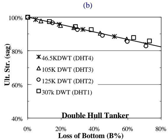
Figure 2 Double hull tankers: hull-girder residual strength versus transverse damage extent
