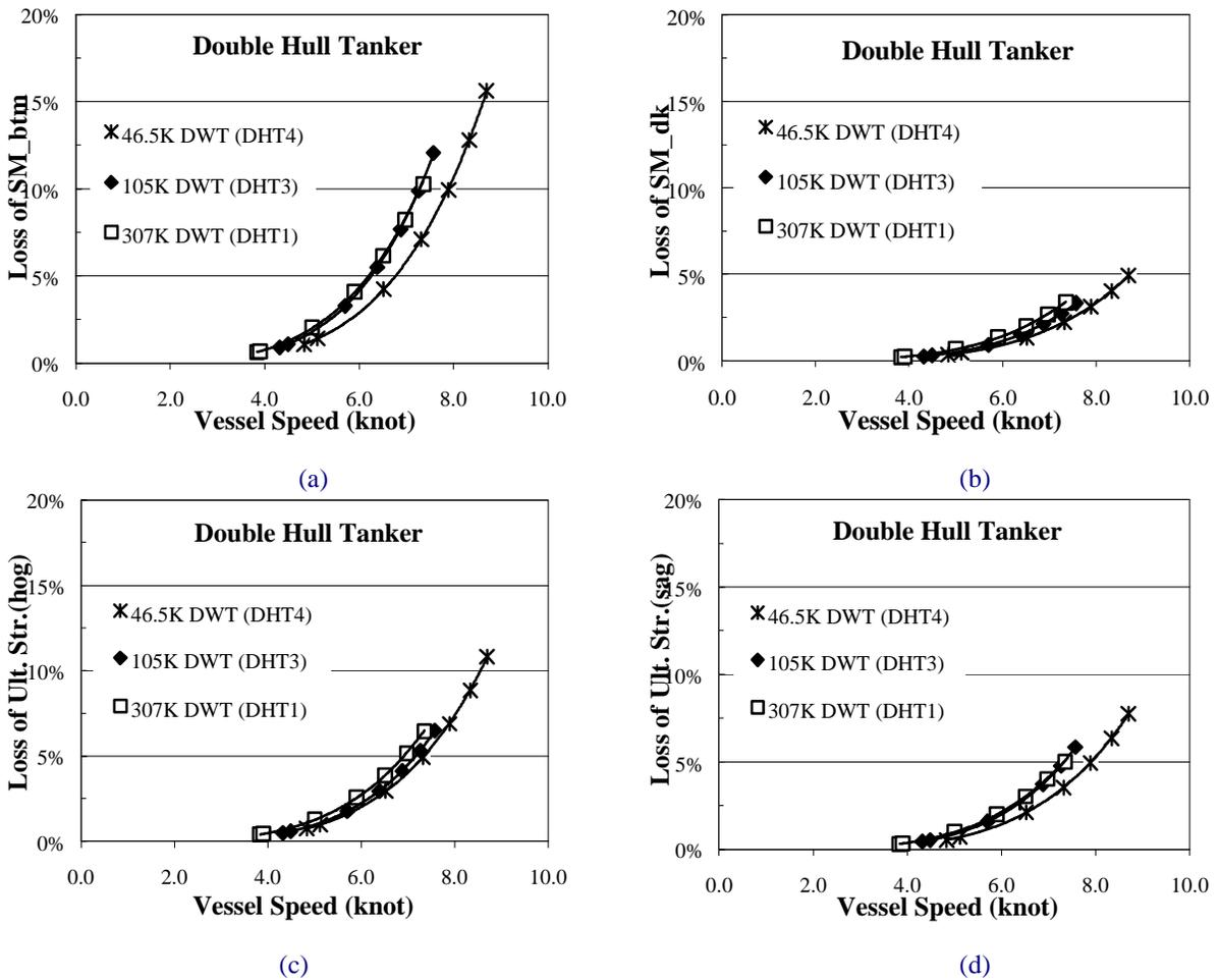
Figure 3 Double hull tankers: loss of hull-girder strength versus ship's speed
