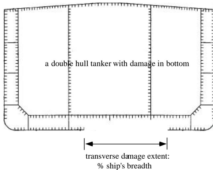
Figure 1 A double hull tanker with damage in bottom
