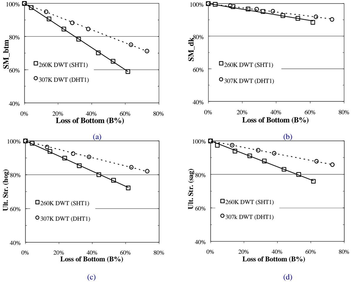
Figure 6 A single hull VLCC and a double hull VLCC: hull-girder residual strength versus transverse damage extent
