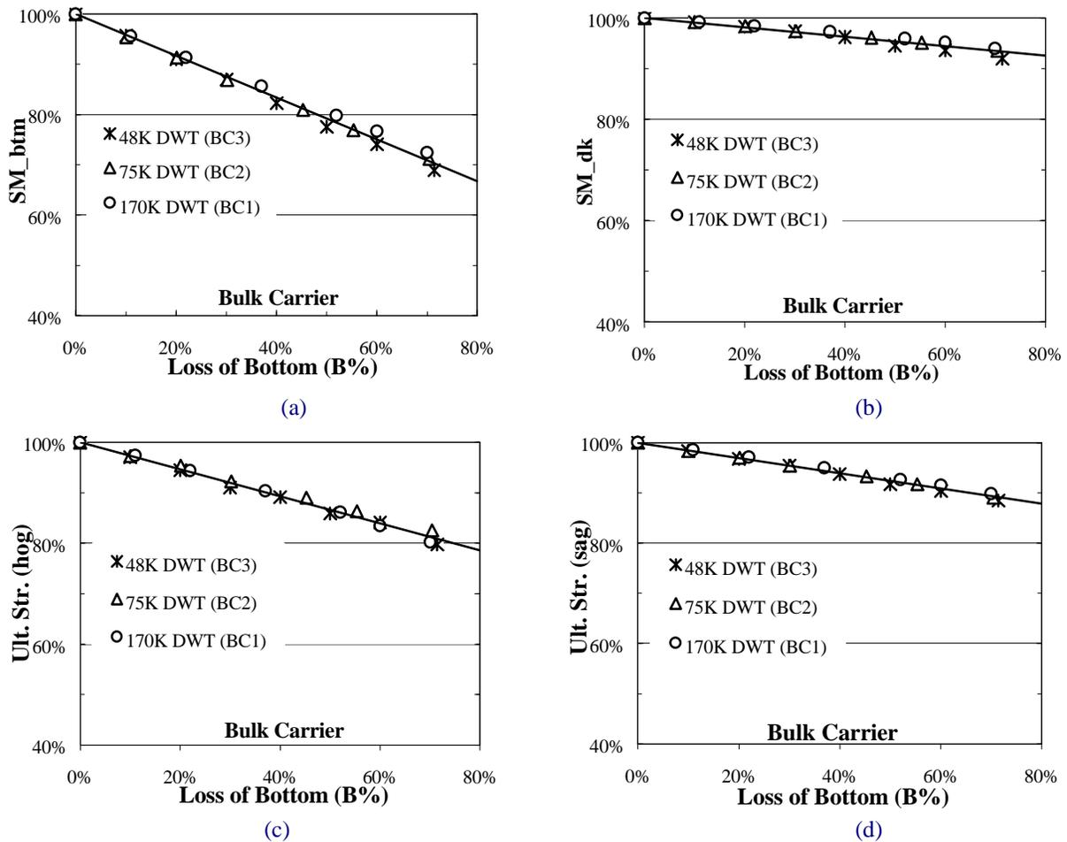
Figure 4 Bulk carriers: hull-girder residual strength versus transverse damage
