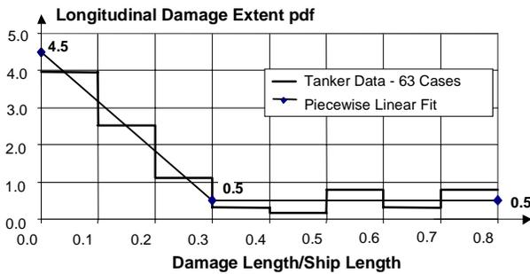
Figure 6 - Damage probability density function (pdf)
