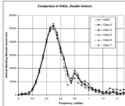
**Fig.2 Comparison of RAOs for Aframax Damage Cases**
