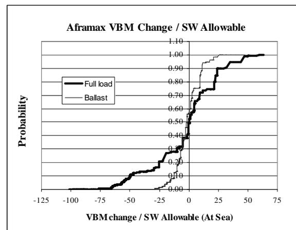
**Fig. 1: Change in Stillwater bending moment due to flooding after side damage**
