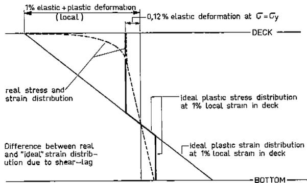
Fig. 5. Stress and Strain Distribution in the Side-Plating When 1% Strain Has Developed Over a Narrow Transverse Strip of Deck-Plating.
