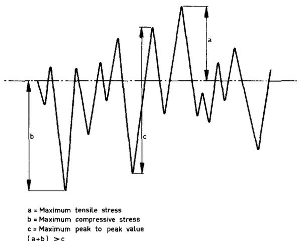
Fig. 3. Correction to Peak to Trough Values.
