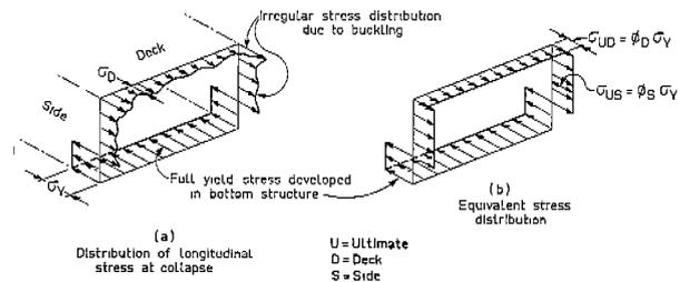
Fig. 6. Ultimate Stress Distributions-Buckling Included-Sagging Condition. (Caldwell<sup>9</sup>)
