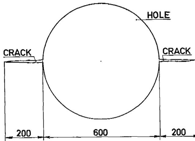
Fig. 14. Crack-Lengths 200 mm. Effective Crack-Length 1000 mm.
