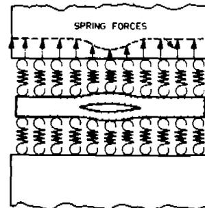
Fig. 13d. Model of Short Plate with Crack.
