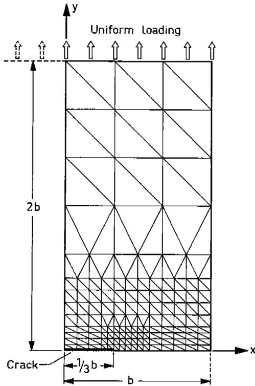
Fig. 15a. A Plate with a Semi-Crack in the Middle, Loaded Uniformly at the Ends. Only One-Quarter of the Idealized Plate is Shown (Using Trim 6 Elements). (Argyris, Patton<sup>13</sup>)
