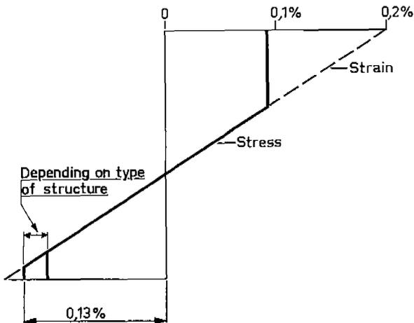
Fig. 10. Real Elasto-Plastic Strain Distribution in Contrast to that of Figure 6.
