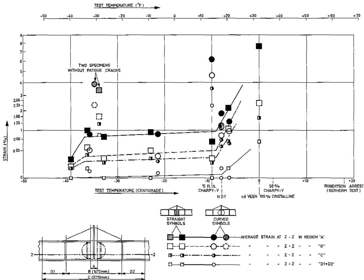
Fig. 12. Local and Overall Strains of a Specimen Containing Fatigue-Cracks at the Moment a Brittle Fracture Started.
