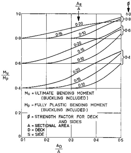
Fig. 7. Effect of Buckling on Ultimate Longitudinal Strength. Single Deck Ship, Sagging Condition. (Caldwell<sup>9</sup>)
