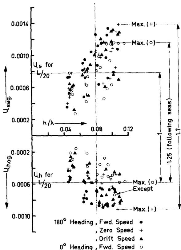
Fig. 4a. Bending Moments Variation with Wave Steepness (N.M. Maniar; E. Numata<sup>15</sup>) (Indications "Max" (o), (+) and Comparison Numbers 1, 1.25 and 1.7 on the Right are added).
