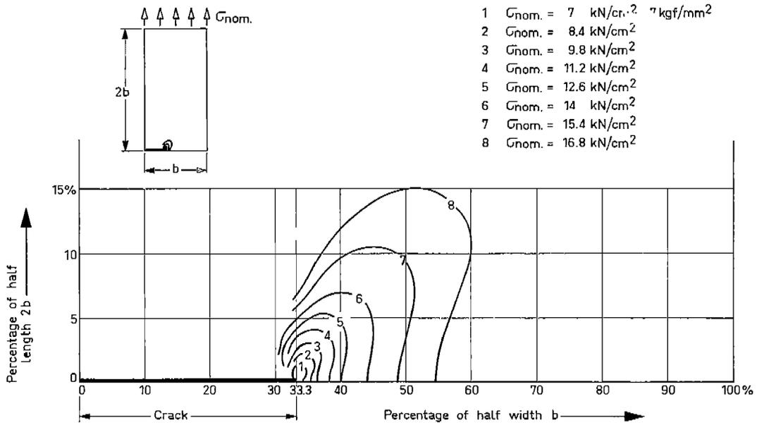
Fig. 15b. Development of the Area of Plastic Deformation in the Cracked Plate with Increasing Applied Load. (Argyris, Patton<sup>13</sup>)
