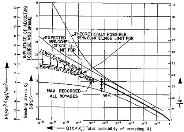
Fig. 2b. Original and Modified Long-Term Distributions with Respectively Theoretical and Supposedly More Realistic Confidence-Limits.
