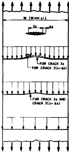
Fig. 13a. Stress Distribution in Long Plate Before and After Crack Extension.
