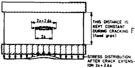
Fig. 13c. Model of Long Plate with Crack.
