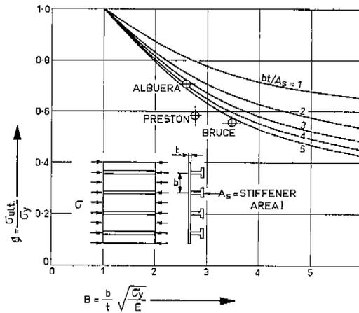
Fig. 8.  $\phi$ -Values for Stiffened Plating. (Faulkner<sup>9</sup>)
