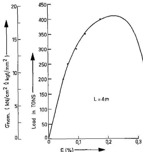
Fig. 11. Load-Deformation Curve of Compression Test.
