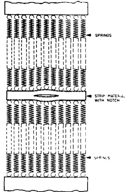
Fig. 13b. Stress Distribution at Loaded Edge of Short Plate, Before and After Crack Extension.
