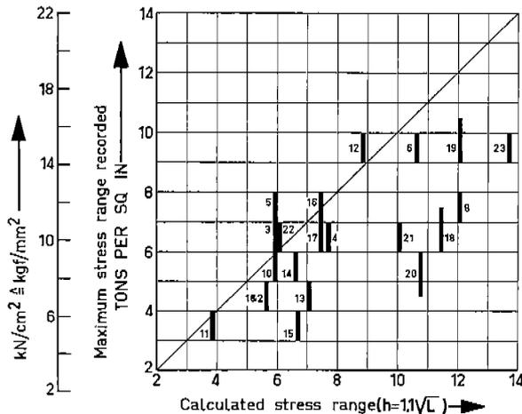
Fig. 1. Comparison of Calculated Stresses with Measured Maxima. (Johnson, Larkin<sup>6</sup>)
