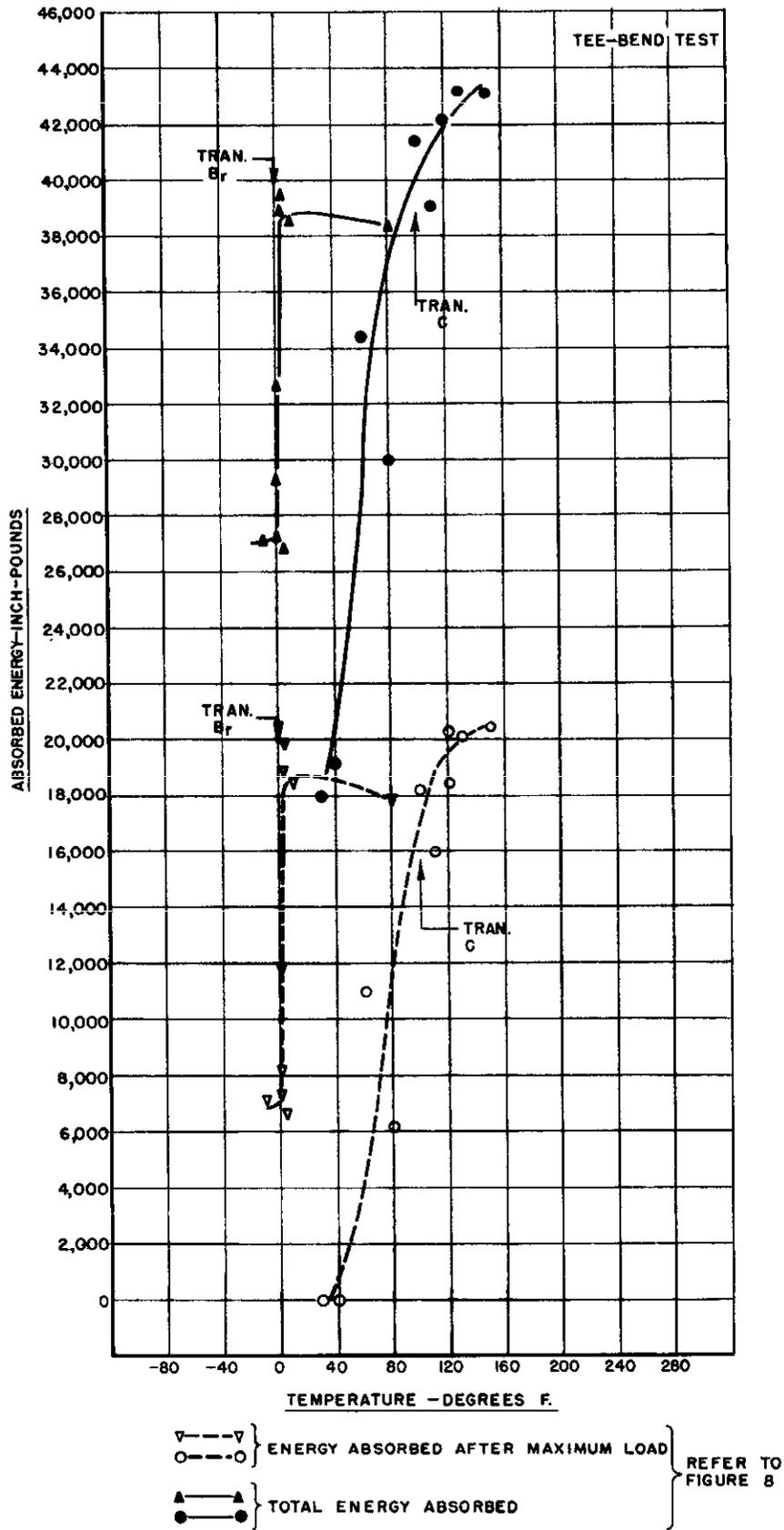
FIGURE II B. TRANSITION-TEMPERATURE CURVES FOR Br AND C STEELS BASED ON ABSORBED ENERGY
