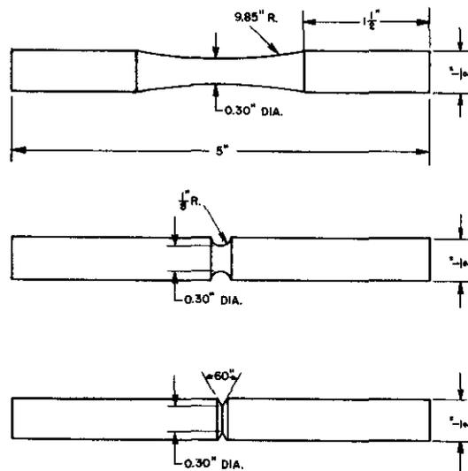
FIGURE 61. SPECIMENS FOR ROTATING BEAM FATIGUE TESTS.
