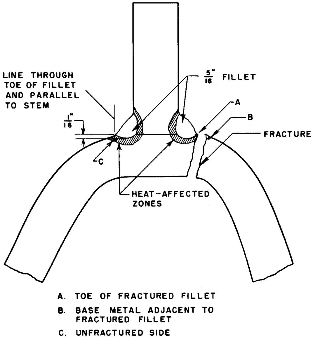
FIGURE 9. LOCATION OF POINTS FOR LATERAL CONTRACTION MEASUREMENTS ON TESTED TEE-BEND SPECIMENS.
