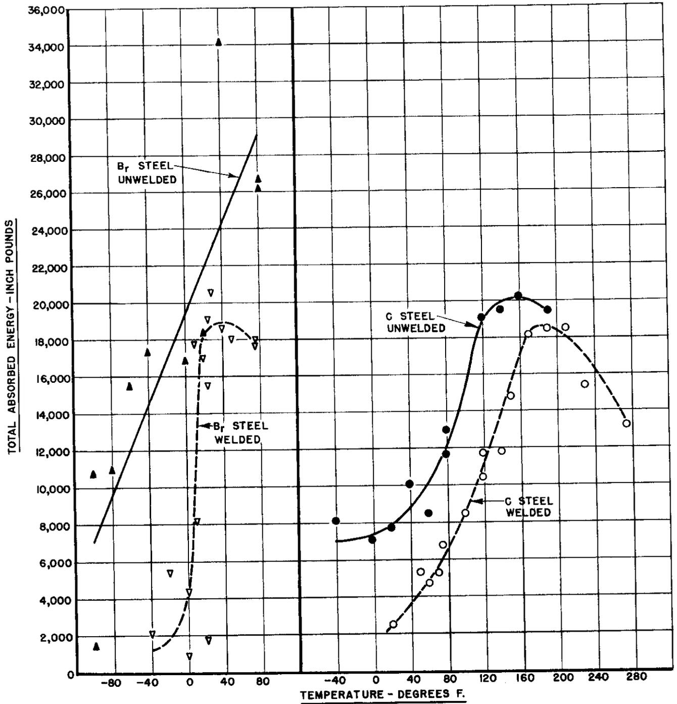
FIGURE 20A. A COMPARISON OF TRANSITION CURVES FOR WELDED AND UNWELDED KINZEL-TYPE SPECIMENS OF B<sub>7</sub> AND C STEELS.
