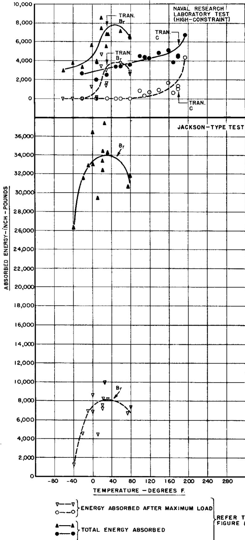
FIGURE II C. TRANSITION-TEMPERATURE CURVES FOR Br AND C STEELS BASED ON ABSORBED ENERGY
