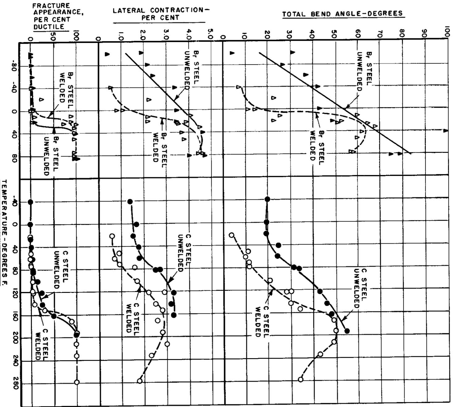
FIGURE 20B A COMPARISON OF TRANSITION CURVES FOR WELDED AND UNWELDED KINZEL-TYPE SPECIMENS OF B7 AND C STEELS.
