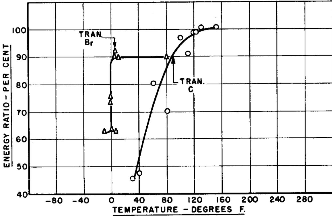
FIGURE 15. TRANSITION-TEMPERATURE CURVES FOR Br AND C STEELS BASED ON THE ENERGY ABSORPTION RATIO OBTAINED FROM TEE-BEND TESTS
