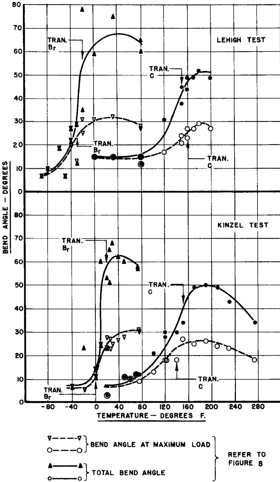
FIGURE 12 A. TRANSITION-TEMPERATURE CURVES FOR Br AND C STEELS BASED ON BEND-ANGLE MEASUREMENTS
