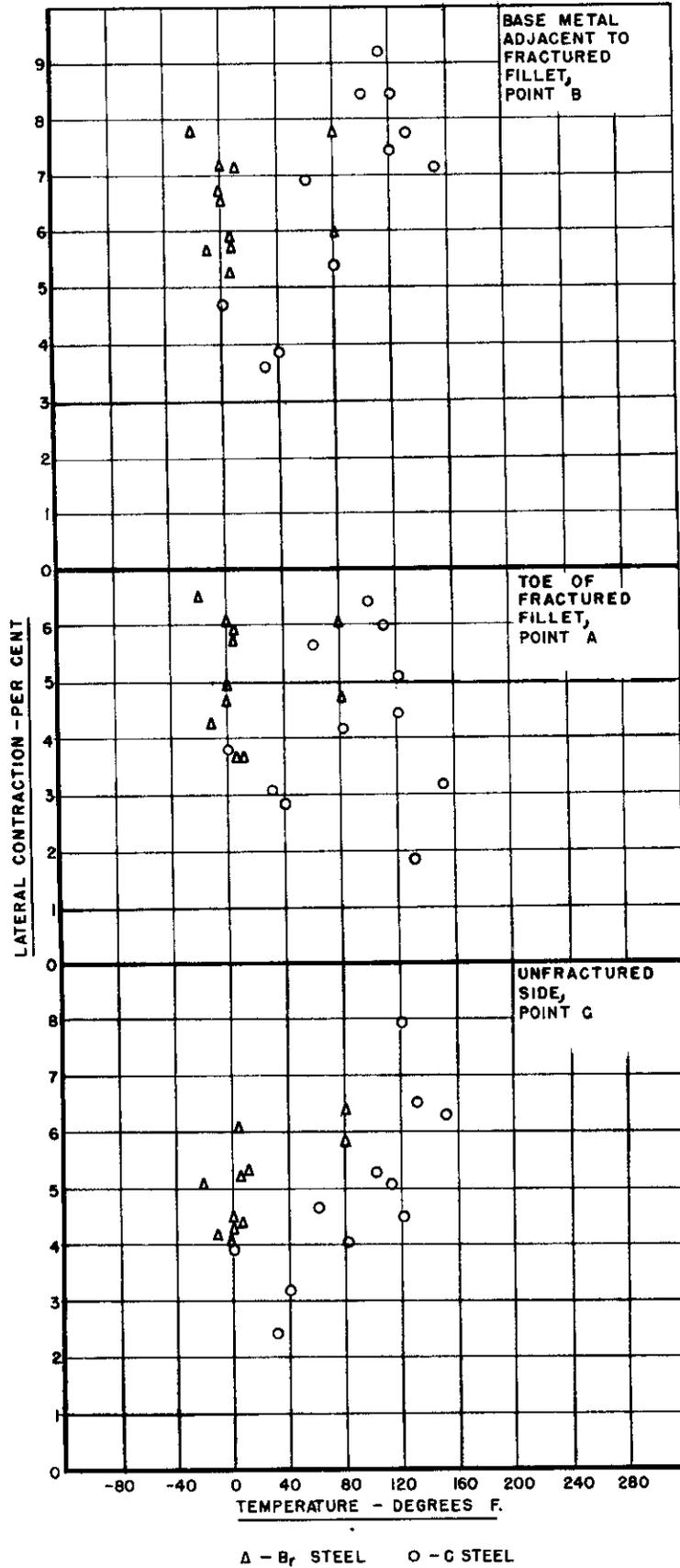
FIGURE 10. A COMPARISON OF LATERAL CONTRACTION MEASUREMENTS AT THREE LOCATIONS ON THE TEE-BEND SPECIMENS. REFER TO FIGURE 9.
