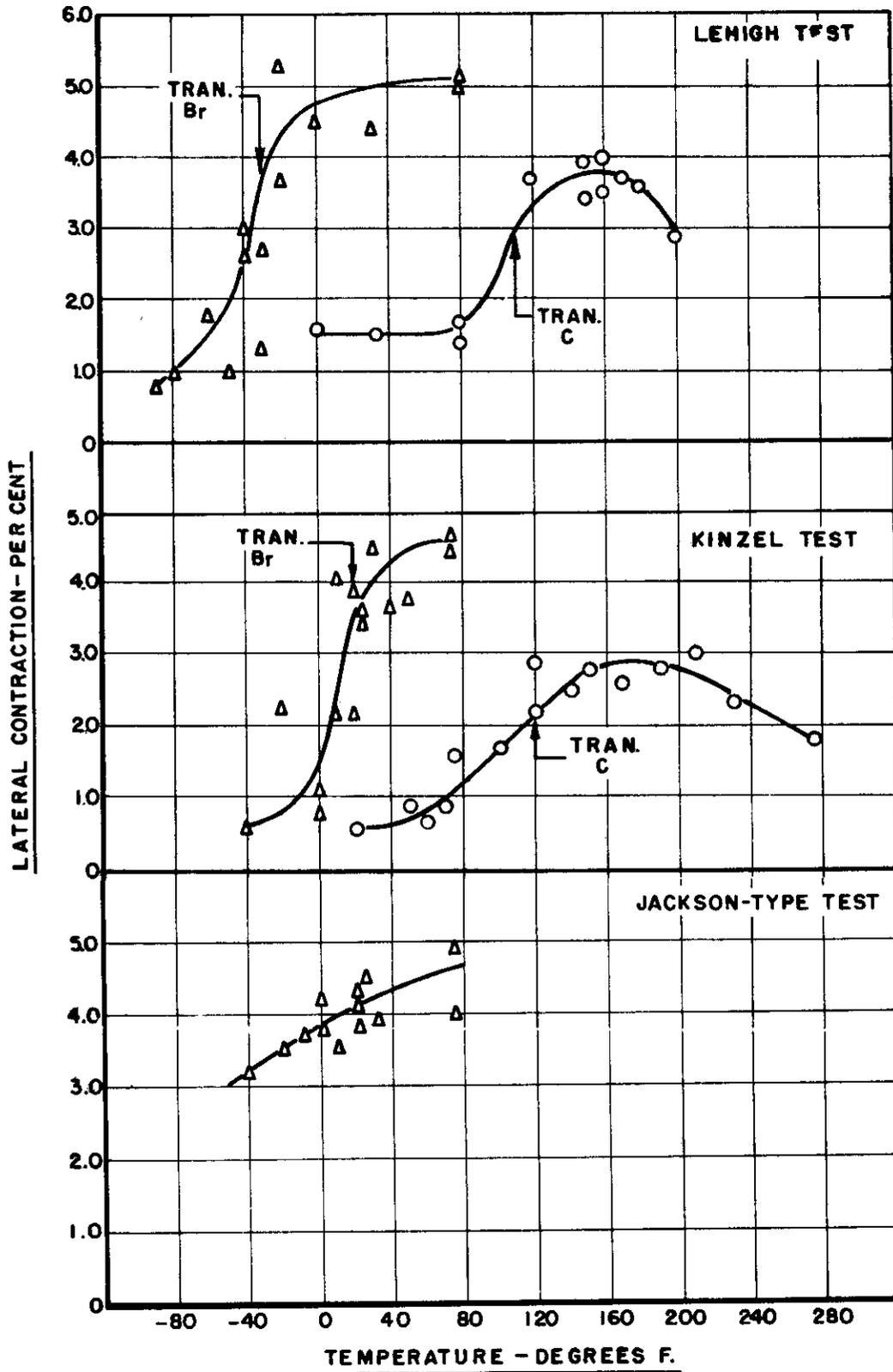
FIGURE 13. TRANSITION-TEMPERATURE CURVES FOR Br AND C STEELS BASED ON LATERAL-CONTRACTION MEASUREMENTS
