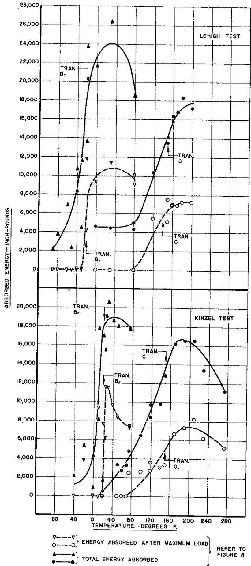
FIGURE II A. TRANSITION-TEMPERATURE CURVES FOR Br AND C STEELS BASED ON ABSORBED ENERGY
