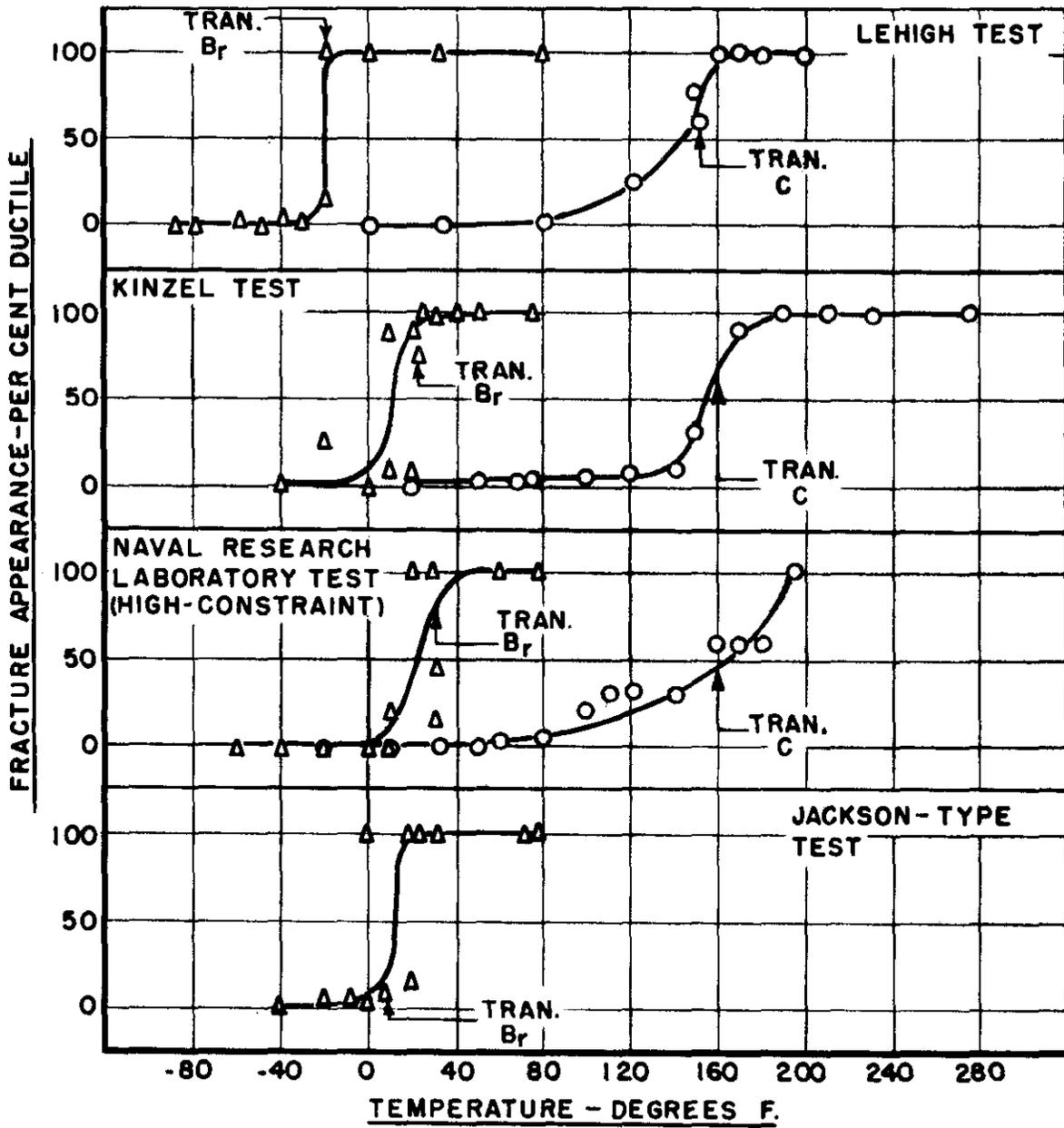
FIGURE 14. TRANSITION-TEMPERATURE CURVES FOR B<sub>r</sub> AND C STEELS BASED ON FRACTURE APPEARANCE
