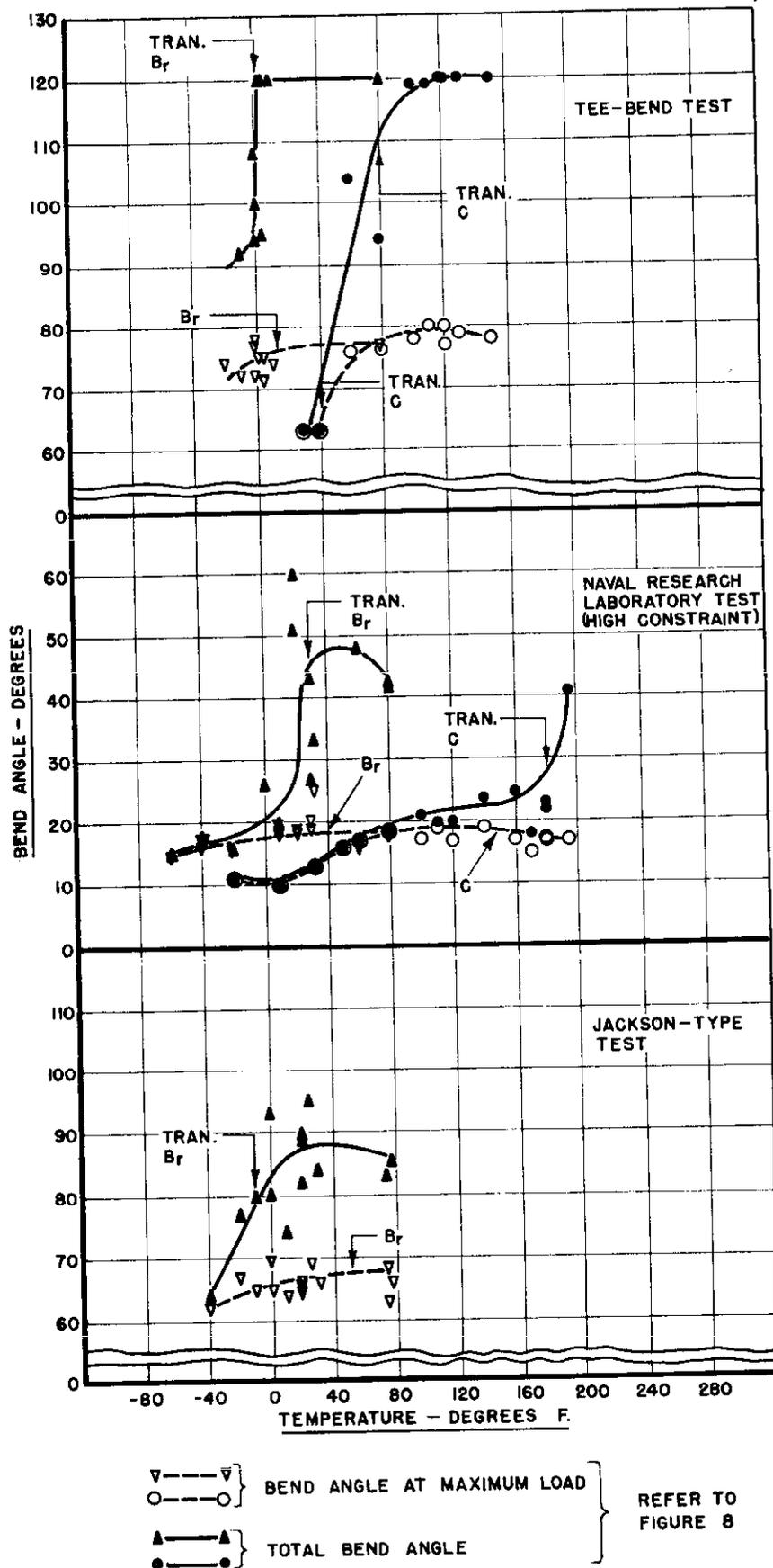
FIGURE 12 B. TRANSITION-TEMPERATURE CURVES FOR Br AND C STEELS BASED ON BEND-ANGLE MEASUREMENTS.
