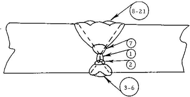
Fig. 2. Typical Welding Sequence
