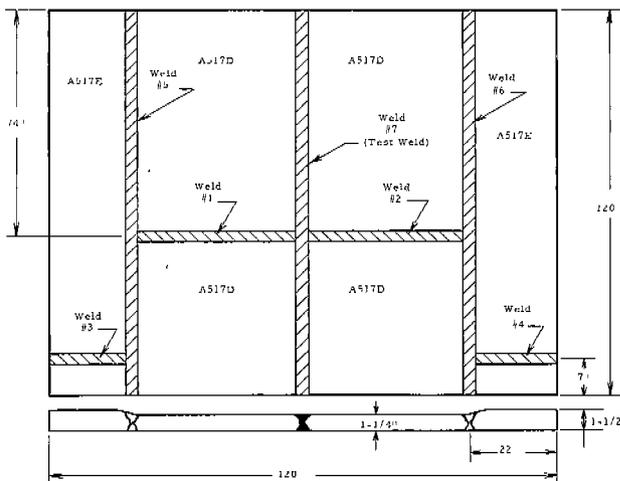
Fig. 9. Fabrication Sequence for 120-Inch Test Specimen
