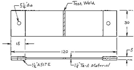
Fig. 6. Basic 30-Inch Wide Test Specimen
