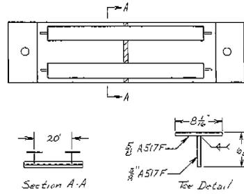
Fig. 7. Tee-Stiffened 30-Inch Wide Test Specimen
