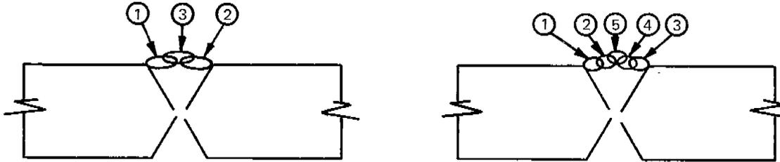
**Tacking:** For sub-arc welding, tacks shall be made using E 8018-C3 electrodes. These tacks shall be made so they can be incorporated in the seal weld.
