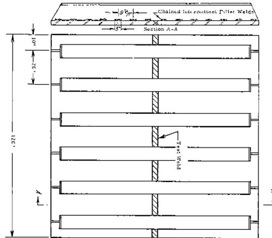
Fig. 10. Location of Tee-Stiffeners on 120-Inch Specimen
