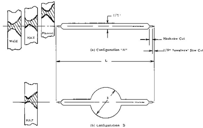
Fig. 8. Through-Wall Flaw Configurations
