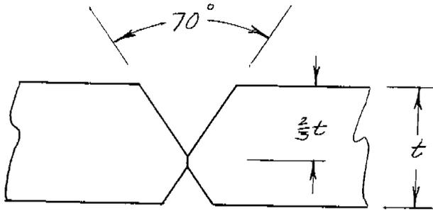
Fig. 1. Typical Weld Joint Design
