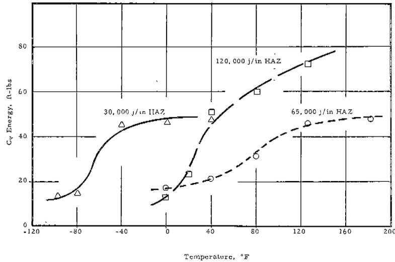
Fig. 5. Effect of Heat Input on Impact Properties of the HAZ of 1- $\frac{1}{4}$ " A517D Submerged Arc Weldments
