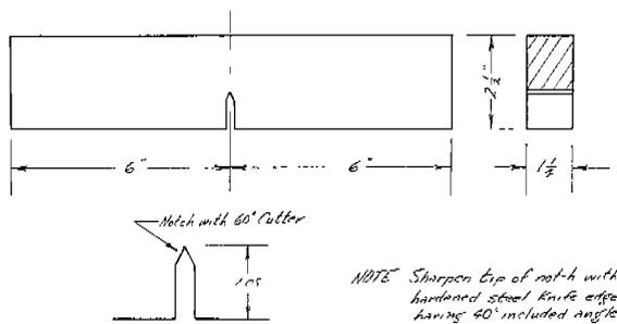
Fig. 13. Notched Impact Test Specimen
