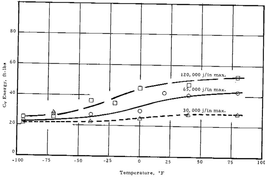
Fig. 3.  $C_v$  Energy Data on Sub-Arc Deposited Weld Metal
