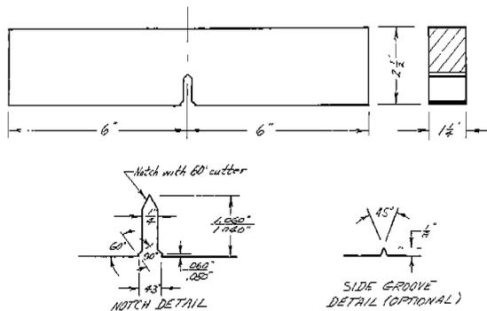
Fig. 12. Slow Bend Fracture Toughness Specimen
