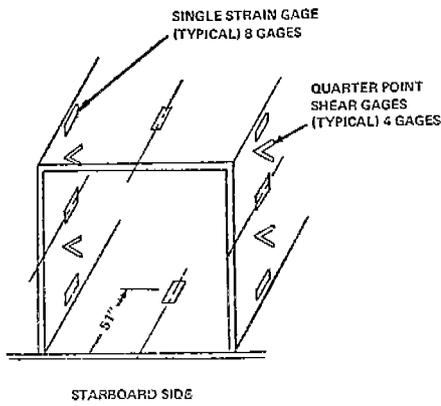
FIGURE A-8 – TRANSVERSE BEAM GAGE LOCATIONS AT FRAMES 194-195
