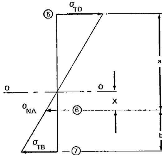
Figure C-2 - TORSIONAL BENDING STRESS
