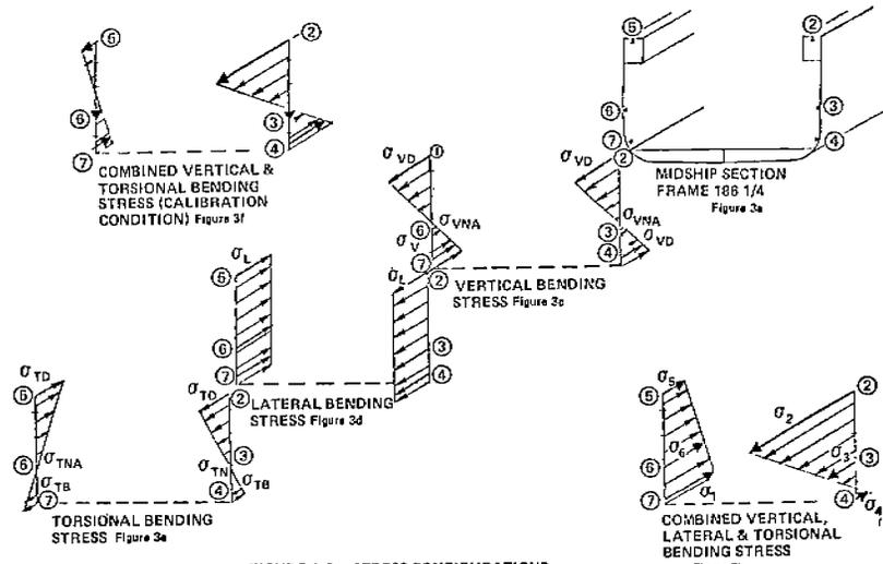
FIGURE A-3 - STRESS CONFIGURATIONS
