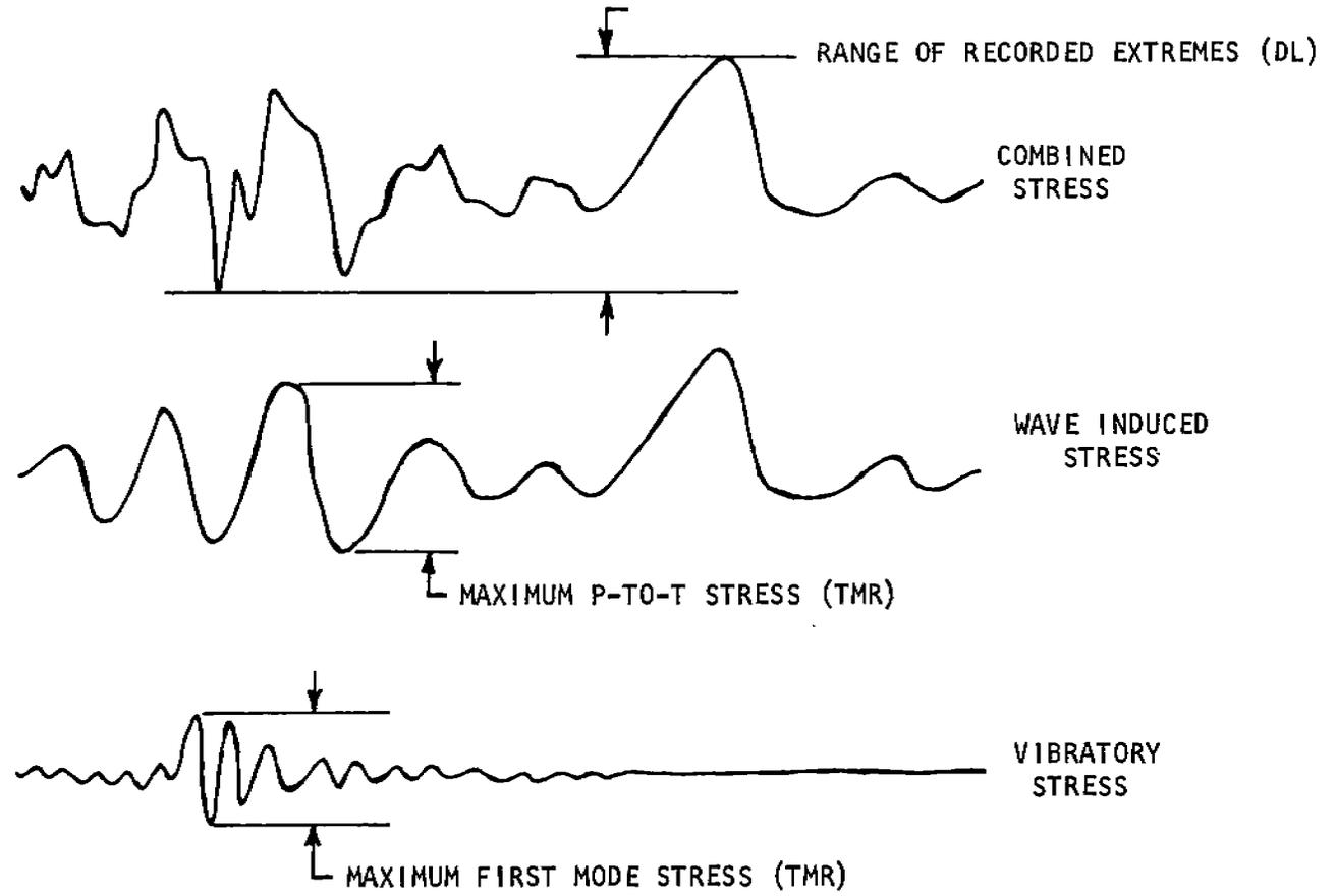
FIGURE 1 SKETCH ILLUSTRATING MAXIMUM STRESS PARAMETERS
