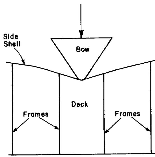
(a) Deformation or Buckling Failure Mode in References [33] and [38]
