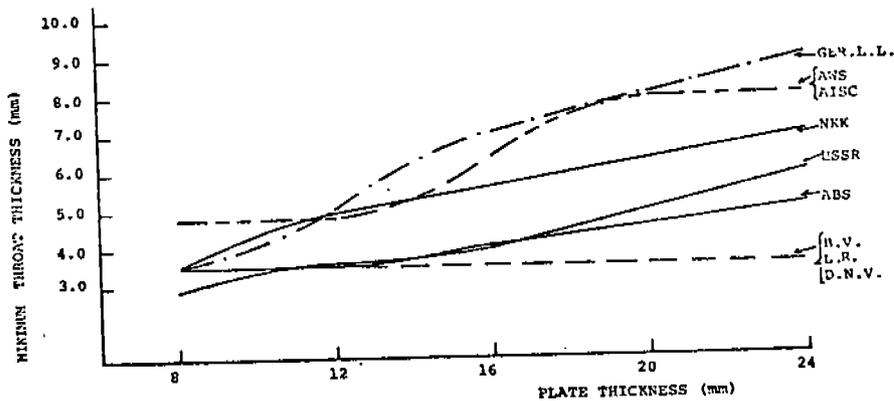
FIGURE 3.2d CURRENT WELDING REQUIREMENTS FOR JOINTS BETWEEN STIFFENERS AND NON-TIGHT STRUCTURAL BULKHEADS
