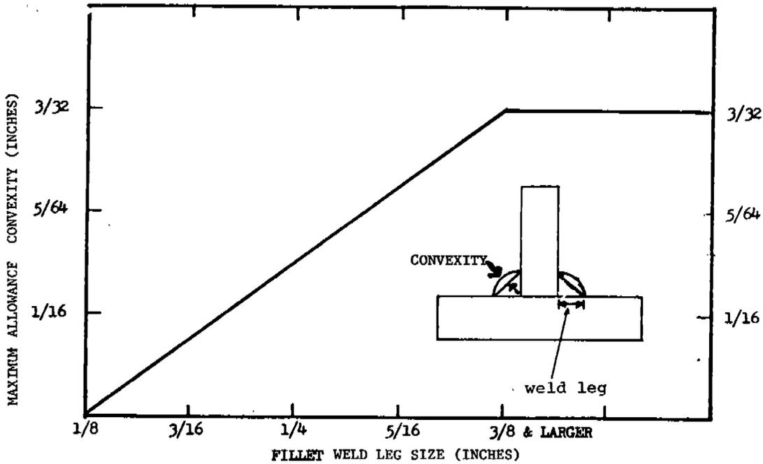
FIGURE 3.8 MAXIMUM ALLOWABLE CONVEXITY FOR FILLET WELD SIZES (19)
