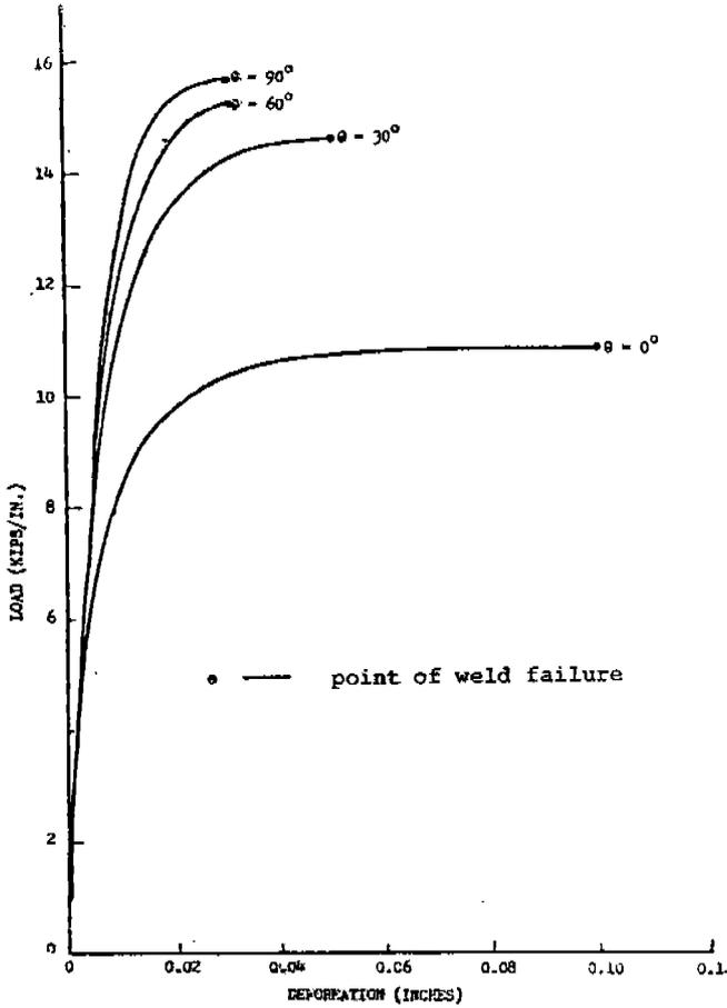
FIGURE 2.2 LOAD VS. DEFORMATION
