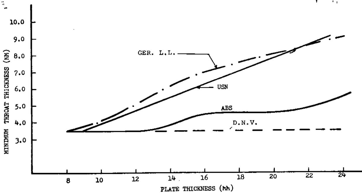
FIGURE 3.6 CURRENT WELDING REQUIREMENTS FOR JOINTS BETWEEN WEB FRAMES AND SHELL PLATING
