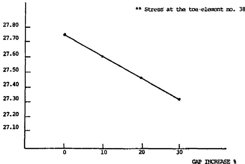
FIGURE 4.11 STRESS CONCENTRATION AT THE TOE ELEMENT
