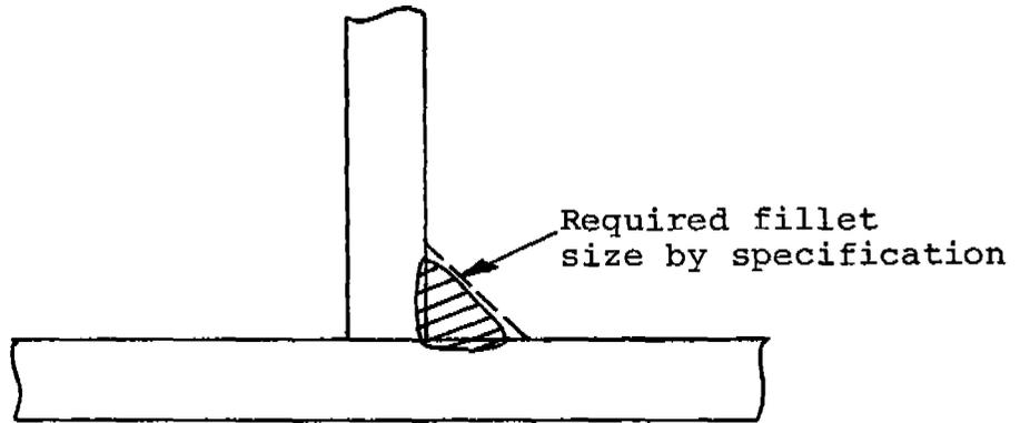
a. Slightly Undersized Fillet Weld
