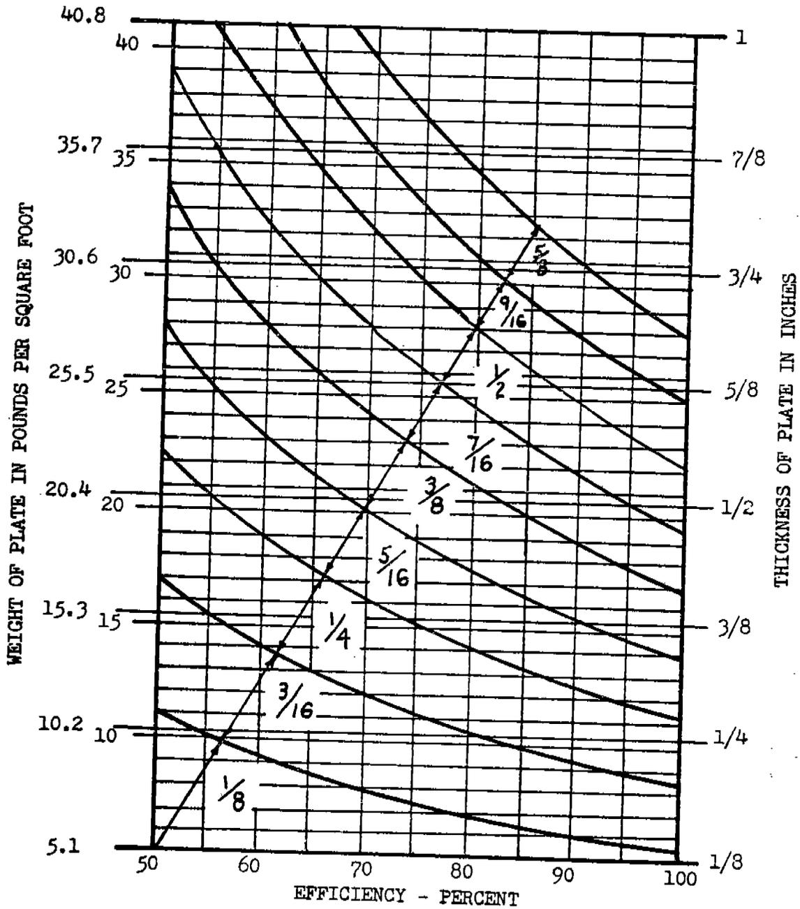
FIGURE 3.4 EFFICIENCY CHART FOR CONTINUOUS DOUBLE-FILLET WELDED TEE JOINTS MADE BETWEEN MEDIUM STEEL WITH MIL-6011 ELECTRODES<sup>(19)</sup> BASED ON THE THINNEST OF THE TWO PLATES JOINED
