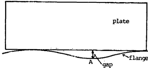
FIGURE 4.10 GAP FORMATION IN A FILLET WELD
