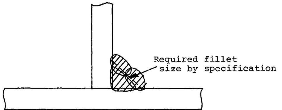
b. Overwelded Fillet Joint as a Result of Additional Welding Two Passes
