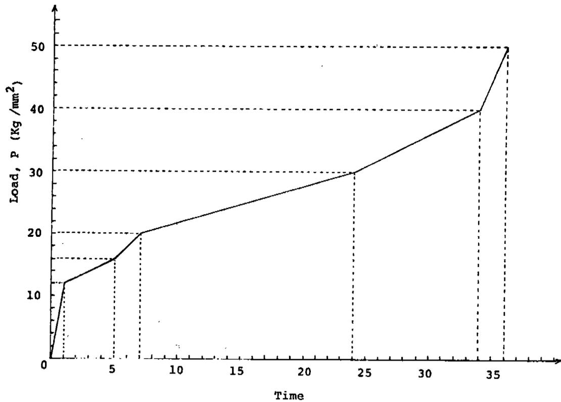
FIGURE 4.5 LOADING FUNCTION FOR TEST RUN
