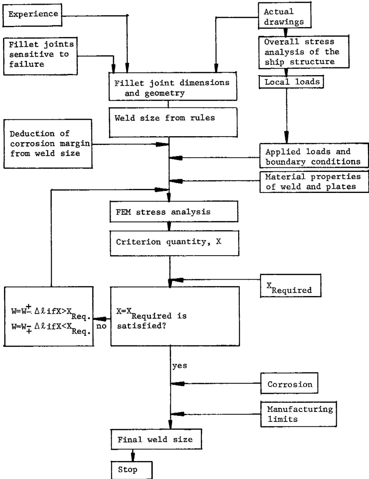
FIGURE 4.2 PROCESS FOR DETERMINING MINIMUM FILLET WELD SIZE
