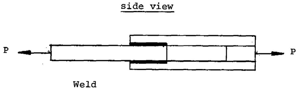
FIGURE 2.1 SCHEMATIC REPRESENTATION OF THE TEST SPECIMEN (9)
