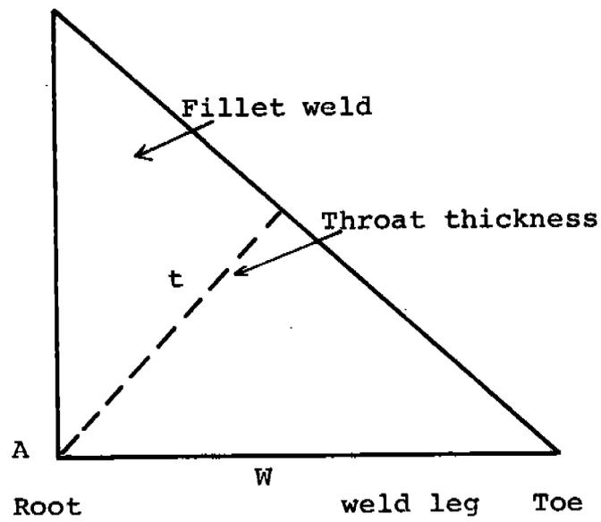
FIGURE 3.1 DEFINITION OF BASIC PARAMETERS IN FILLET WELDS
