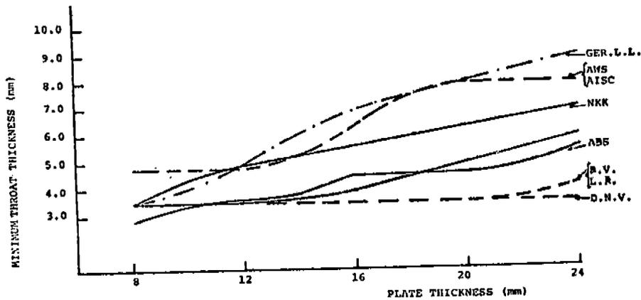
FIGURE 3.2c CURRENT WELDING REQUIREMENTS FOR JOINTS BETWEEN WEB FRAMES AND SHELL PLATING
