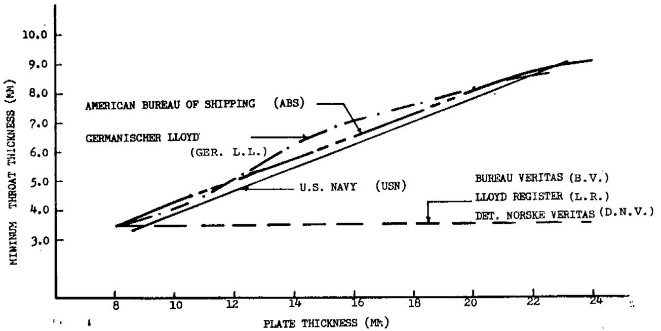
FIGURE 3.5 CURRENT WELDING REQUIREMENTS FOR JOINTS BETWEEN DOUBLE BOTTOM FLOORS AND SHELL PLATING
