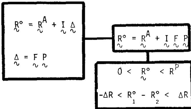
$\vec{R}^o$  : vector of bearing reactions during operation
