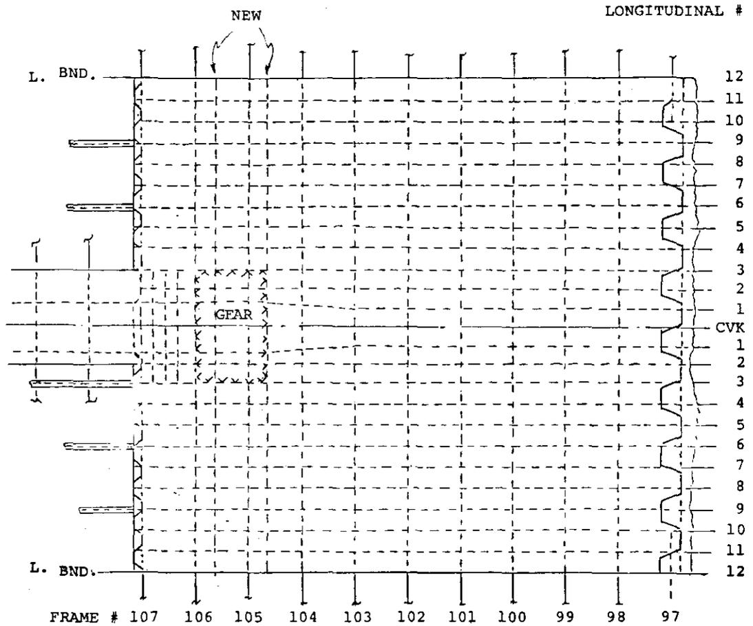
TWO ADDITIONAL FLOORS SUPPORT THE GEAR FOUNDATION
