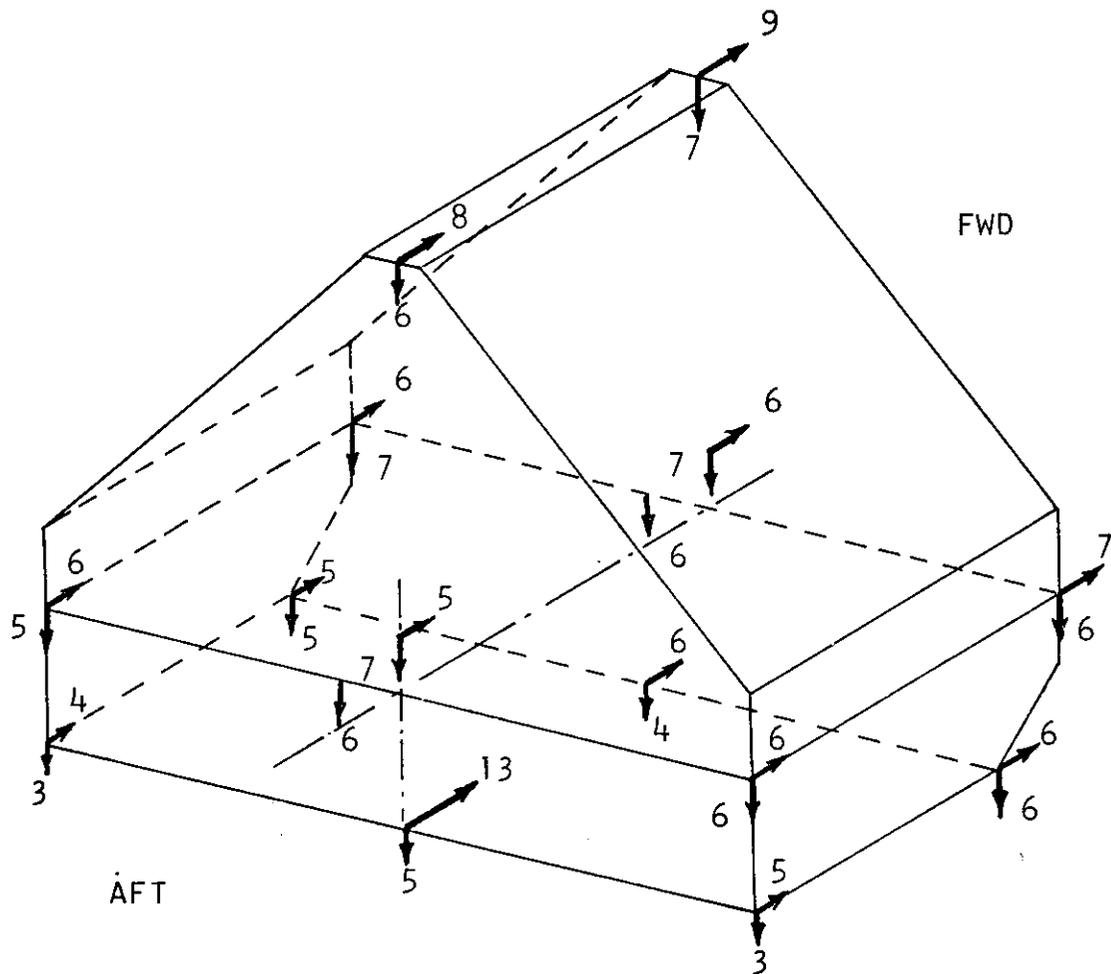
3 MIL VALUES AT LOWER AFT CORNERS ARE INVALID DUE TO POOR INDICATOR MOUNTING
