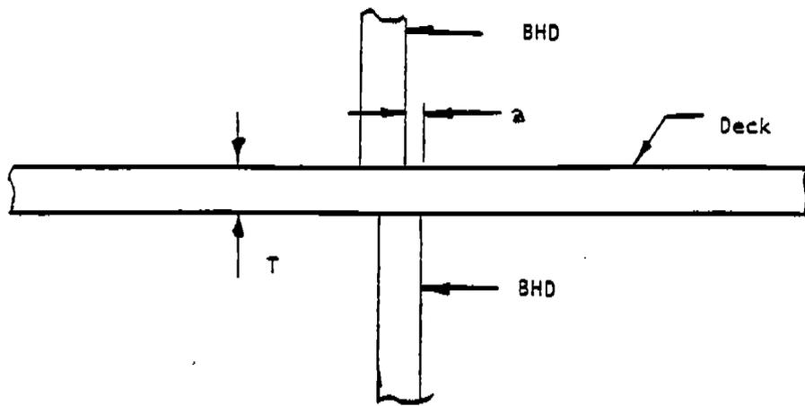
Figure 4: BULKHEAD MISALIGNMENT
