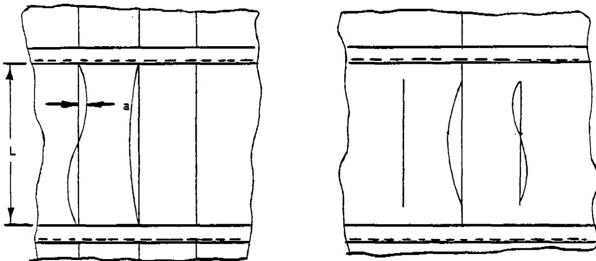
Figure 12: DISTORTION IN PANEL STIFFENERS
