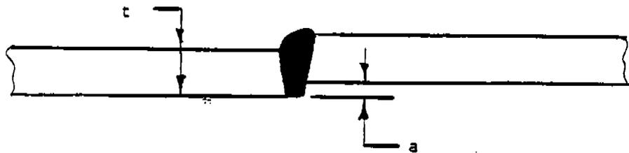
Figure 5: MISALIGNMENT OF BUTT CONNECTIONS
