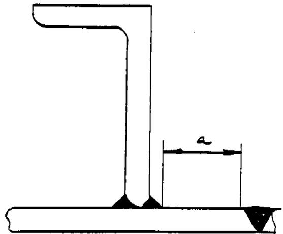
Figure 10: DISTANCE BETWEEN BUTT WELD AND FILLET WELD
