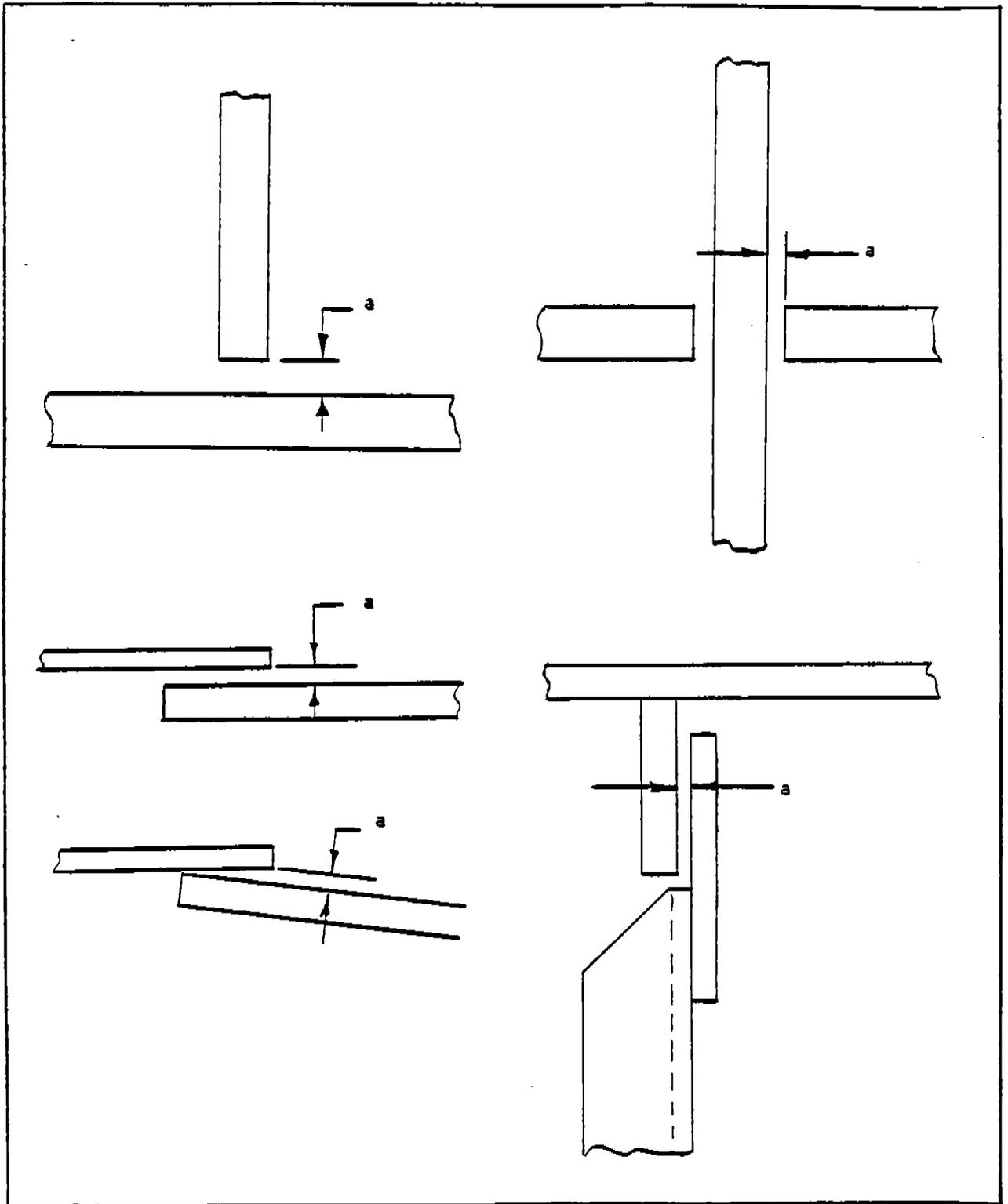
Figure 6: EXCESSIVE GAPS BETWEEN MEMBERS
