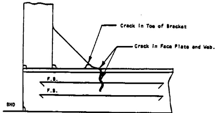
Figure 20: FRACTURE IN LONGITUDINAL INTERCOSTAL GIRDER
