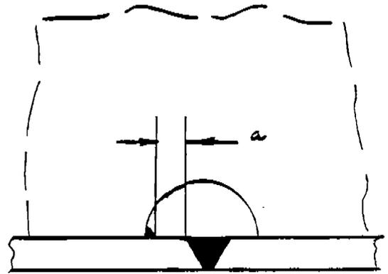
Figure 8: DISTANCE BETWEEN BUTT WELD AND SCALLOP
