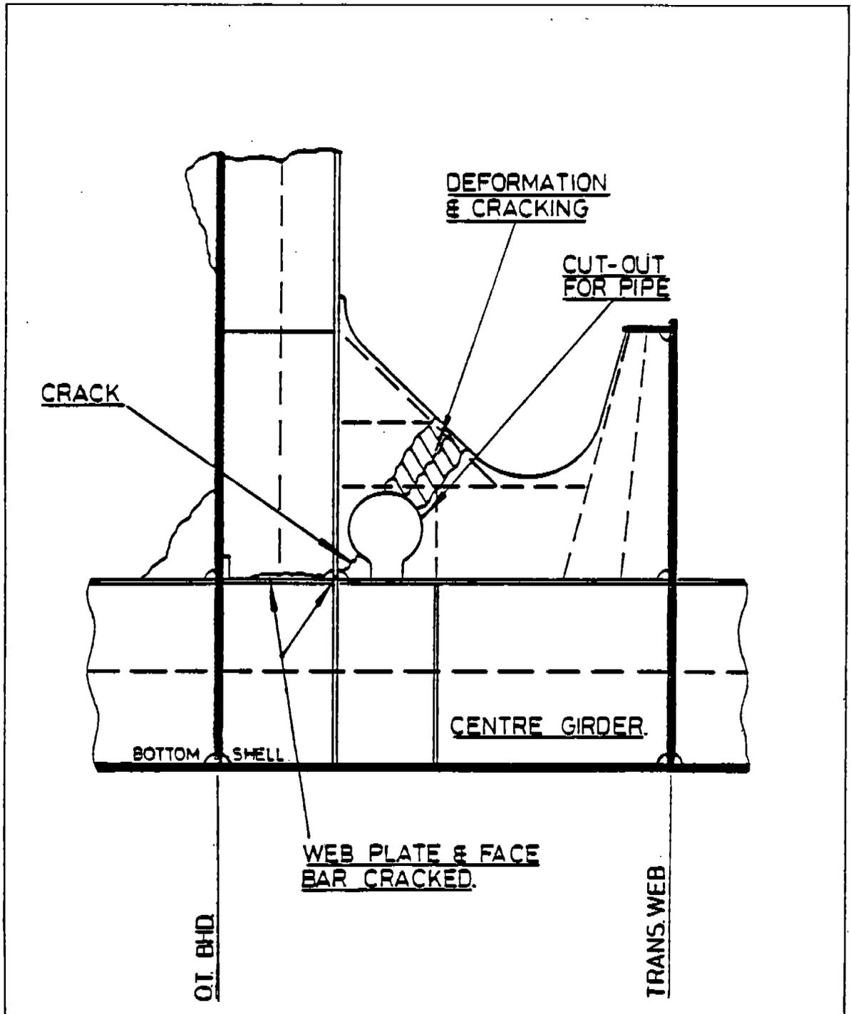
Figure 23: CENTER GIRDER CRACKING
