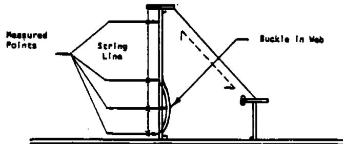
Figure 21: BUCKLING OF CENTERLINE GIRDER
