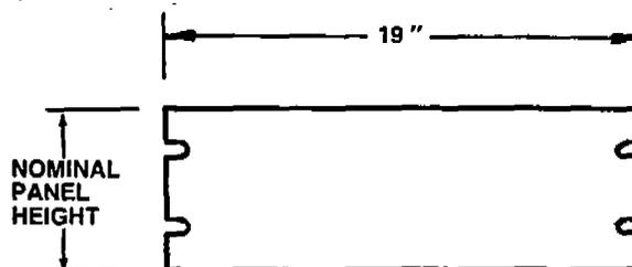
Consoliner may be used as storage, transit or permanent housing for 19" rack equipment with panel heights from 5 1/4" to 26 1/4" high. Like most TA cases, Consoliner are watertight and can be produced to conform to any applicable military specification.
