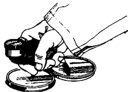
Figure 5-18 Barcol Impressor (Model 934 or 935 for readings over 75) [Cook, Polycor Polyester Gel Coats and Resins]
