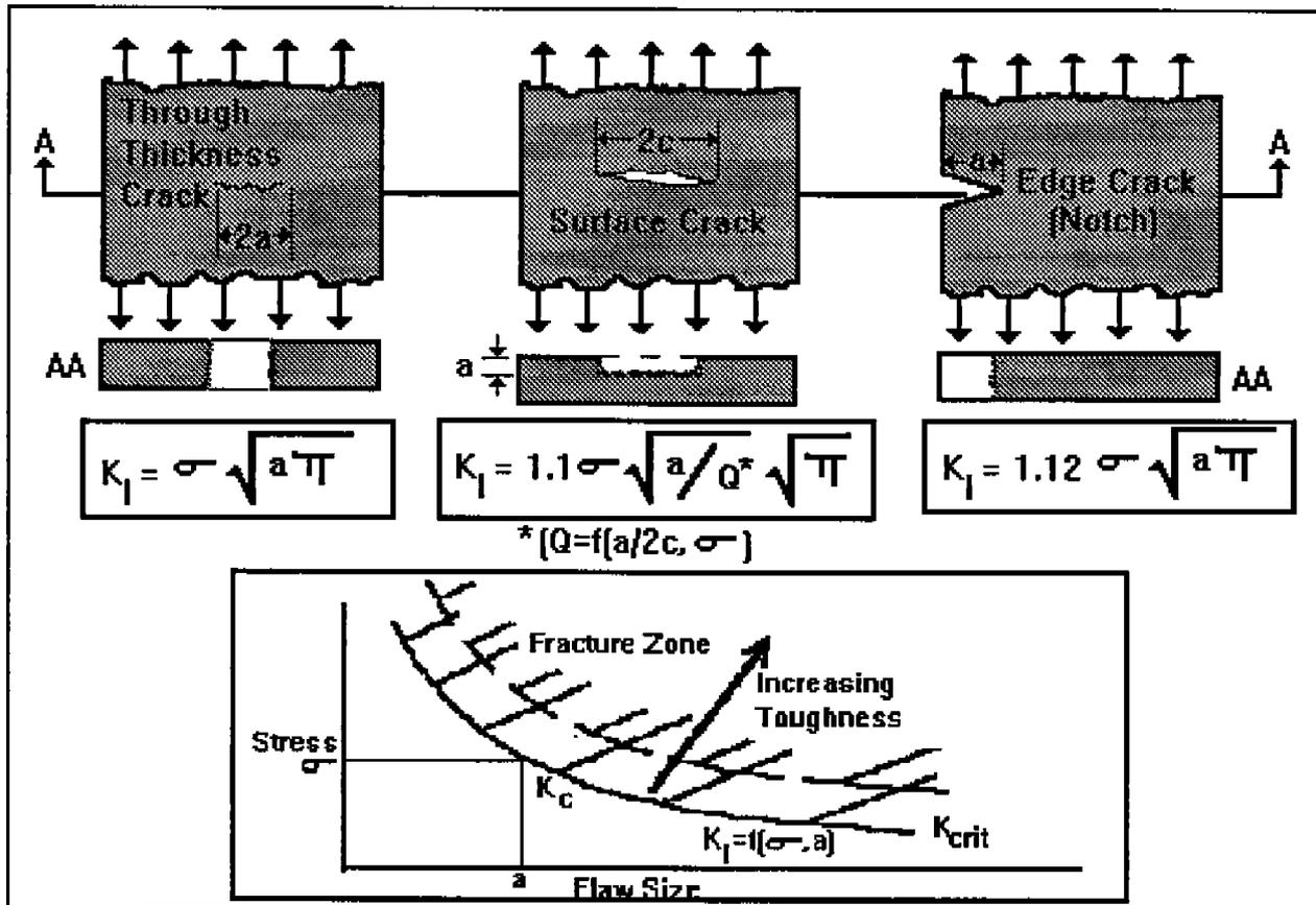
Figure 17  $K_I$  for various cracks, stress/flaw size/toughness curves.
