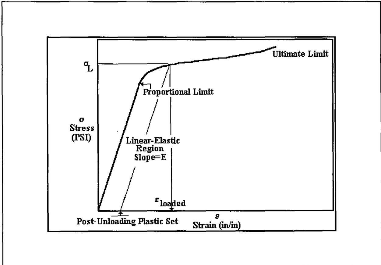
**Figure 13** Stress-Strain Curve for Metal
