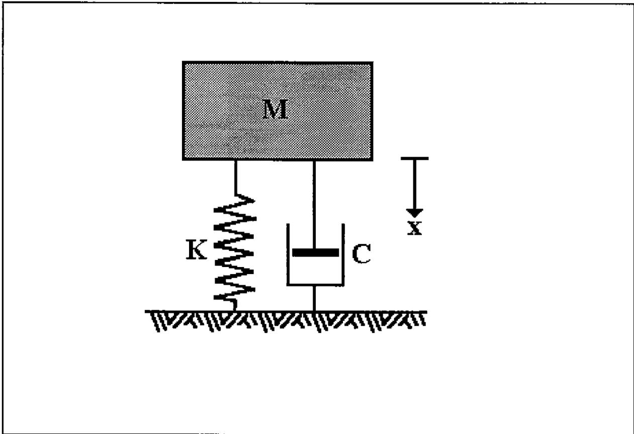
**Figure 9** Spring-Mass-Damper Model
