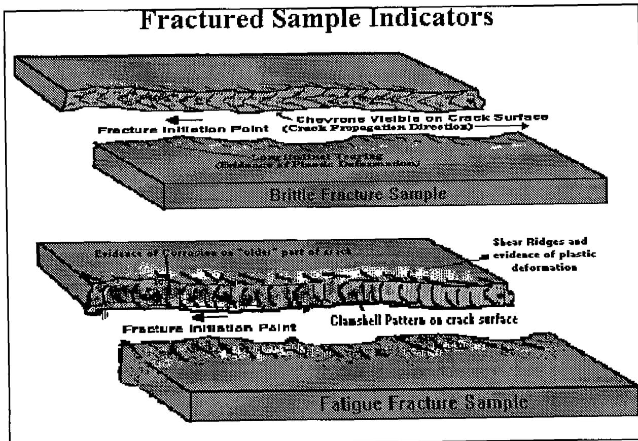
**Figure 16** Fracture Mode Identification Sketch
