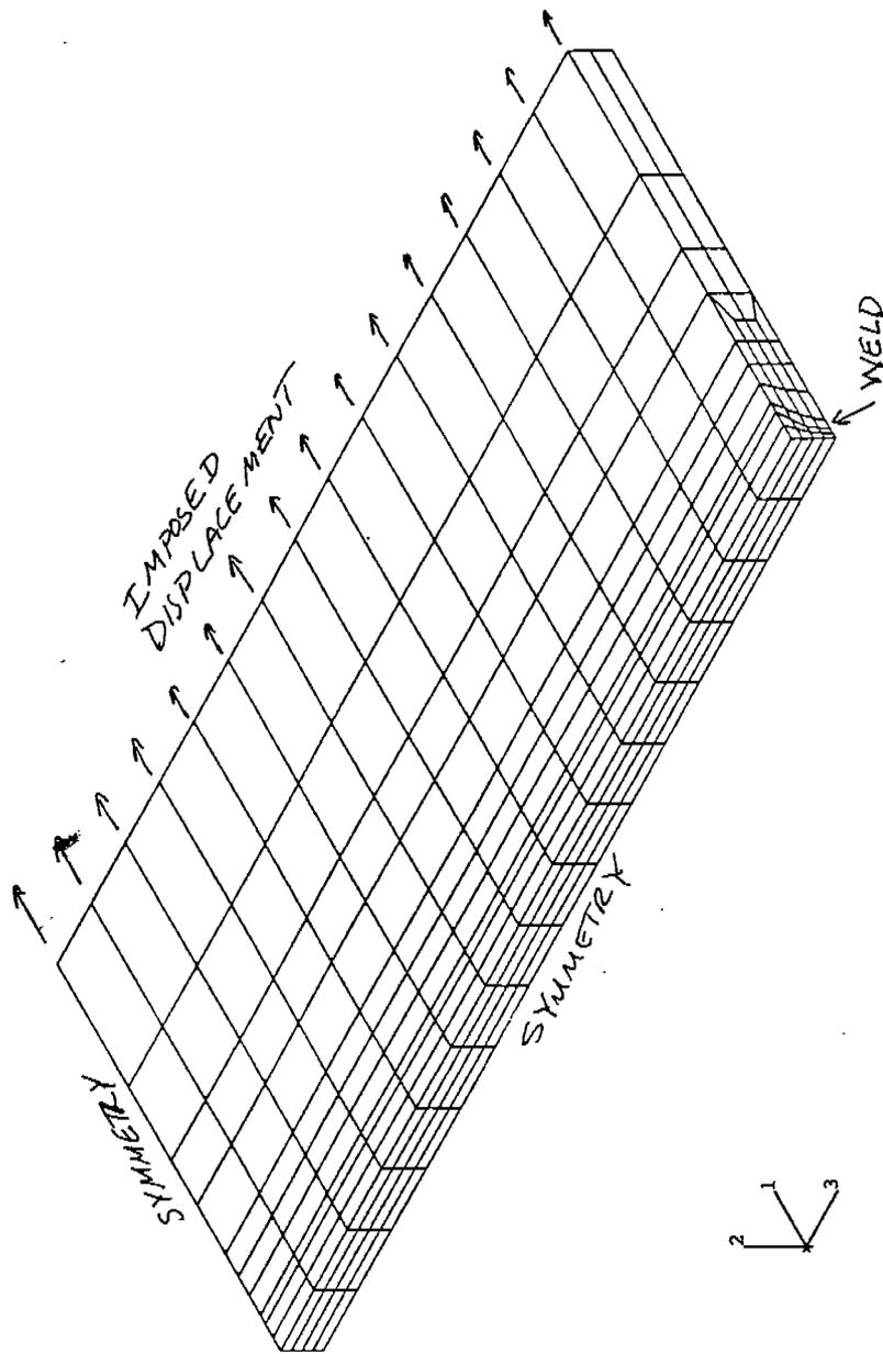
**Figure 4-1** Three-dimensional Finite Element Model of 540, 20-Node, Reduced Integration Solid Brick Elements
