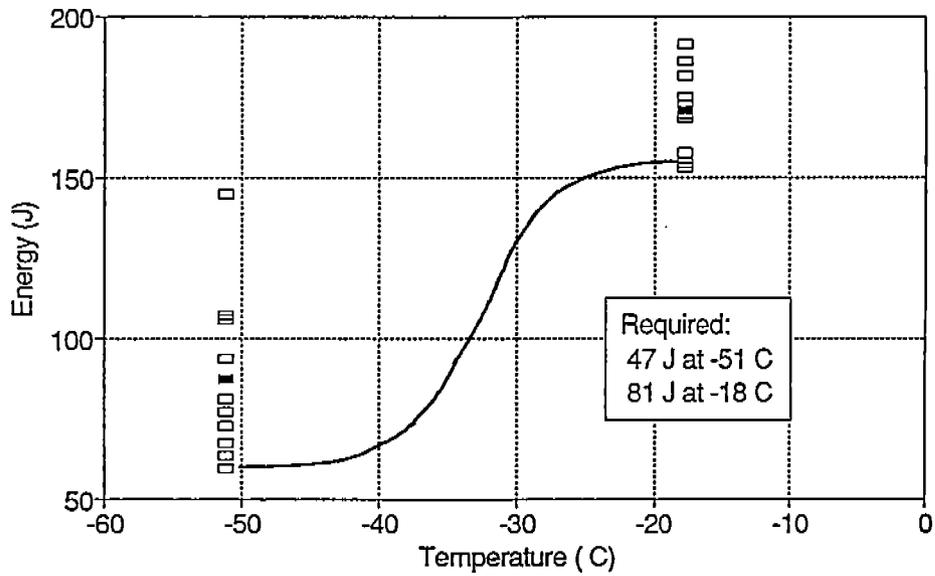
**Figure 3-2** Comparison of Charpy Toughness Data for the 120S-1 and 100S-1 Welds Showing the Better Toughness of the 100S-1 Weld Metal.
