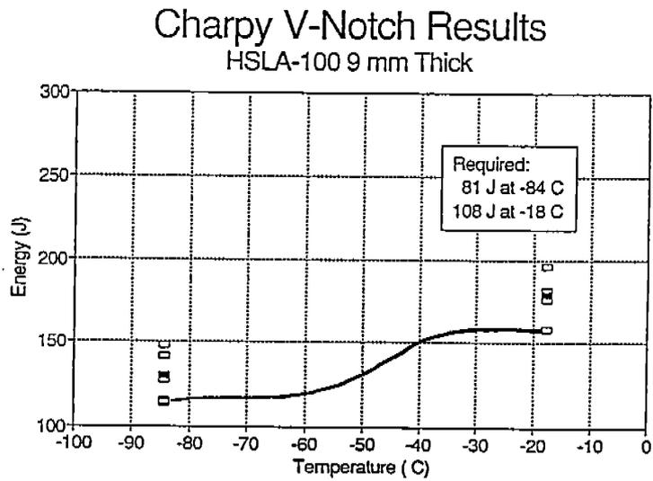
**Figure 3-1** Charpy Toughness Data for HSLA-100 Plates in First Series of Tests.
