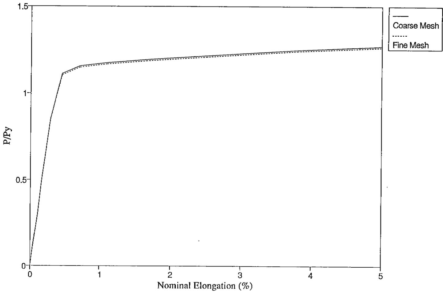
Figure 4-6 Comparison of Computed Load-Displacement Data for the Coarse and Fine Meshes Showing Good Agreement.
