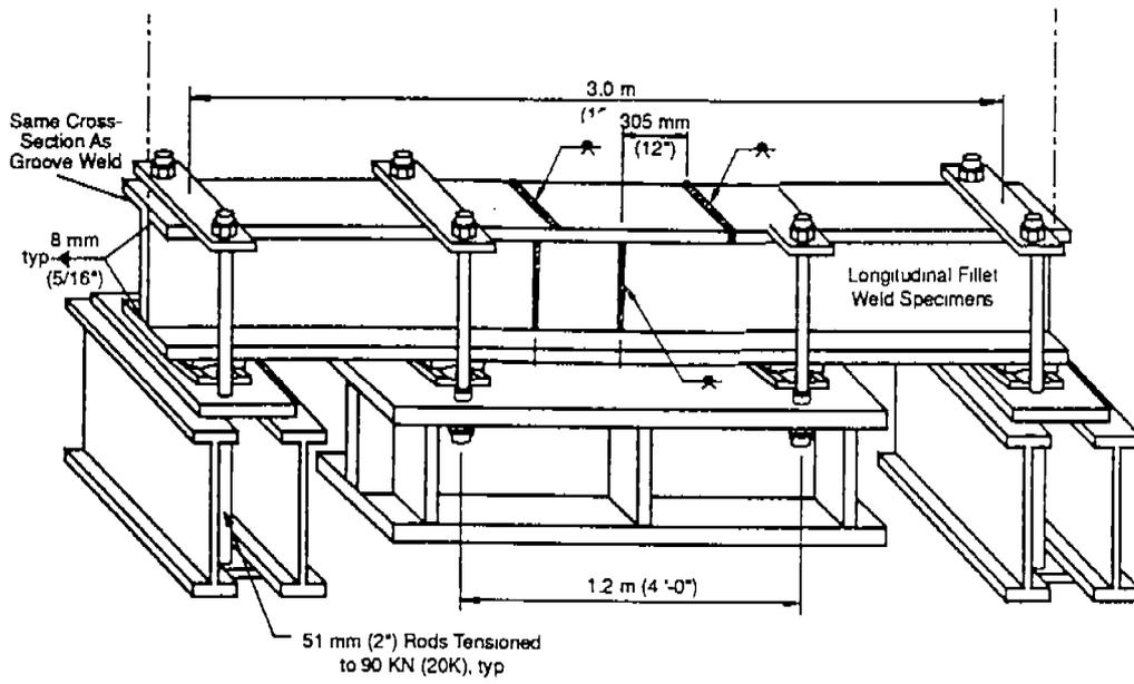
**Figure 3-4** Fatigue Specimen and Test Set-Up.
