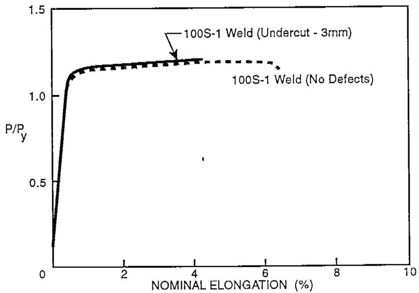
**Figure 4-15** Comparison of the Load Deformation Curves of an Undermatched Welded Joint with Simulated Undercut to an Undermatched Welded Joint Without Defects Showing the Undercut Does Not Cause a Significant Reduction of Strength or Ductility.
