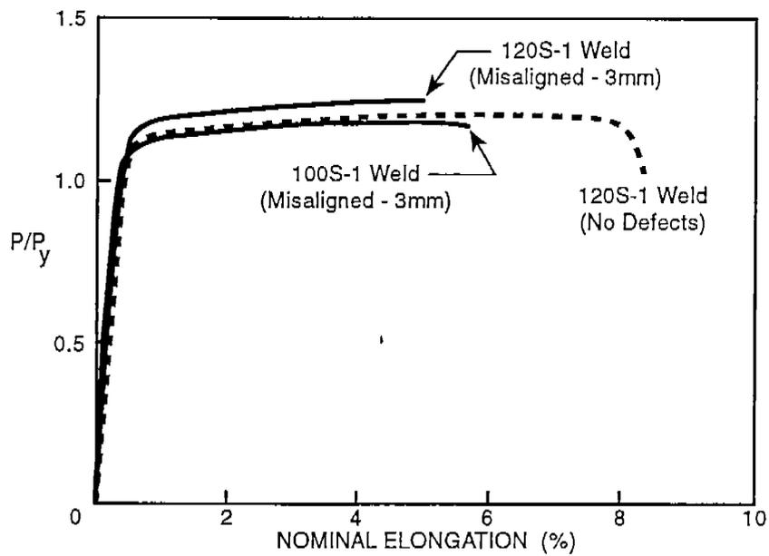
**Figure 4-13** Comparison of the Load-Deformation Behavior of Misaligned Over- and Undermatched Welded Joints with Overmatched Welded Joint Showing the Misalignment has no Effect on Strength and Only Slightly Decreases Ductility.
