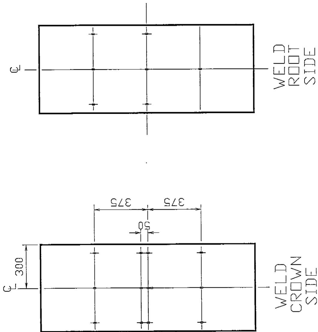
Figure 3-13 Instrumentation Plan for Tension Specimens.
