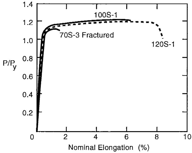
**Figure 3-17** Normalized Load Displacement Curves for Three Different Weld Metal Specimens.
