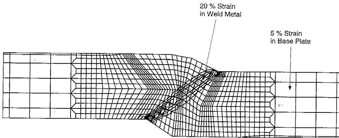
**Figure 4-12** Weld Macrosection and Strain Contours from a Generalized Plane-Strain Finite Element Analysis of a Misaligned Welded Joint.
