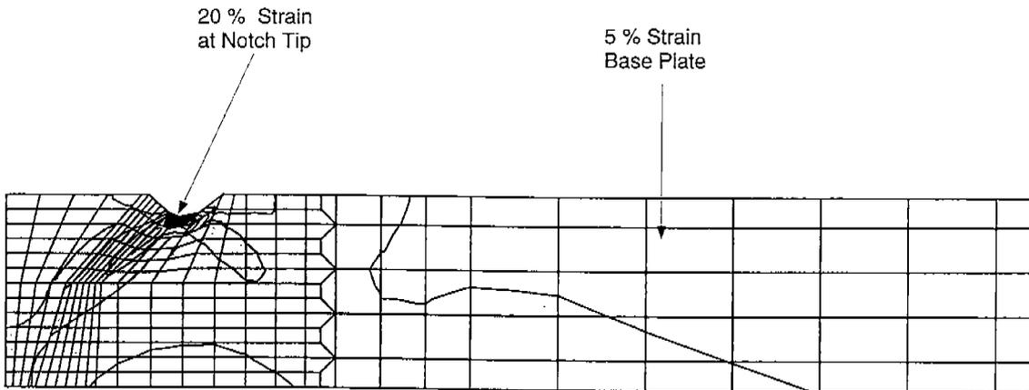
**Figure 4-14** Weld Macrosection and Finite-Element Strain Contours for a Welded Joint with Simulated Undercut.
