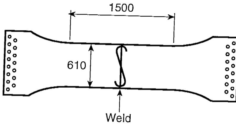
**Figure 3-12** Tension Specimen Design.
