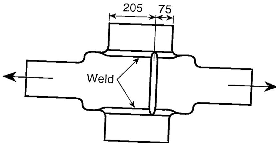
Figure 3-6 Shear Specimen Design.
