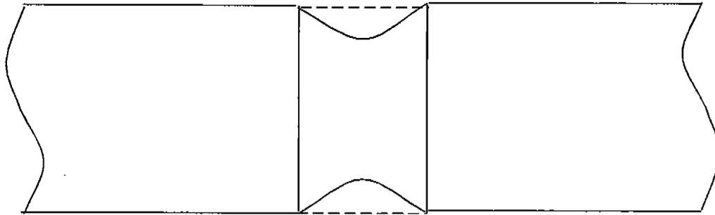
**Figure 2-2** Weld Deformations that Lead to the Development of Constraint.
