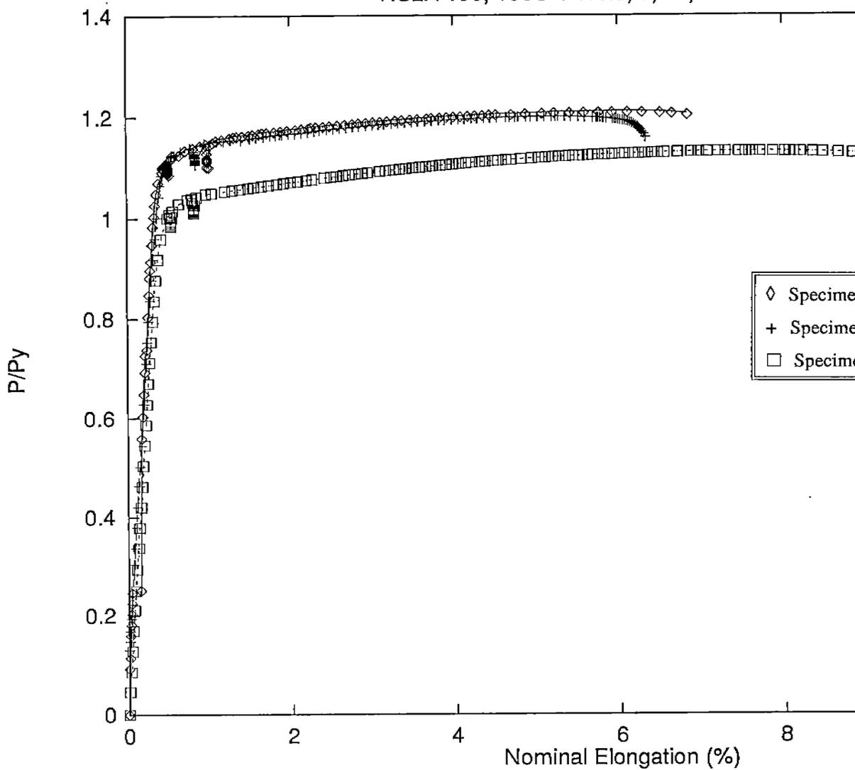
Figure 3-16 Normalized Load Displacement Curves for Three Different Thicknesses of the 100S-1 Weld Metal.
