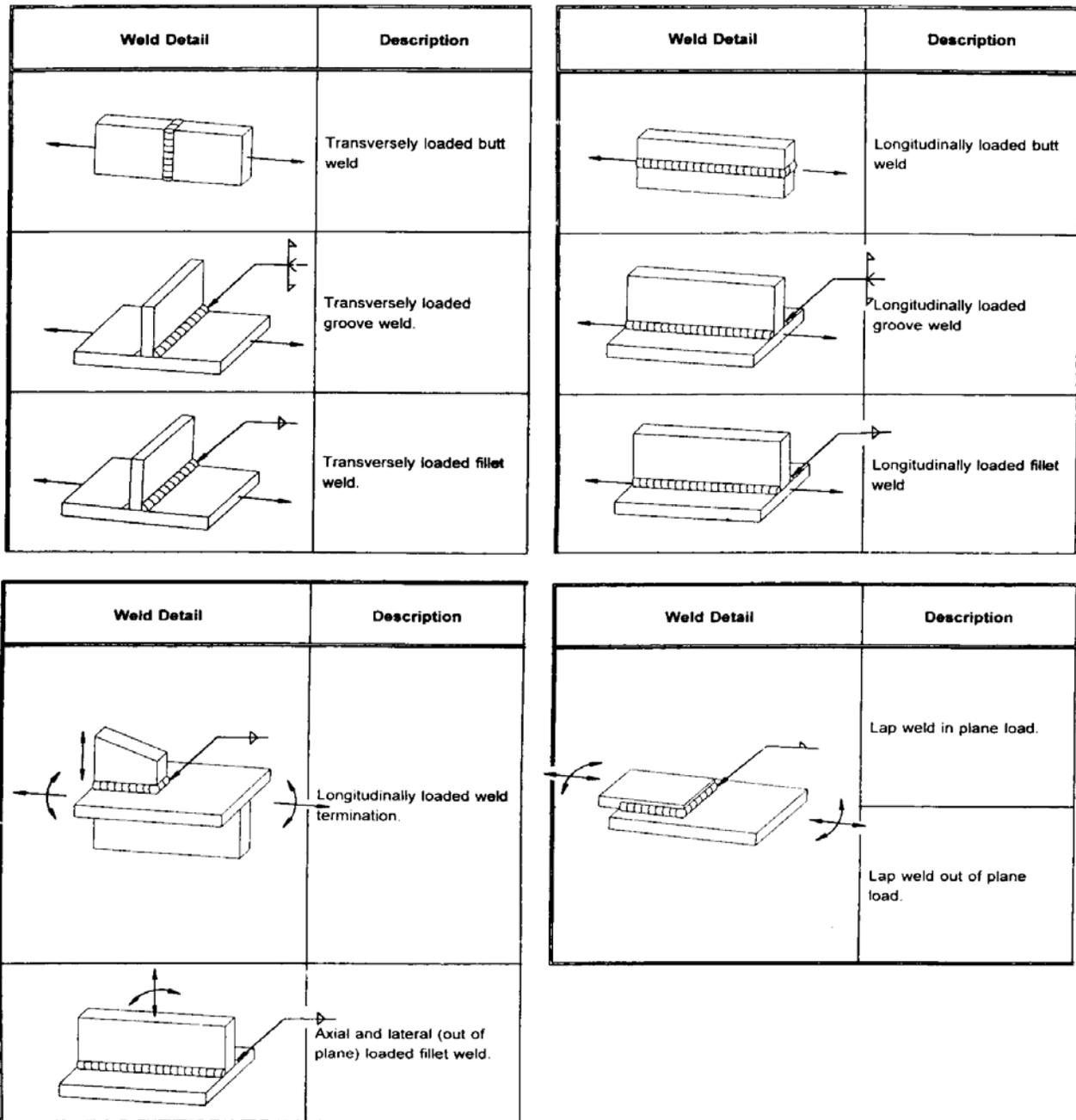
Figure 4.2 Basic Weld Details (Stambaugh et. al., 1994)
