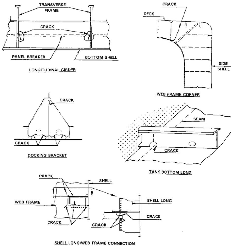
**Figure 2.2 Typical TAPS Tanker Cracking Problems (Heyburn and Riker, 1994)**
