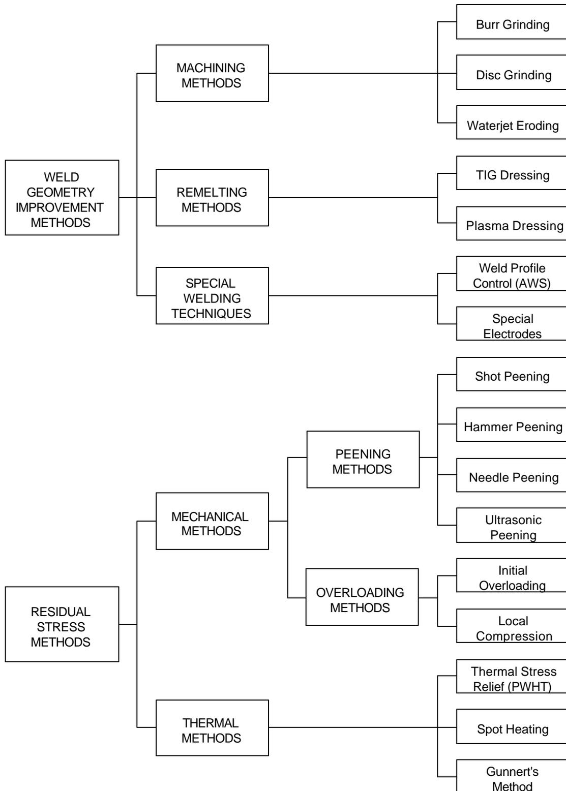
**Figure 3.1 Classification of Some Weld Improvement Methods**
