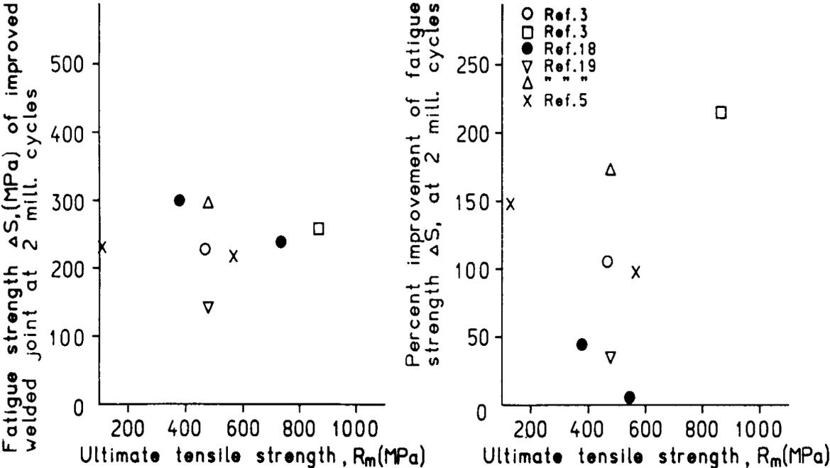
**Figure 3.18 Variation in Fatigue Strength Improvement Due to Hammer Peening as a Function as a Base Material Strength (Haagensen, 1985)**
