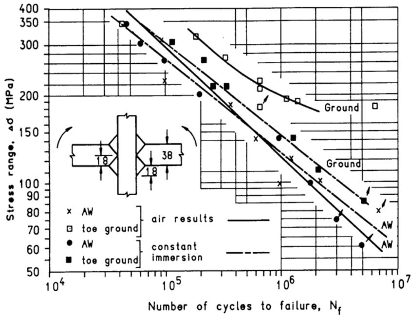
Figure 3.29 The Effect of Free Corrosion in Seawater on the Fatigue Strength of As-Welded and Ground Specimens (Booth, 1978)
