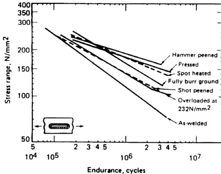
Figure 3.33 Effect of Improvement Techniques Applied to Mild Steel Fillet Welded Longitudinal Non-Load-Carrying Joints (Booth, 1991)
