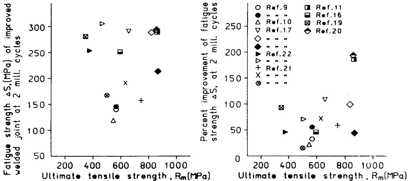
Figure 3.9 Variation in Fatigue Strength Improvement Due to TIG Dressing as a Function of Base Material Strength (Haagensen, 1985)
