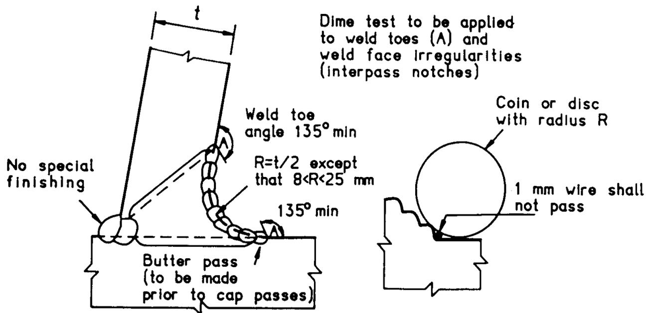
Figure 3.11 The AWS Improved Profile Weld and the "Dime Test" (AWS, 1996)
