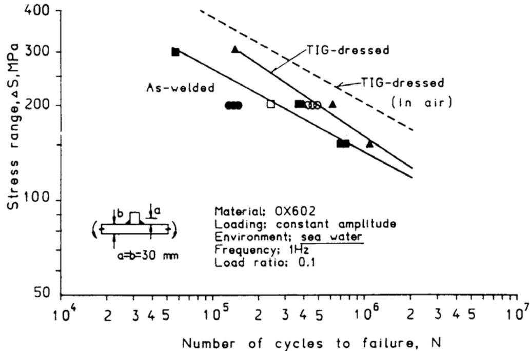
**Figure 4.10 Influence of Seawater Corrosion on the Fatigue Strength of As-Welded and TIG**
