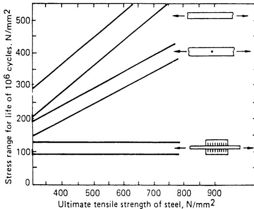
**Figure 2.4 Effect of Tensile Strength on Fatigue Strength of Steel (Maddox, 1983)**
