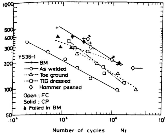
**Figure 4.5 Effect of Weld Toe Treatment on the Fatigue Strength of a 272 MPa Yield Strength Steel in Artificial Seawater (Matsumoto et al., 1989)**
