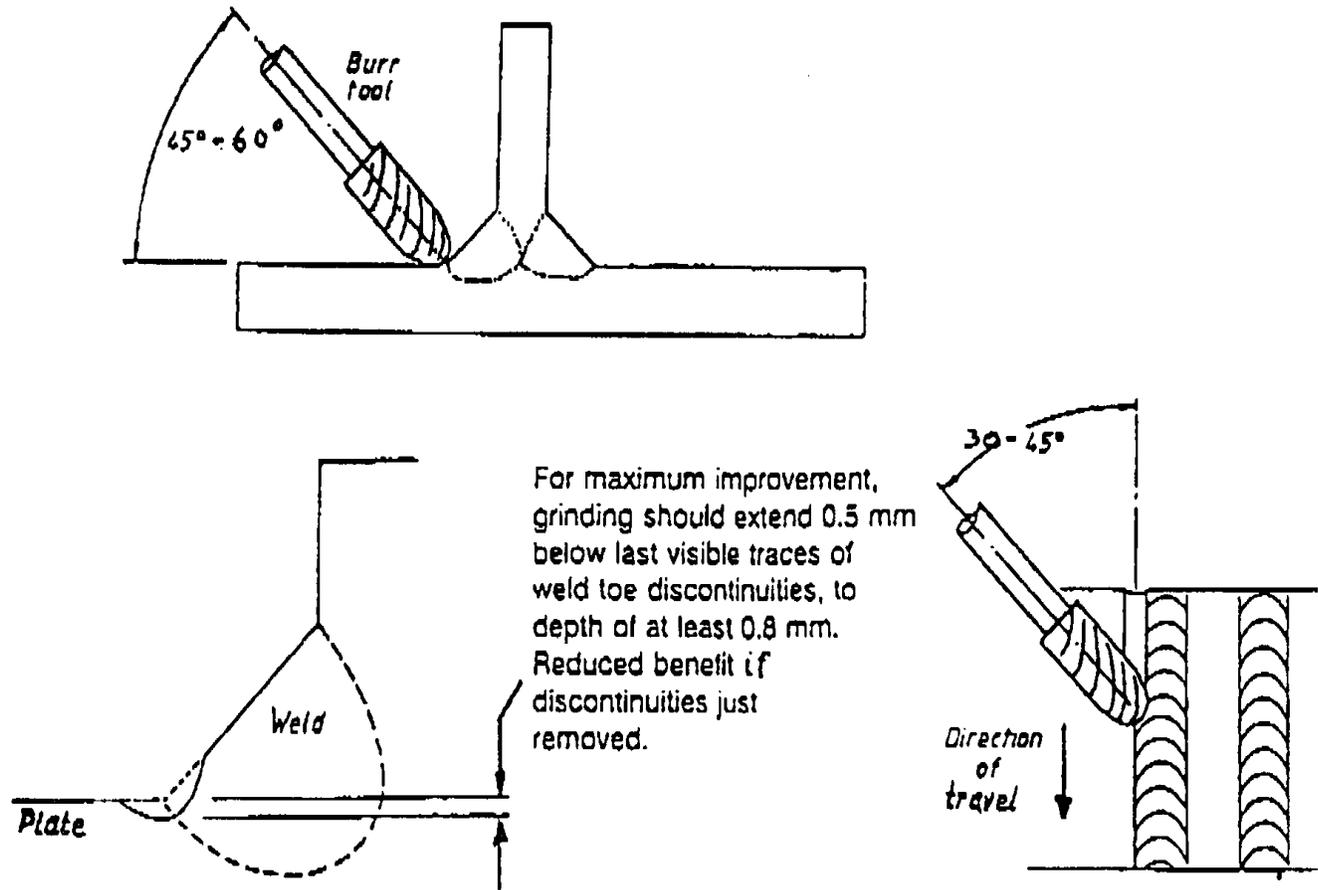
**Figure 3.3 Weld Toe Burr Grinding Technique (Haagensen and Maddox, 1995)**
