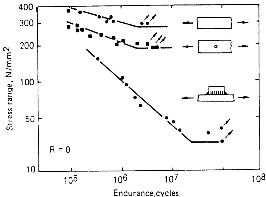
**Figure 2.3 Comparison Between Fatigue Strengths of Plain Steel Plate, Notched Plate, and Plate with Fillet Welded Attachment (Maddox, 1983)**
