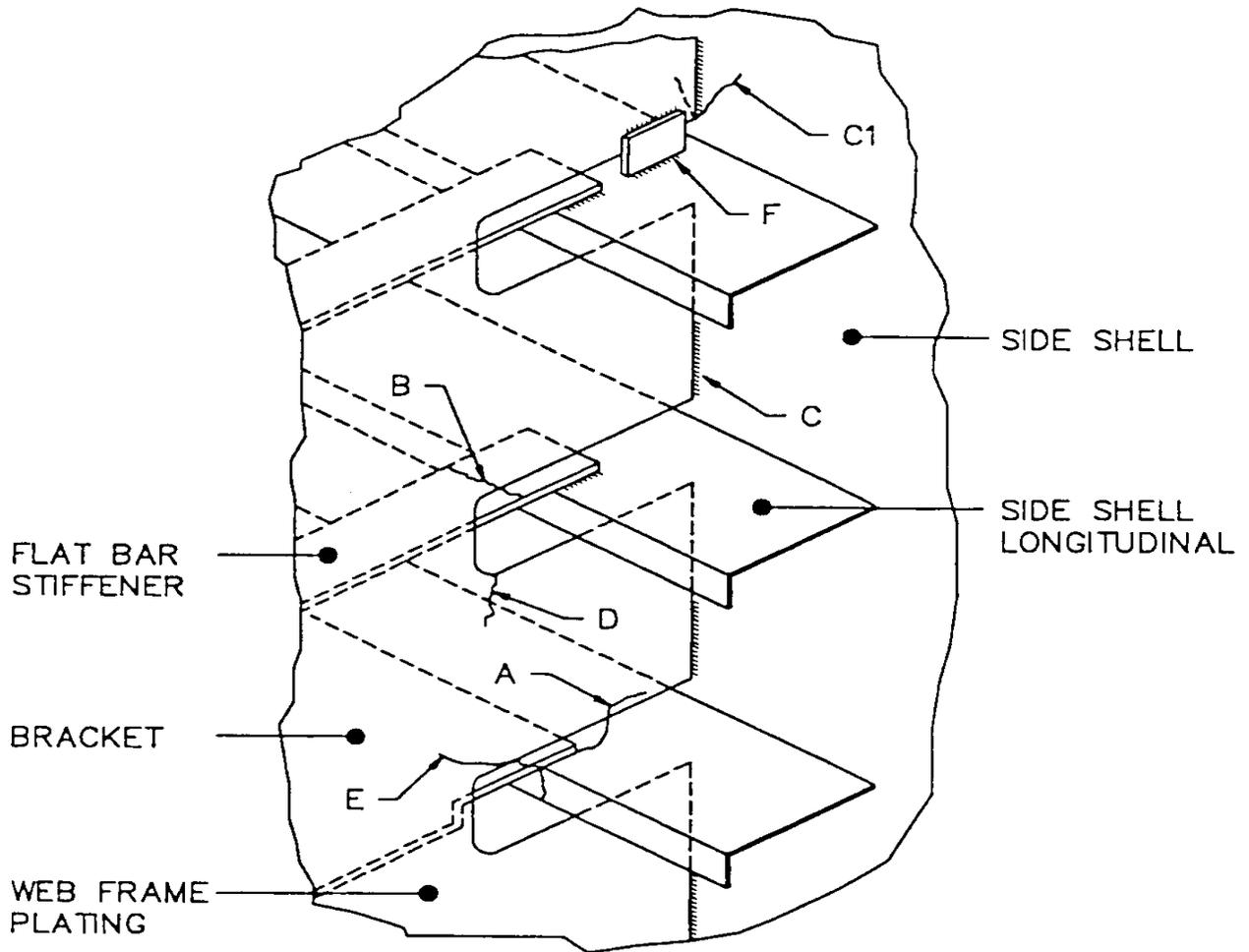
TYPICAL SIDE SHELL STRUCTURAL DEFECTS
