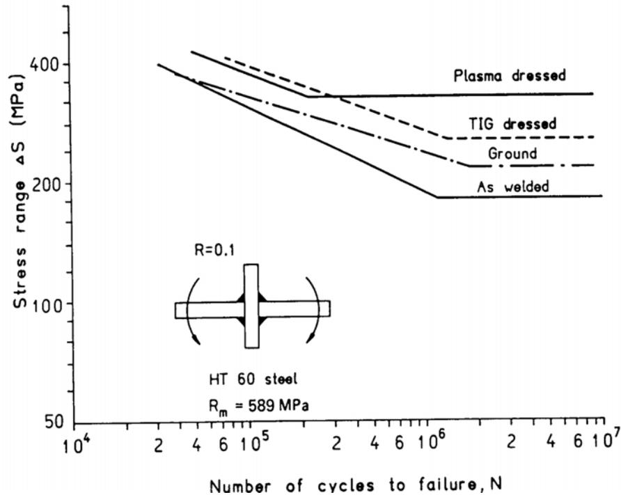
Figure 3.31 Effect of Some Improvement Methods Applied to High-Strength Steels (Shimada et al., 1977)
