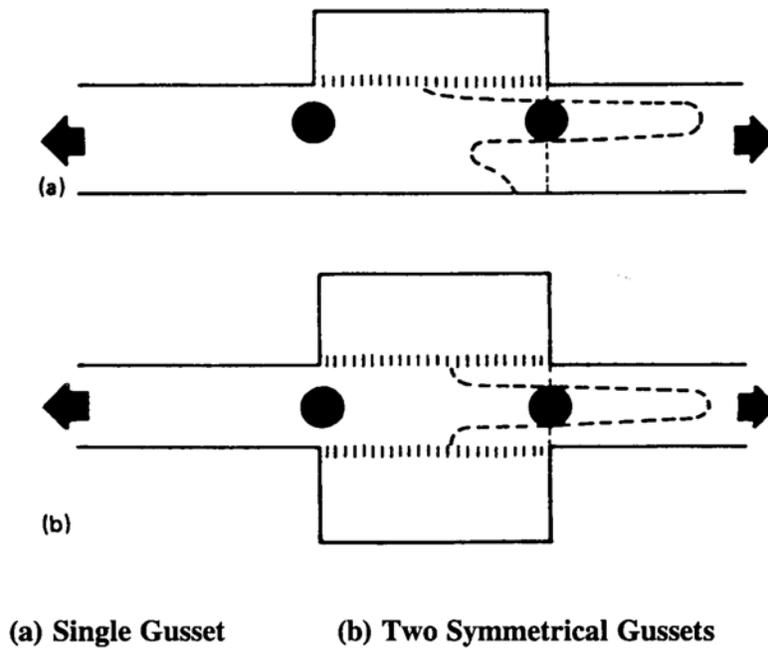
Figure 3.22 Suggested Positions for Heated Spot in Specimens with Discontinuous Longitudinal Welds (Booth, 1991)
