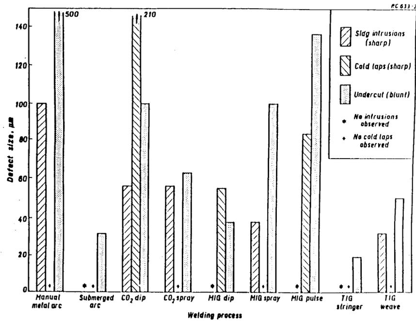
Figure 2.6 Weld Defect Sizes for Different Welding Processes (Gordon, 1993)
