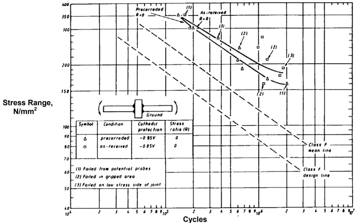
Figure 4.3 Fatigue Tests for Ground Joints (Booth, 1987)
