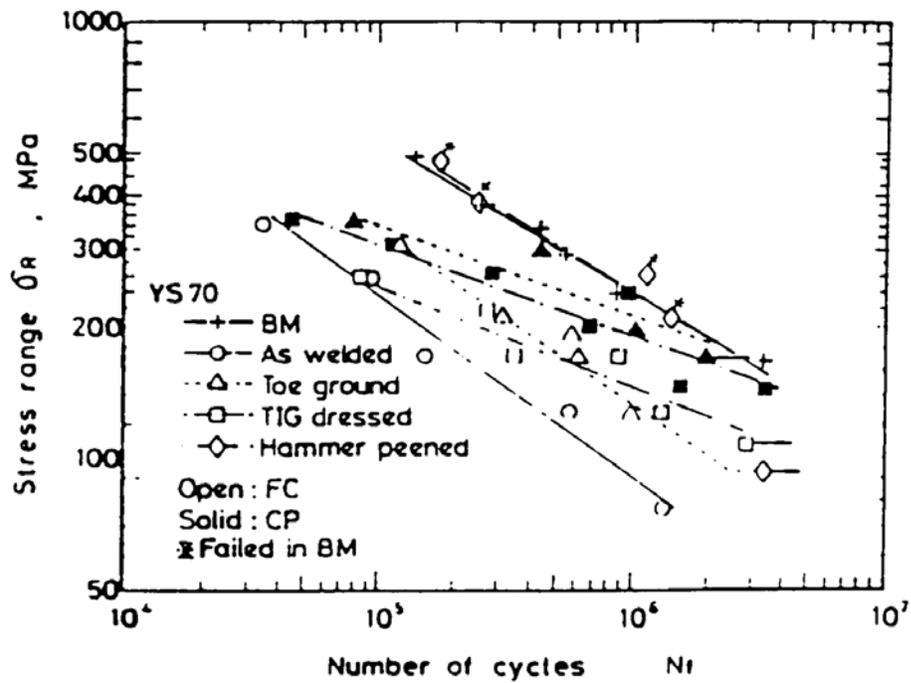
**Figure 4.8 Effect of Weld Toe Treatment on the Fatigue Strength of a 764 MPa Yield Strength**
