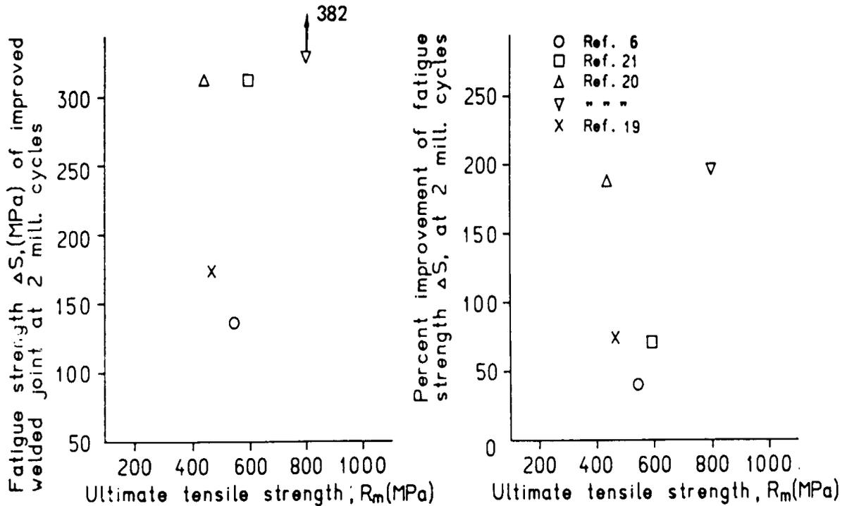
**Figure 3.10 Variation in Fatigue Strength Improvement Due to Plasma Dressing as a Function of Base Material Strength (Haagensen, 1985)**
