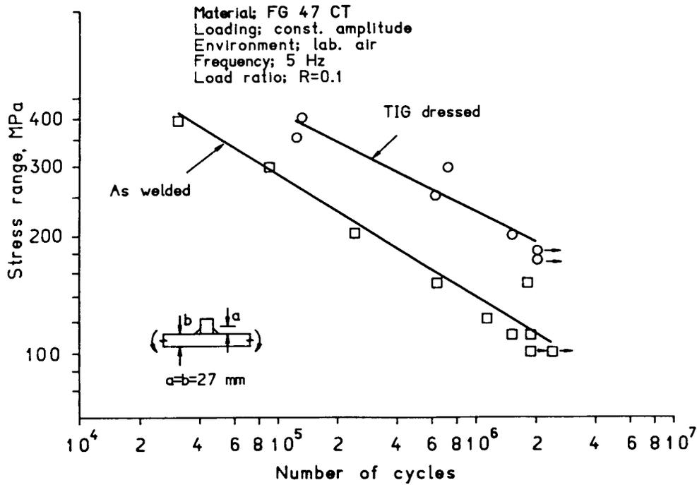
Figure 3.8 Effect of TIG Dressing on the Fatigue Strength of a Medium Strength Steel
