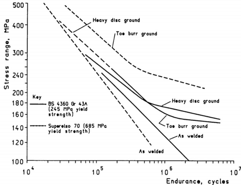
Figure 3.28 Fatigue Strength Improvements Due to Toe Burr and Disc Grinding (Knight, 1978)
