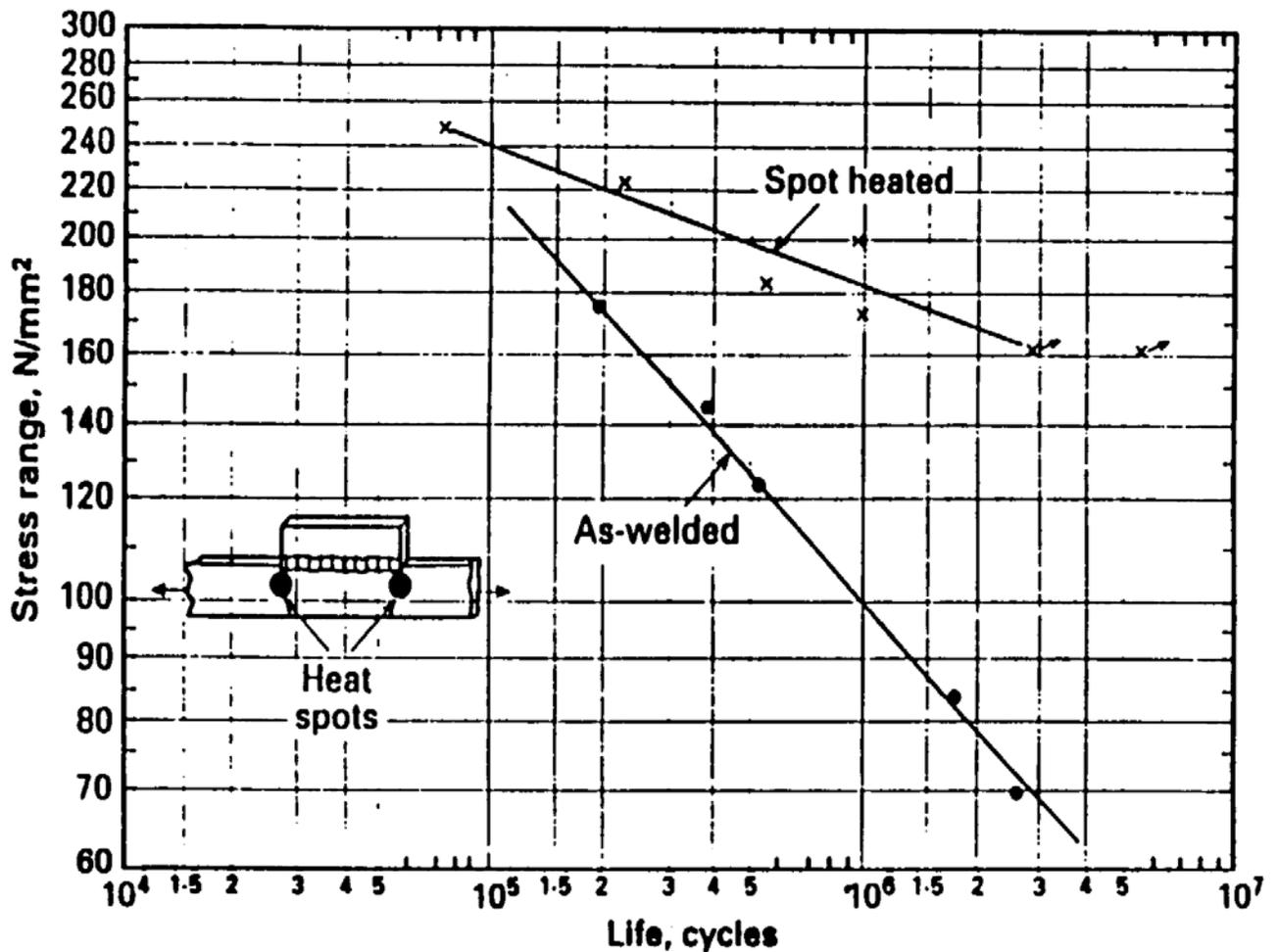
Figure 3.23 Effect of Spot Heating on Fatigue Strength of Plate with Edge Attachment (Gordon, 1993)
