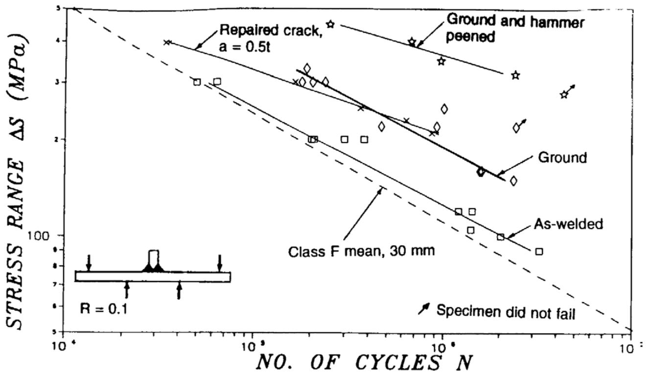
Figure 3.35 Comparison of S-N Curves for As-Welded, Toe Ground, Repaired and Ground and Hammer Peened Specimens (Haagensen, 1993)
