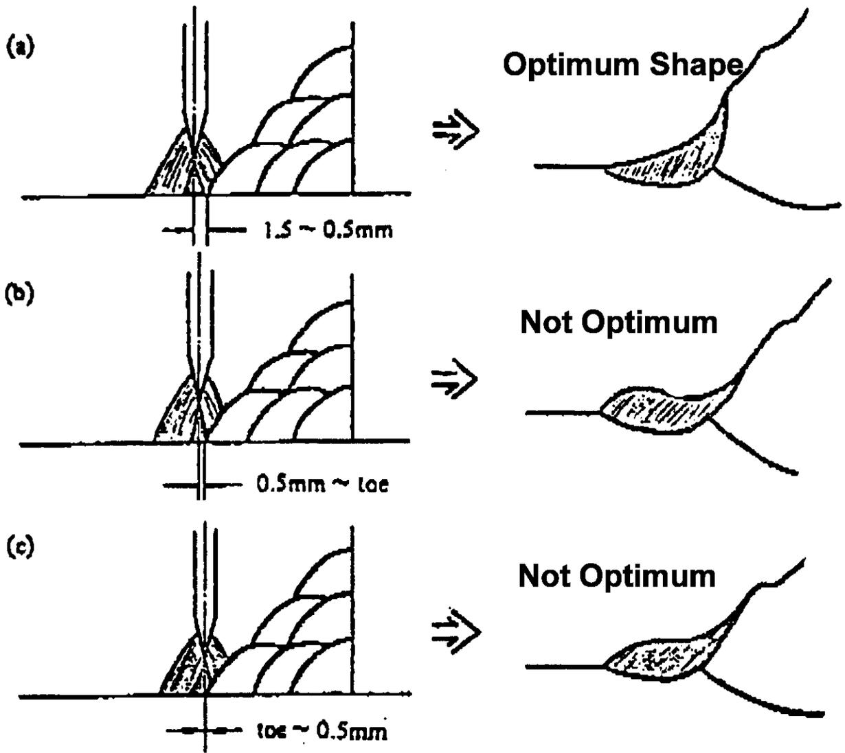
(b) and (c) are too close to toe resulting in non-optimal shape
