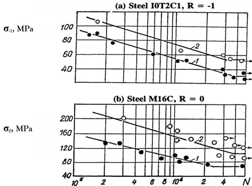
Figure 3.25 Improvements in Fatigue Strength of Welded Joints with Transverse Stiffeners Using the Explosive Treatment (Petushkov, 1993)
