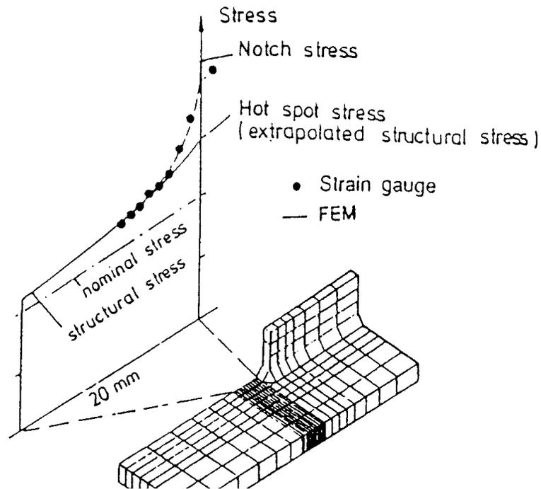
**Figure 2.7 Stresses Near the Weld Toe (Maddox, 1993)**
