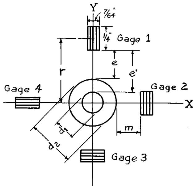
Fig. 1. Gage Location for Calibration Tests
