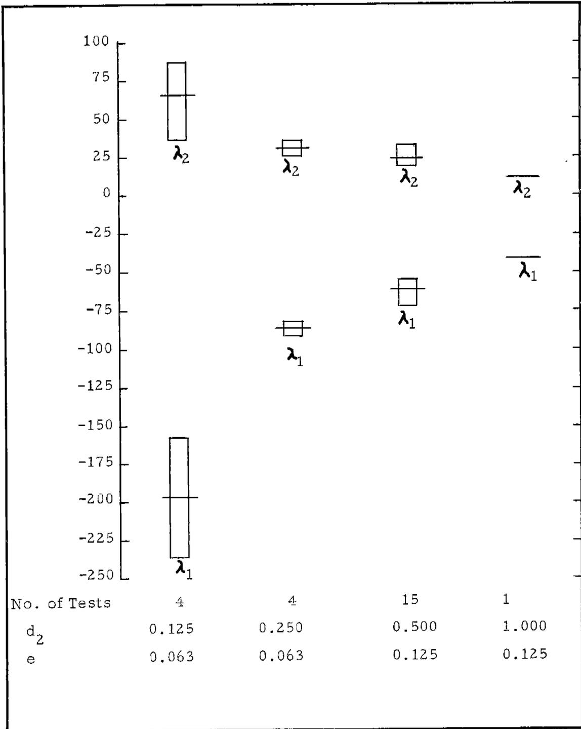
Fig. 4.  $\lambda_1$  and  $\lambda_2$  values for various hole diameters in Arrangement I from no hole to a final twist drilled hole. All tests were performed in tension on an approximately equal number of 3/8-in. thick and 3/4-in. thick specimens. The length of bar indicates the range of values and the horizontal line in each bar represents the average value for the indicated number of tests.
