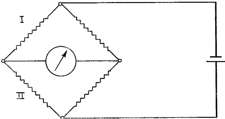
Fig. A-8. Connection of Gages in Measuring Bridge for Arrangement III
