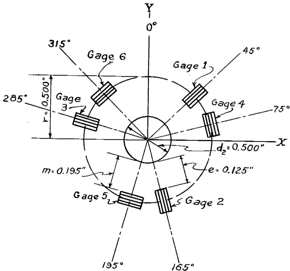
Fig. 5. Gage arrangement field type on stress-relieved plate (Test 37)
