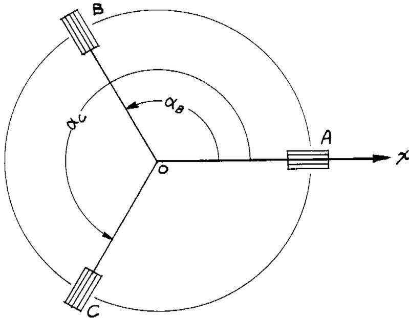
Fig. A-2. Placement of Gages for Measuring Strain in the Radial Direction for Arrangement I
