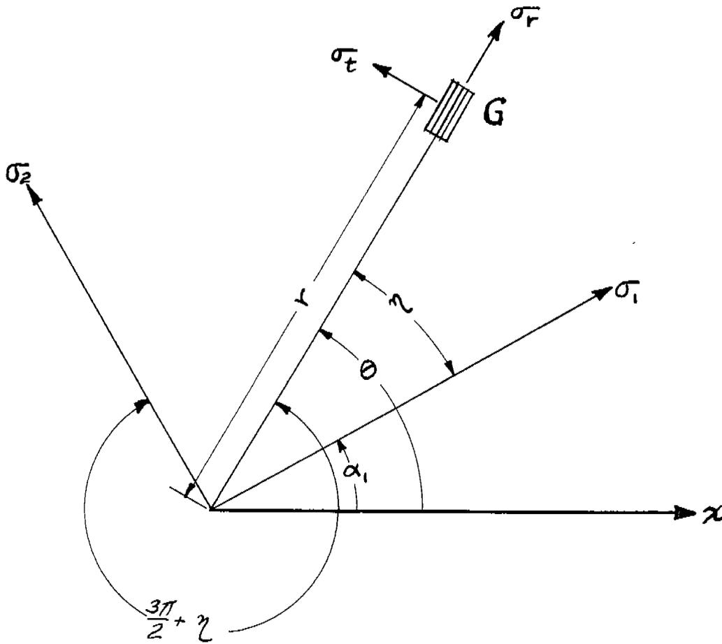
Fig. A-3. Description of Terms as Used in Arrangement I
