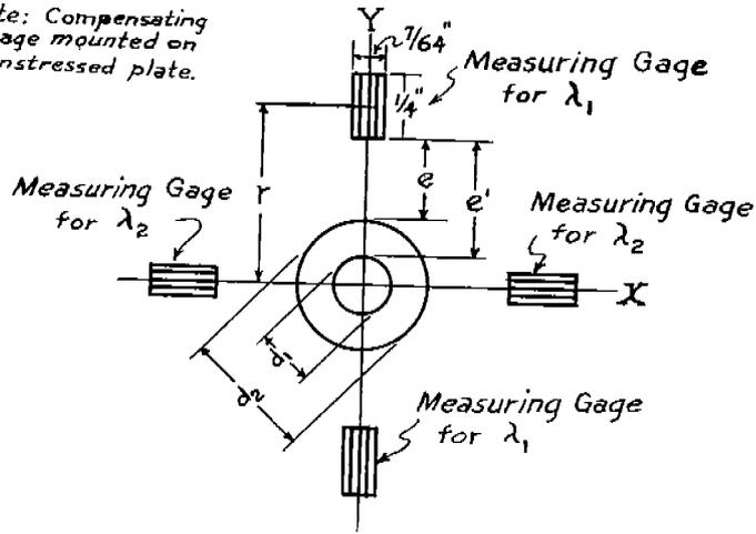
Fig. 2 . Double Arrangement I of Gages to Obtain an Average  $\lambda$  Value
