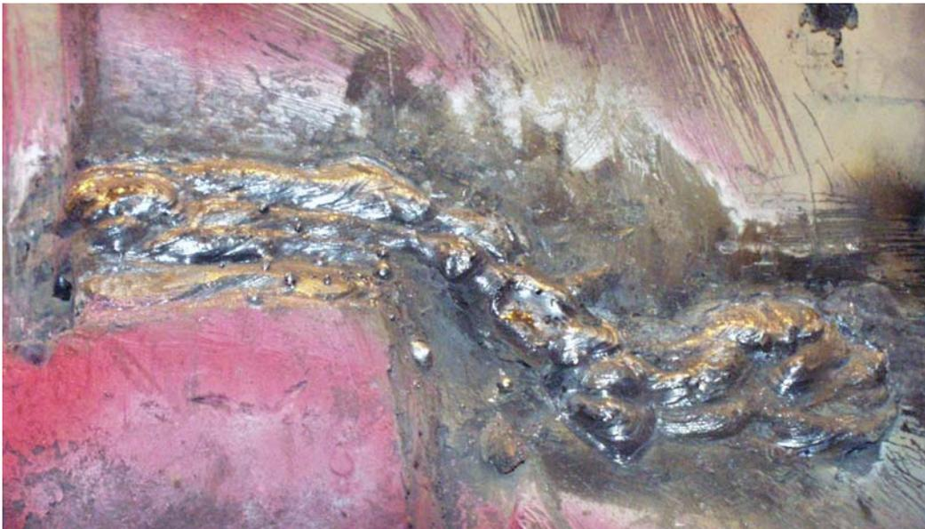
Figure 14: Weld repair of crack not yet through-thickness without termination holes.
