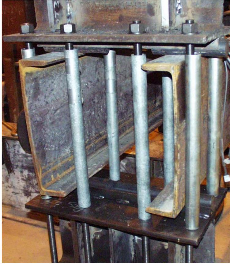
Figure 3.25: Clamped-roller support connection.
