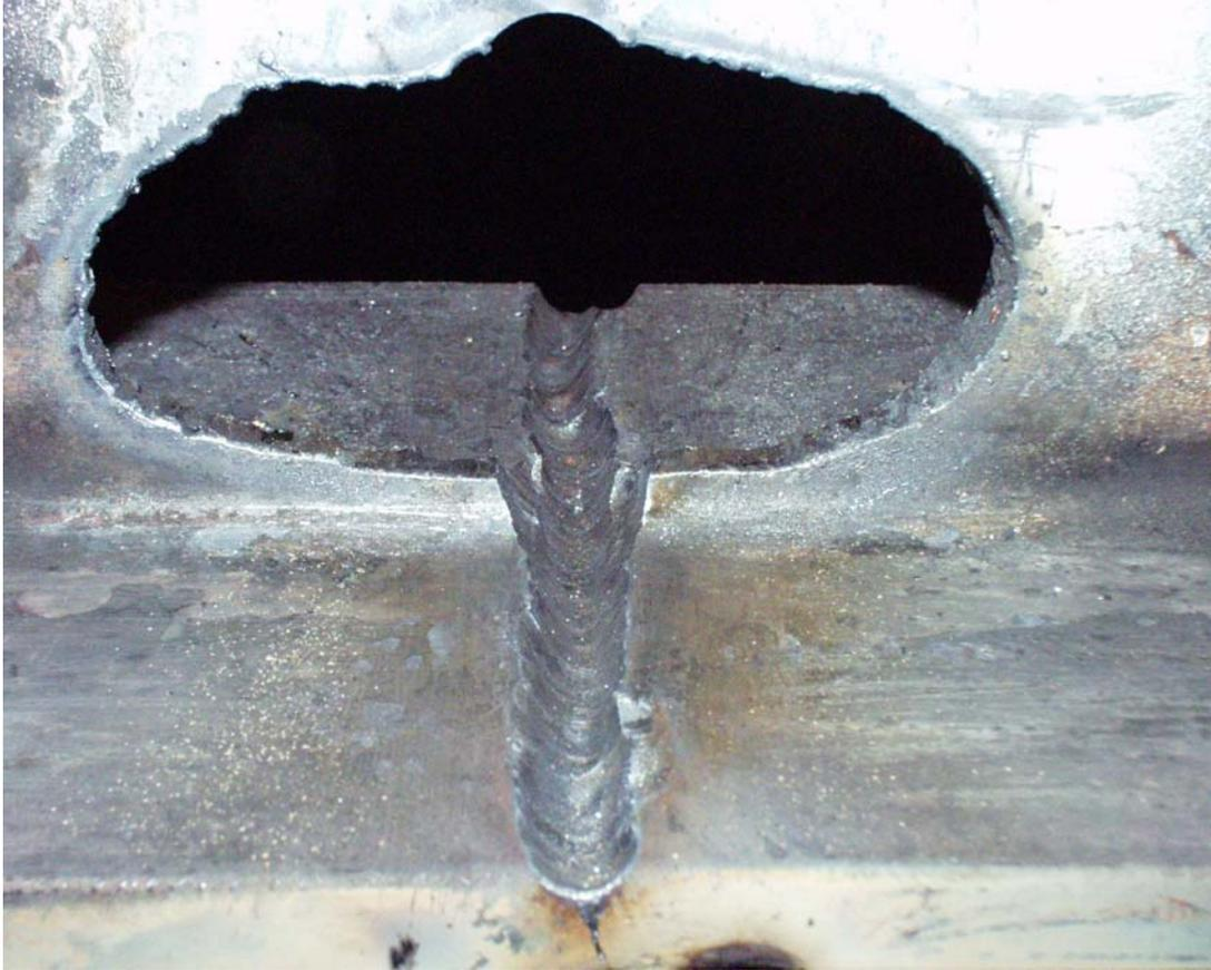
Figure 13: Gouge and access hole at attachment detail
