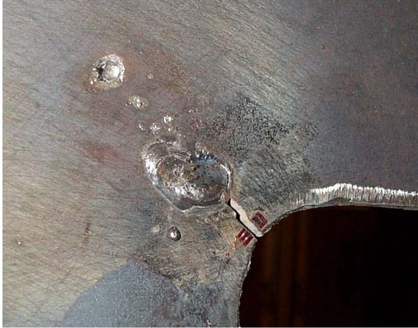
Figure 3.47 Typical saw cut and tack weld used to initiate cracks at cutouts
