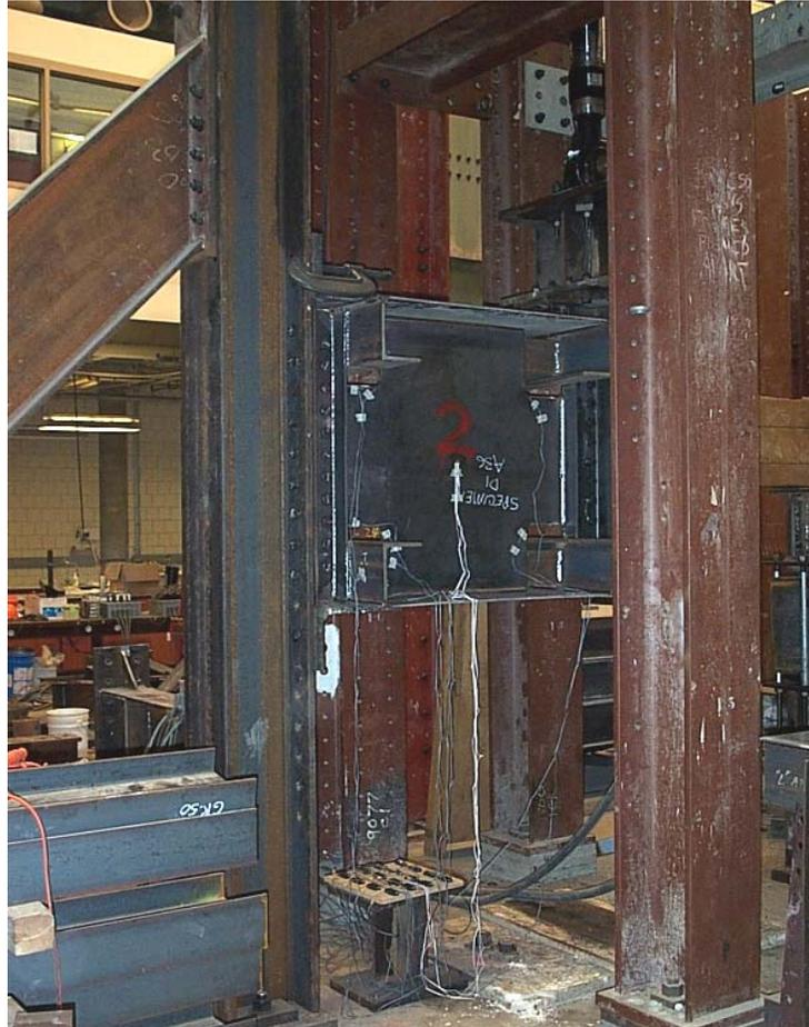
Figure 3.42 Photo of simplified web frame specimen in test fixture
