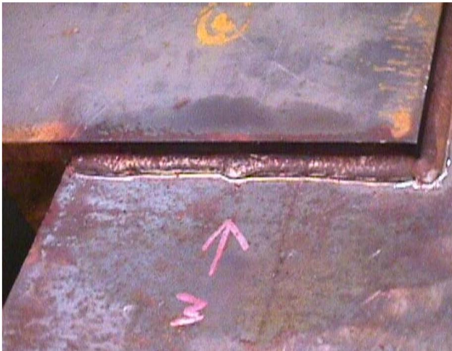
Figure 20: Hammer peened toe of a fillet weld
