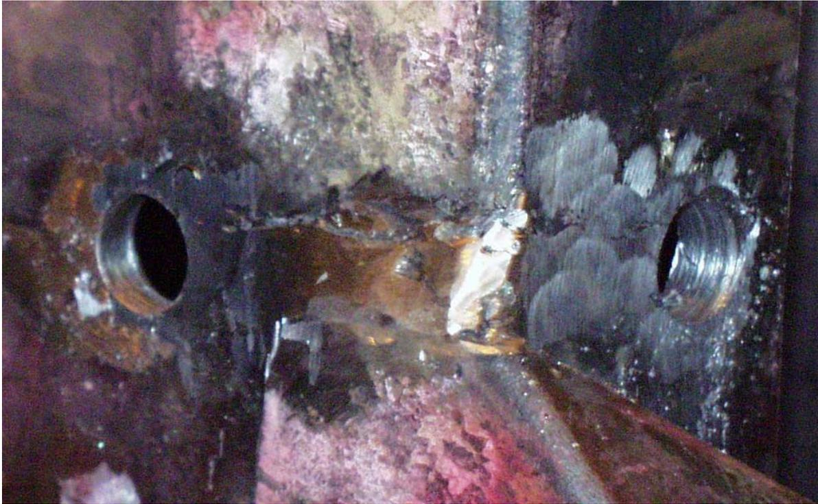
Figure 3.33: Weld ground after repair.
