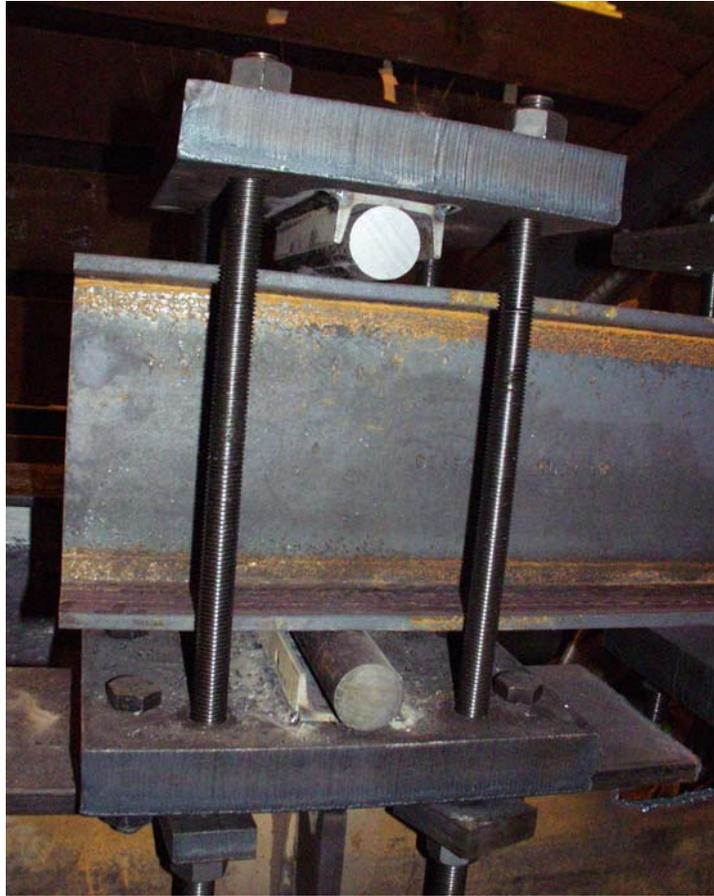
Figure 3.5: Clamped-roller connection.
