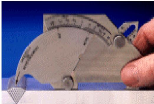
**Figure 4.2: Tool for Measuring Weld Reinforcement Height and/or Plate Alignment and Fillet Weld Leg Size**
