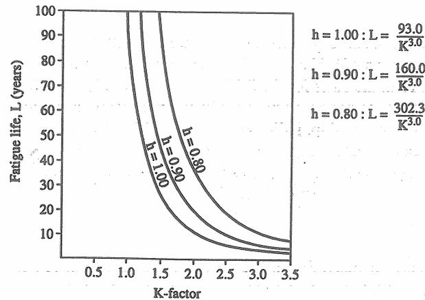
**Figure 3.14: Fatigue Life Sensitivity to Stress Concentration Factor K and Weibull Shape Factor H**
