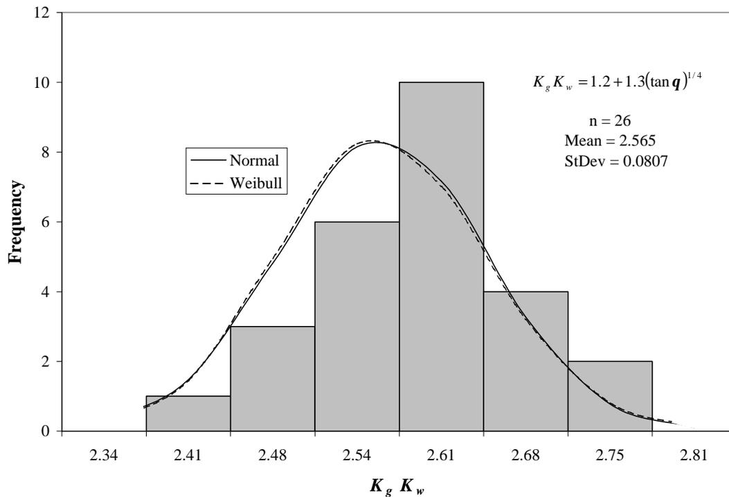
**Figure 5.10: Histogram of  $K_g K_w$  with Normal and Weibull (smallest) Distribution Fits for Fillet Weld**
