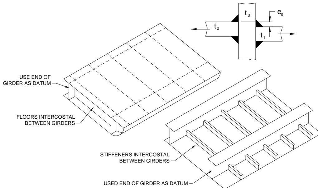
**Figure 4.6: Measuring Misalignment in Cruciform Joints**
