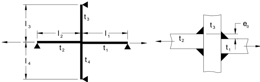
**Figure 3.7: Cruciform Joint Misalignment – Variables**
