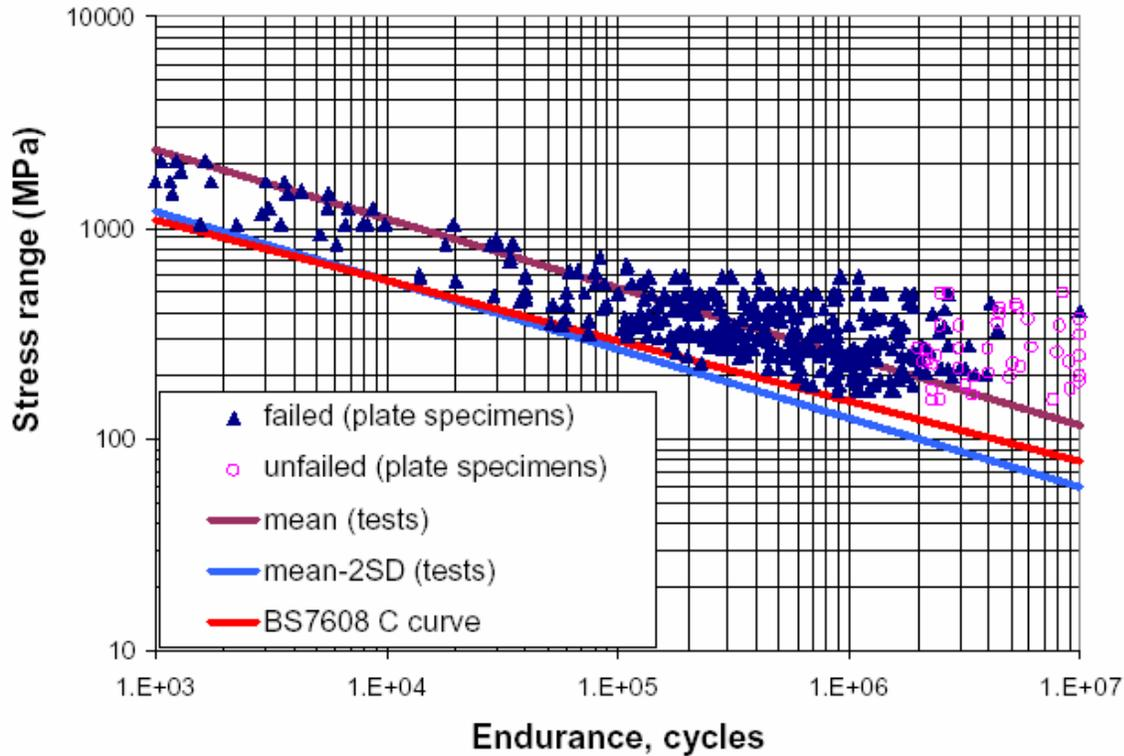
**Figure 3.1: Typical S-N Curve**
