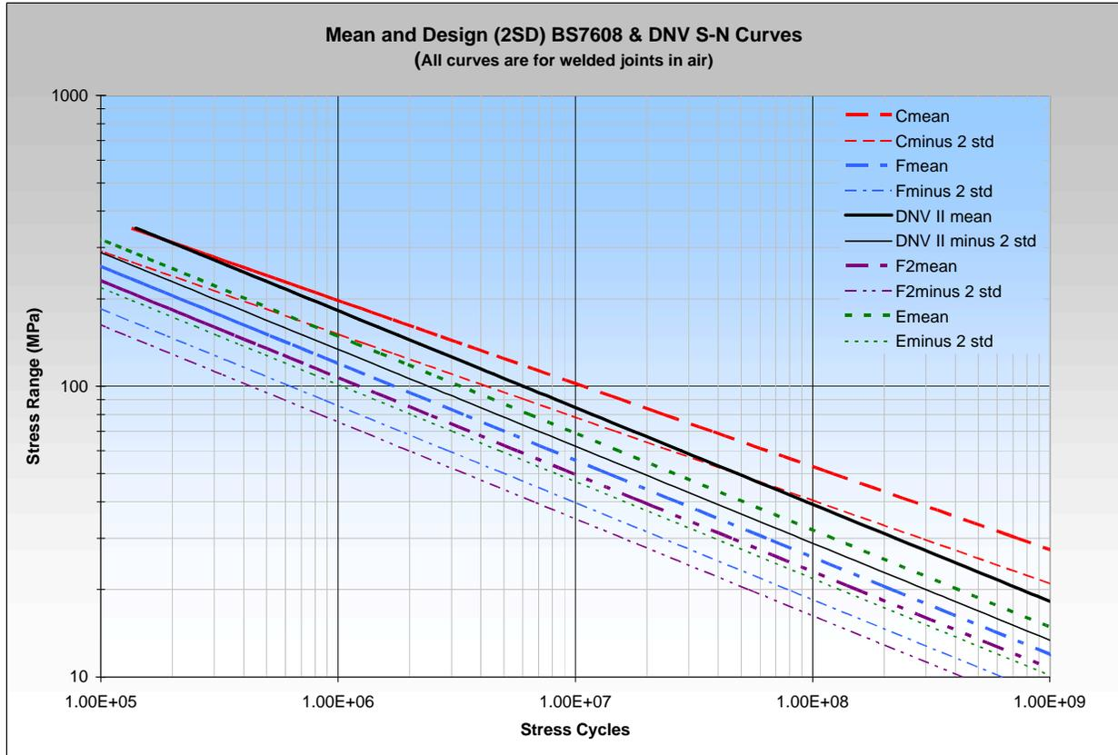
**Figure 6.2: S-N Design Curves Showing 2SD Offsets**
