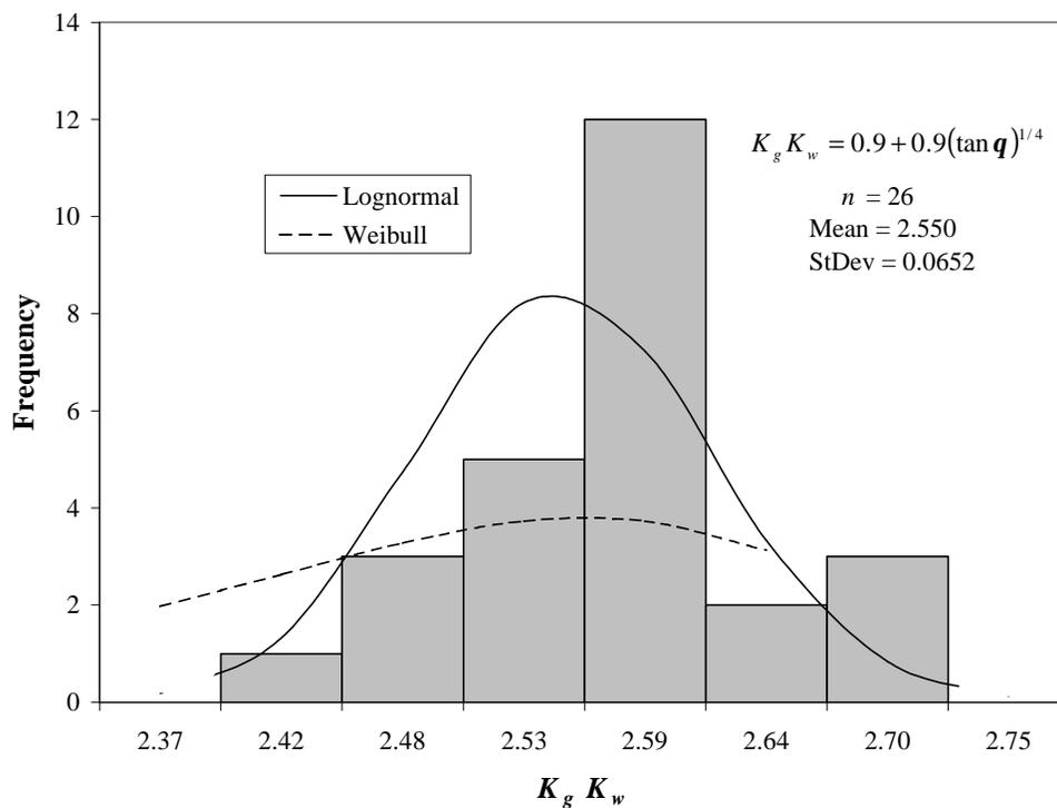
**Figure 5.11: Histogram of  $K_g K_w$  with Lognormal and Weibull Distribution Fits for Full Penetration Weld**
