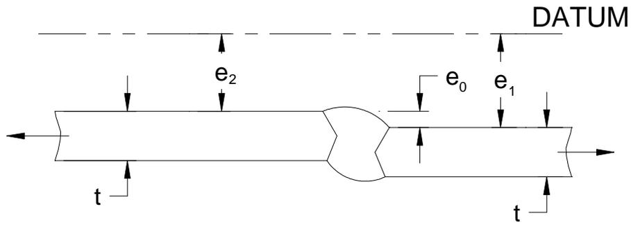
**Figure 3.3: Butt-Welded Plate Misalignment - Variables**
