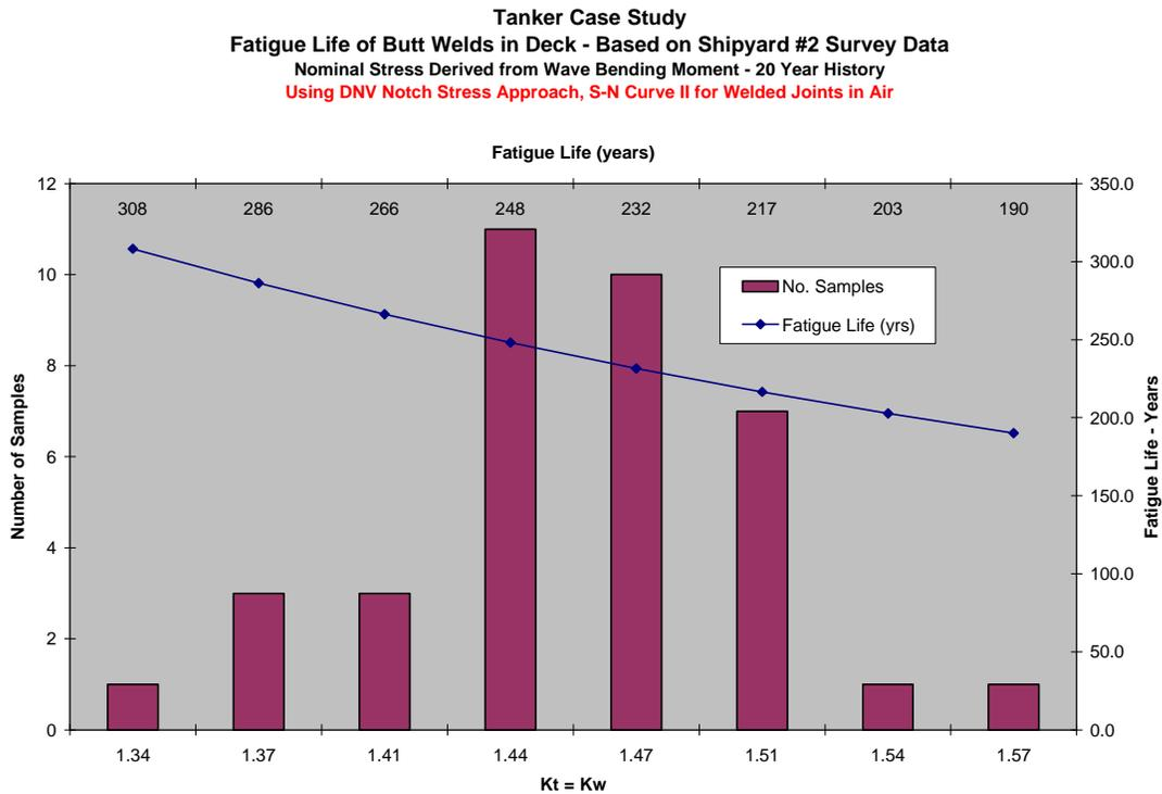
**Figure 7.6: Case 3 Fatigue Life Analysis with  $K_{total} = K_w$**
