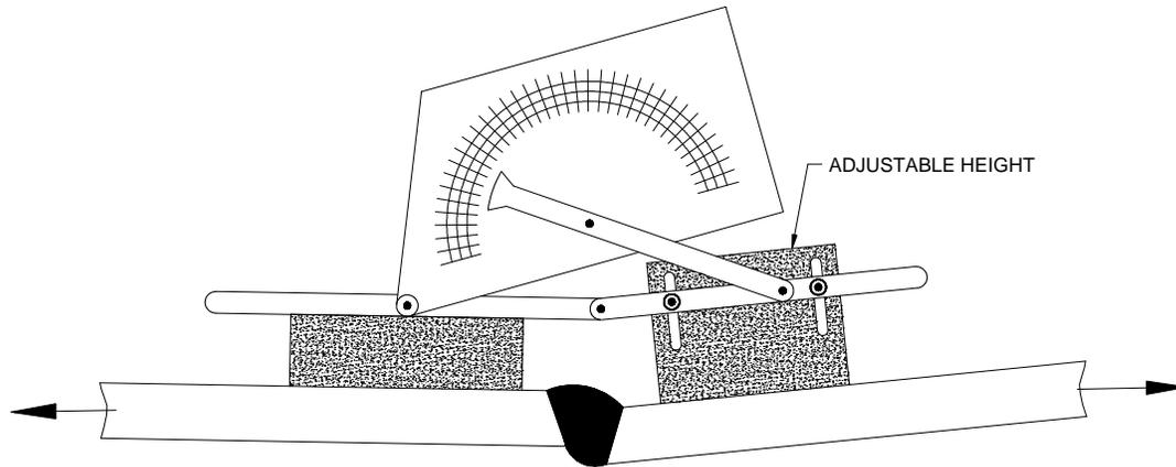
**Figure 4.5: Modified Protractor for Measuring Angular Misalignment**
