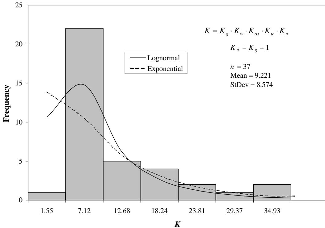
**Figure 5.13: Histogram of Total Stress Concentration Factor  $K$  with Normal and Lognormal Distribution Fits for Butt-Welded Plates (Shipyards #2)**
