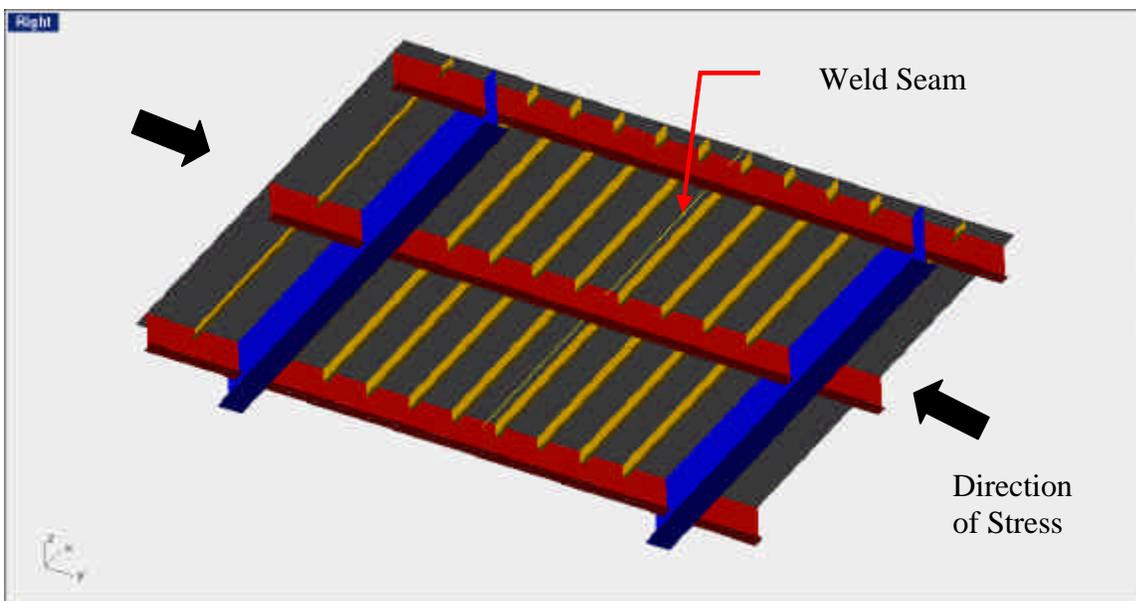
**Figure 6.1: Typical Butt Weld**
