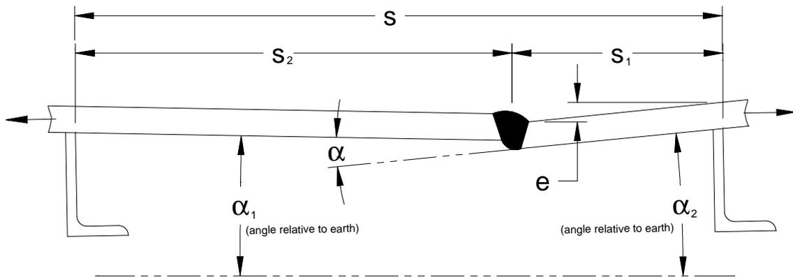
**Figure 3.4: Butt-Welded Plate Angular Misalignment - Variables**
