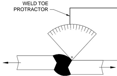
**Figure 4.3: Measuring Weld Toe Angle**
