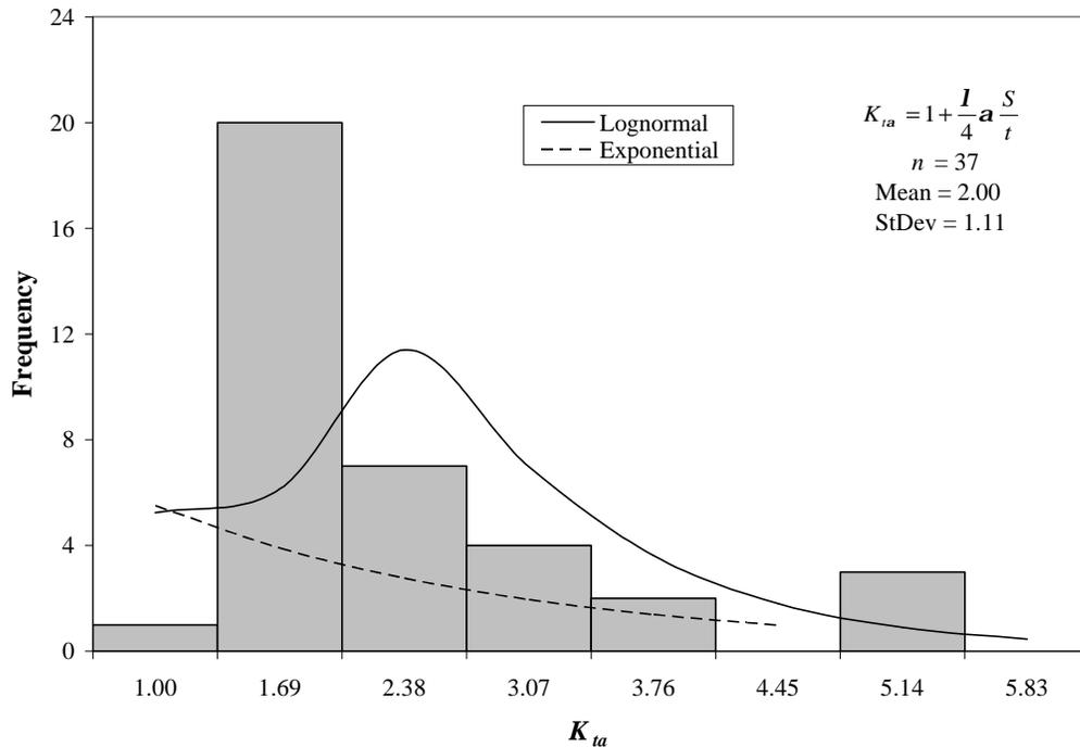
**Figure 7.3:  $K_{ta}$  Adjusted for Thickness, Fixity**
