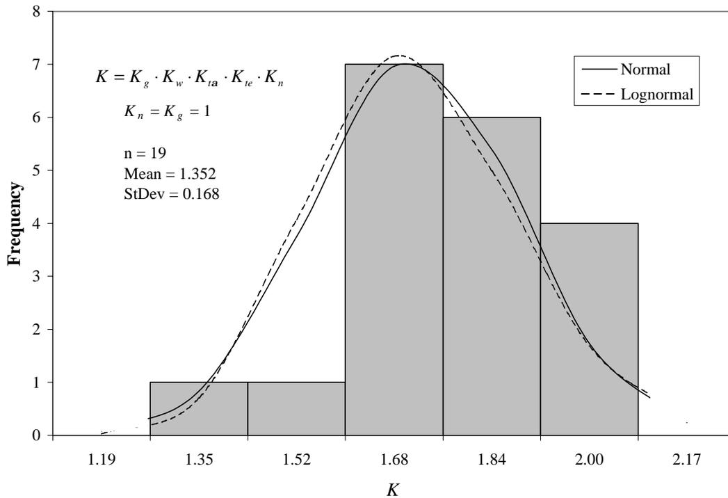
**Figure 5.12: Histogram of total Stress Concentration Factor  $K$  with Normal and Lognormal Distribution Fits for Butt-Welded Plates (Shipyards #1)**
