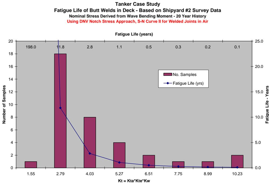
**Figure 7.4: Case 1 Fatigue Life Analysis with  $K_{total} = K_{ta} \cdot K_{te} \cdot K_w$**
