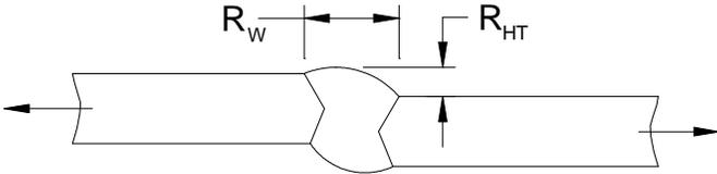
**Figure 3.6: Butt-Welded Plate Weld Reinforcement - Variables**
