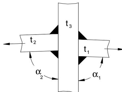
**Figure 3.9: Cruciform Joint Angular Misalignment – Variables**
