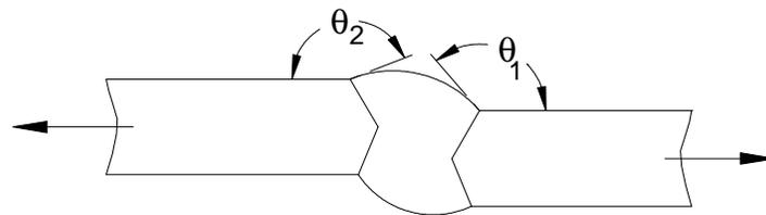
**Figure 3.5: Butt-Welded Plate Weld Toe Angle - Variables**
