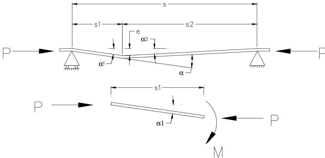
**Figure 3.11: Angularly Misaligned Plating - Seam at Location other than Halfway between Supports**
