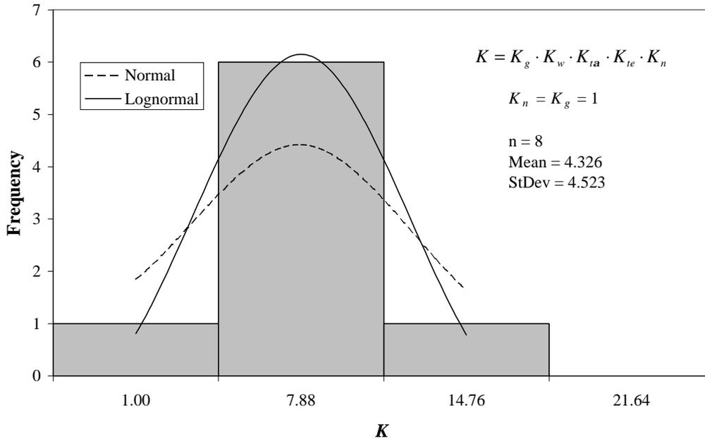
**Figure 5.14: Histogram of Total Stress concentration factor  $K$  with Lognormal and Normal Distribution Fits for Butt-Welded Stiffeners (Shipyards #2)**
