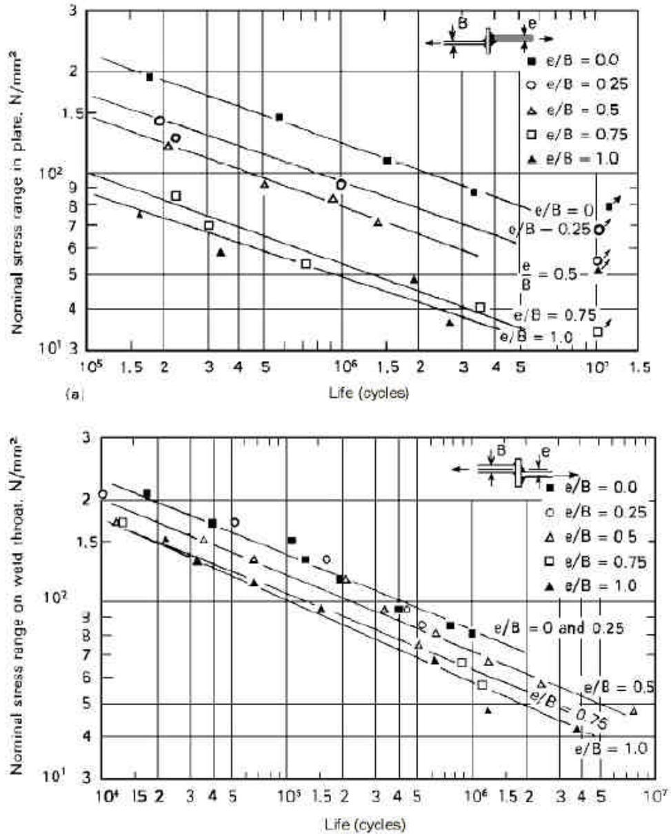
Figure 3.12: Effect of Misalignment on Fatigue Strength (Maddox, 1991)
