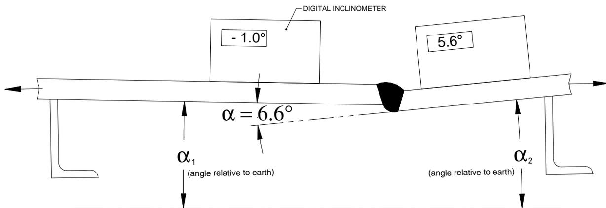
**Figure 4.4: Measuring Angular Misalignment**
