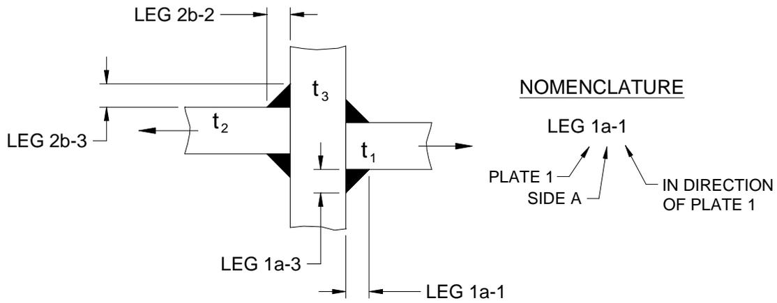
**Figure 3.8: Cruciform Joint Weld Geometry – Variables**
