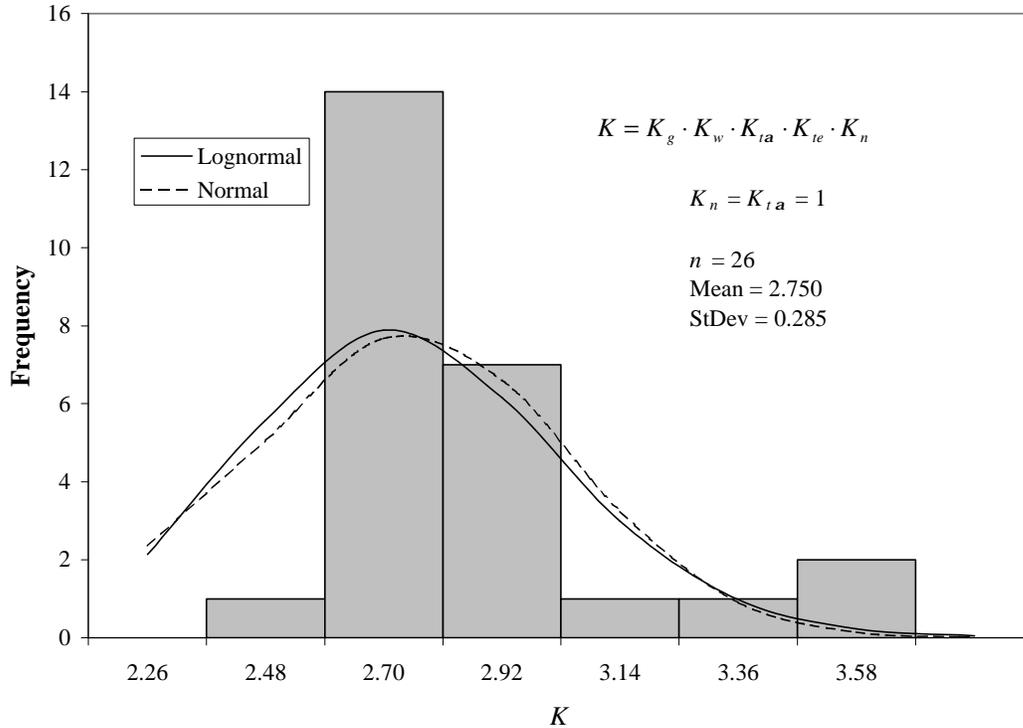
**Figure 5.16: Histogram of Total Stress concentration factor  $K$  with Lognormal and Normal Distribution Fits for Cruciform Joints, Full Penetration Weld (Shipyards #1 and #2)**
