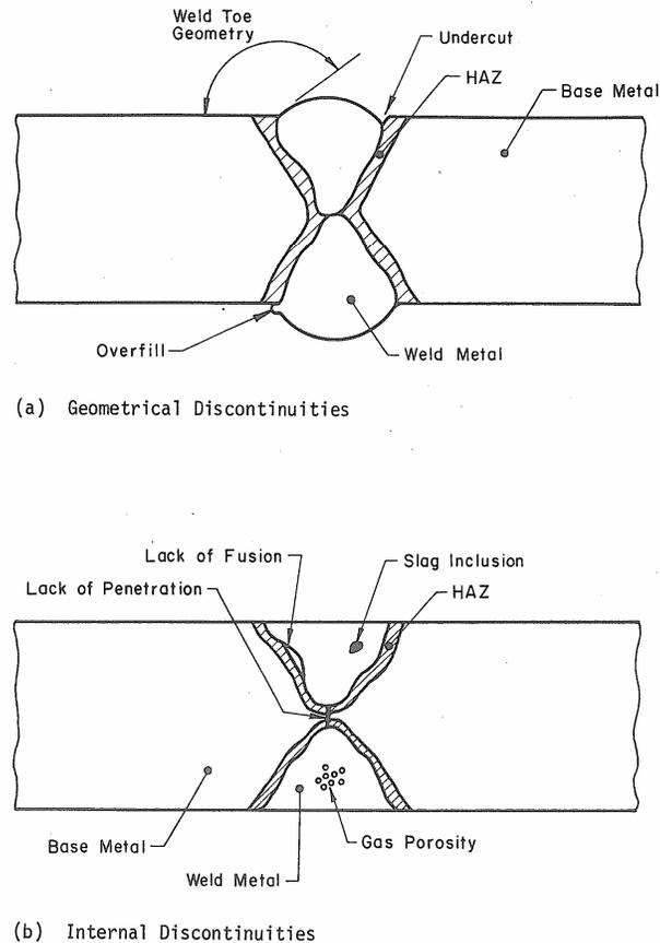
**Figure 3.2: Common Geometrical and Internal Weld Discontinuities**
