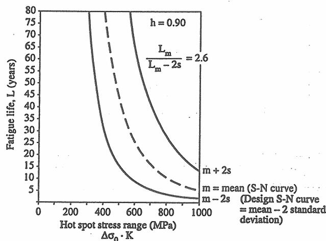
**Figure 3.13: Fatigue Life Influence of Stress Level and S-N Data for Welded Connections**
