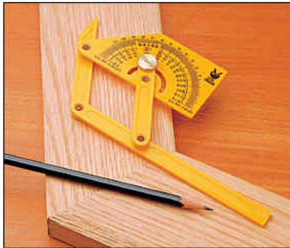
**Figure 4.7: Protractor for Measuring Angular Misalignment in Cruciform Joints**
