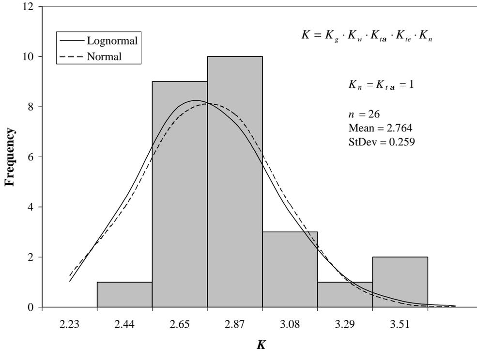
**Figure 5.15: Histogram of Total Stress concentration factor  $K$  with Lognormal and Normal Distribution Fits for Cruciform Joints, Fillet Weld (Shipyard #2)**
