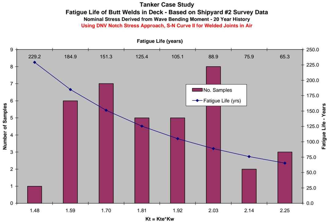
**Figure 7.5: Case 2 Fatigue Life Analysis with  $K_{total} = K_{te} \cdot K_w$**
