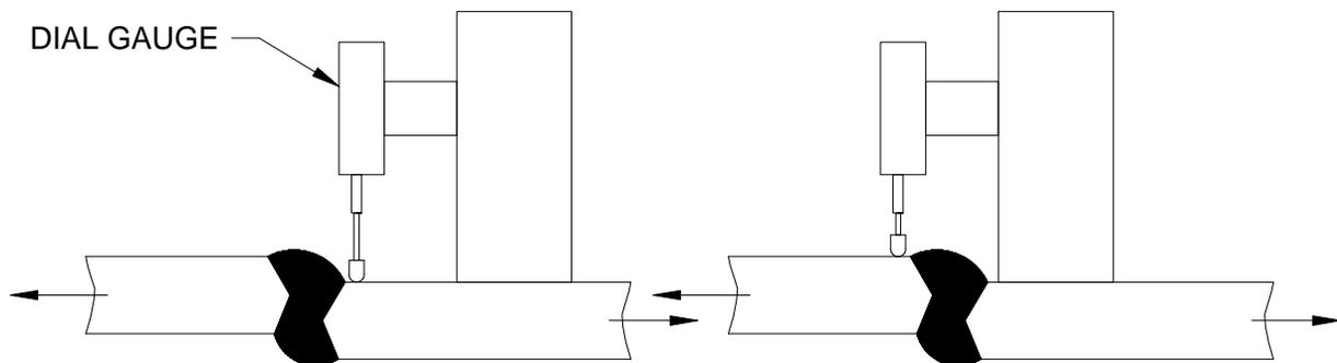
**Figure 4.1: Measuring Alignment and/or Weld Reinforcement Height**
