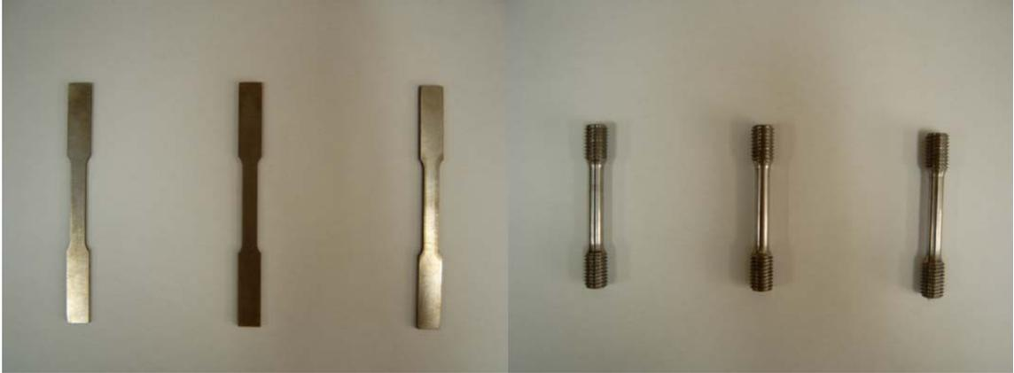
Fig. 96 Specimens of tensile test
