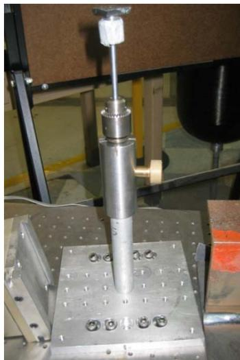
Figure 6.5: Nickel-reference sample in cadmium container
