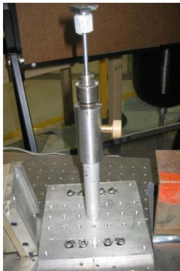
Figure 6.5: Nickel-reference sample in cadmium container
