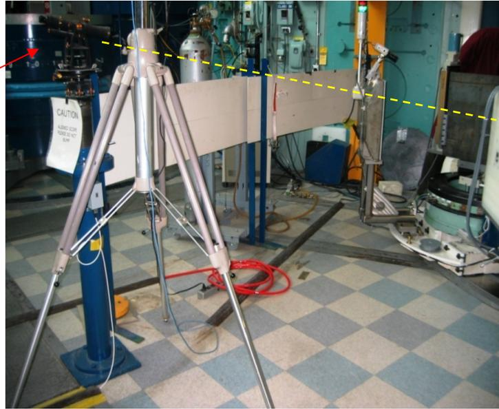
Figure 6.1: Tilted telescope pointed at the y-centre of rotation of the specimen
