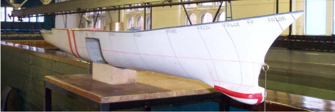
Figure 3-6: General view of the model for loading tests in damaged conditions
