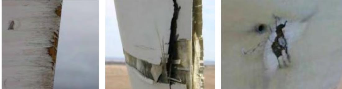
**Figure 73. Wind blade damage showing: Leading Edge Erosion, Severe Blade Damage (left) , Delamination (center) and Lightning Damage to Blade [Knight & Carver]**
