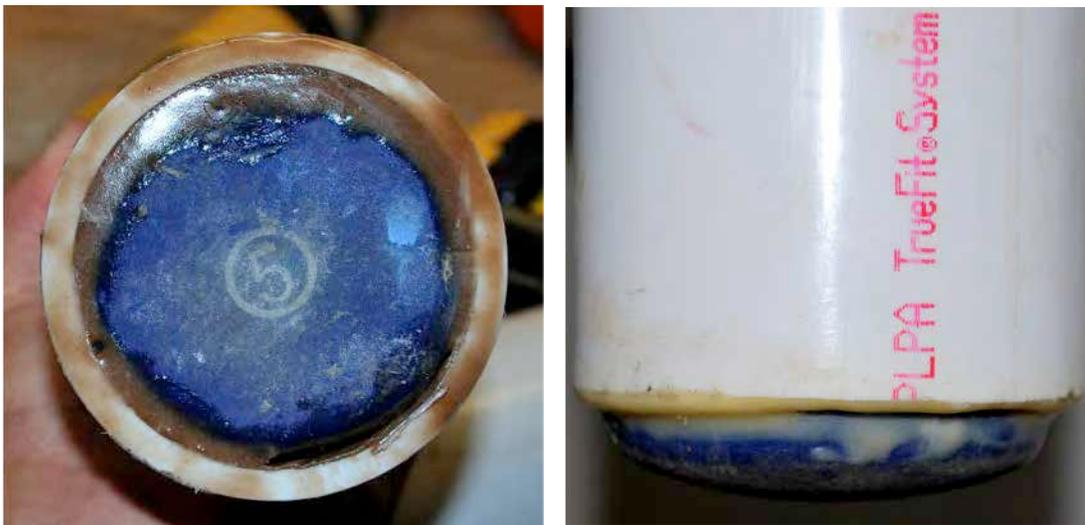
**Figure 93. Rubber coated barbell is epoxied into PVC tube to form impactor**
