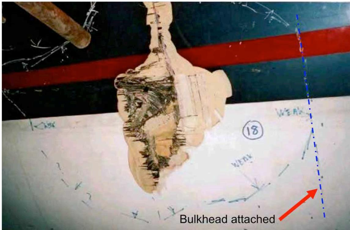
**Figure 119. Full extent of internal damage to hull sandwich construction [Laser Technology, Inc.]**
