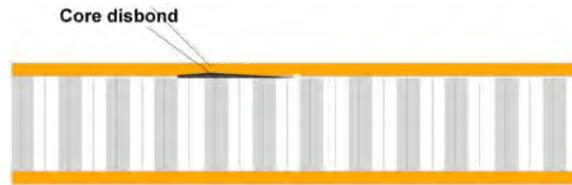
Figure 37. Schematic of skin-to-core disbond [NetComposites 2004]
