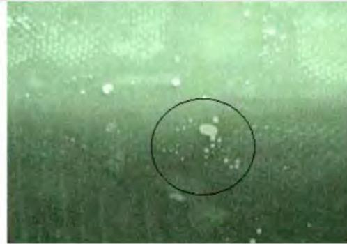
Air bubbles trapped during hand layup that were removed by sanding [Boat-Project.com, 2001]
