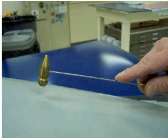
**Figure 46. Picture of a military specification tap hammer [Courtesy of Abaris Training Resources Incorporated]**
