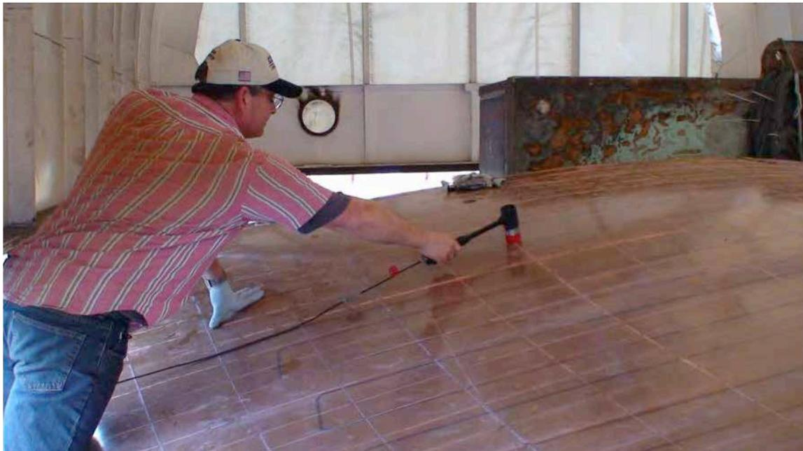
**Figure 55. An instrumented hammer is used to excite a composite destroyer rudder during SIDER examination [author photo]**
