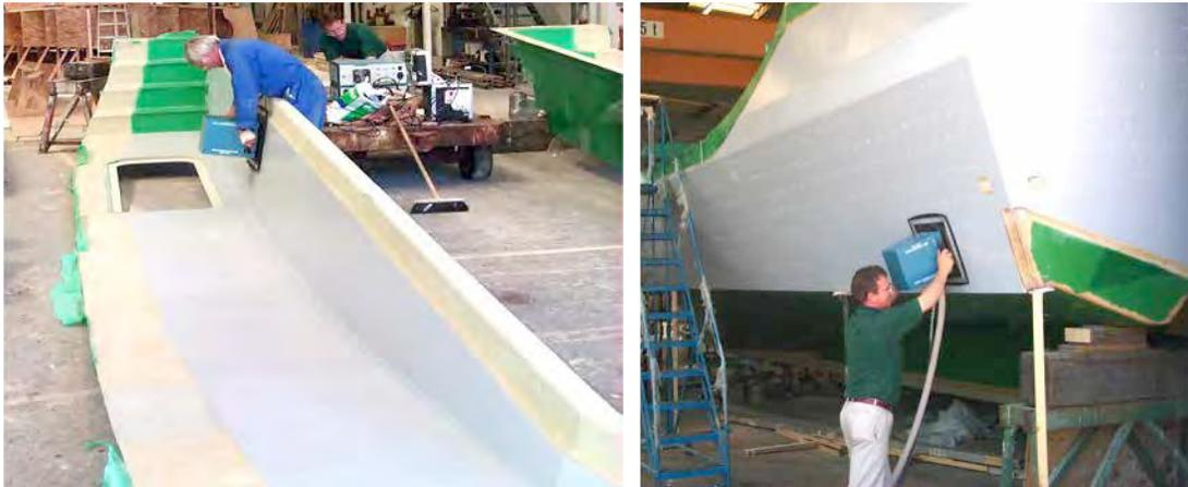
**Figure 116. Vacuum hood used to test flat panel portions of RNLI lifeboat hulls [Laser Technology, Inc.]**
