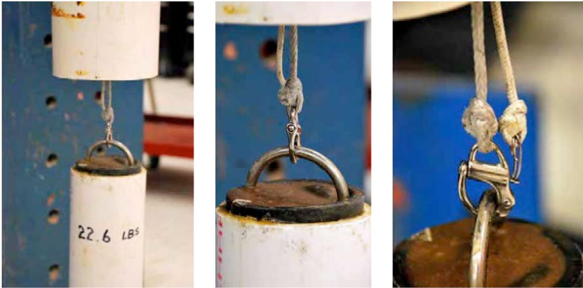
Figure 94. Detail of impactor release mechanism
