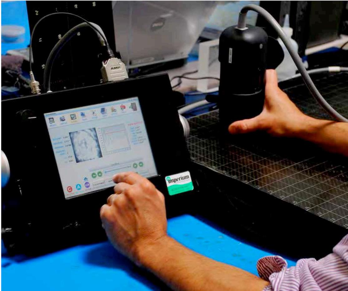
**Figure 106. Acoustocam i600 used to inspect a project carbon fiber panel with simulated delaminations [author photo]**
