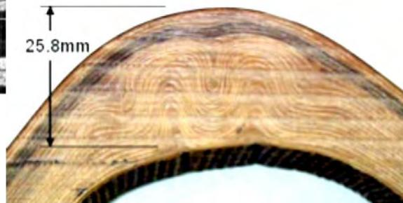
Figure 33. Composite sample close-up of apex showing extreme fiber-waviness [Anastasi 2008]
