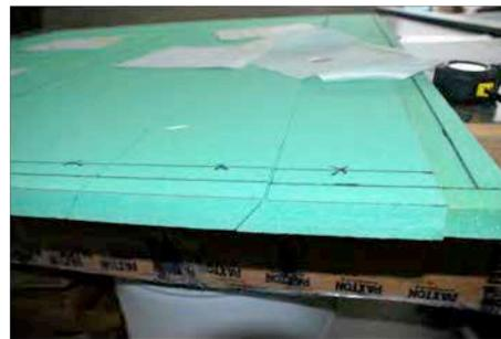
45° saw cuts (3, 6 and 12 inches long) in core used to simulate core shear failure
