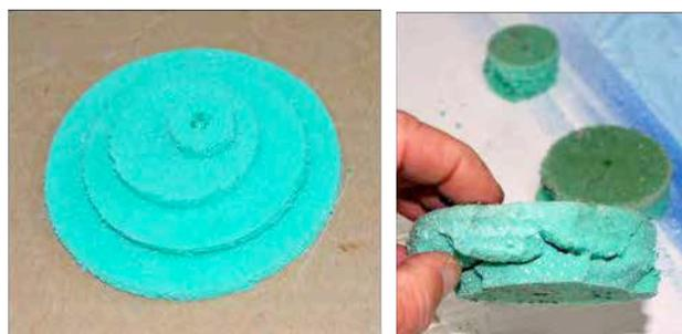
Removed core (left) and replacement plugs (right) used to entrap water behind skin
