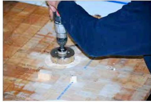
Hole saw is used to create a 1/8 inch deep void for water to be encapsulated
