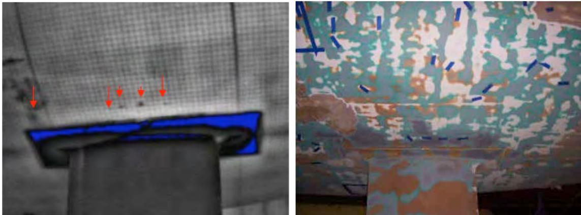
**Figure 124.** This IR image shows that moisture ingress on the starboard side of the keel box has not migrated further than the local area. The red arrows show laminate anomalies that were confirmed to be “resin starved” areas. [Independent Marine Systems]
