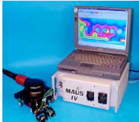
**Mobile Automated Scanner (MAUS IV) UT C-scan or Low-Frequency Bond Tests (LFBT)**
