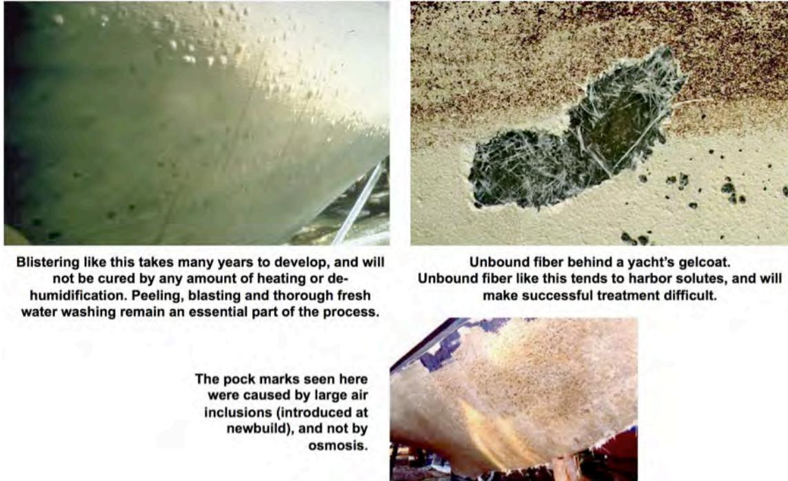
Figure 5. Illustration of blisters in boat hulls [Clegg 2009]
