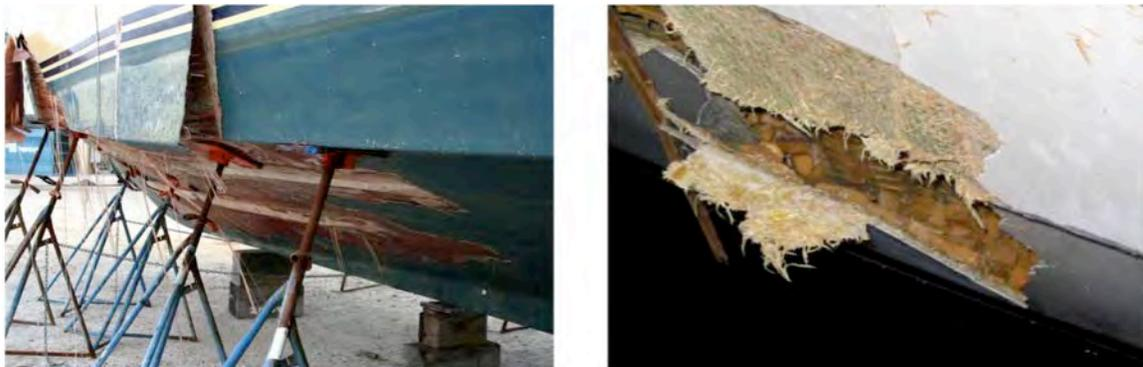
**Figure 11. Examples of severe delamination resulting from manufacturing defects [www.yachtforums.com]**
