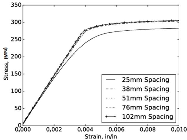
Figure 28: HAZ Tensile Coupons of 6061 Plate
