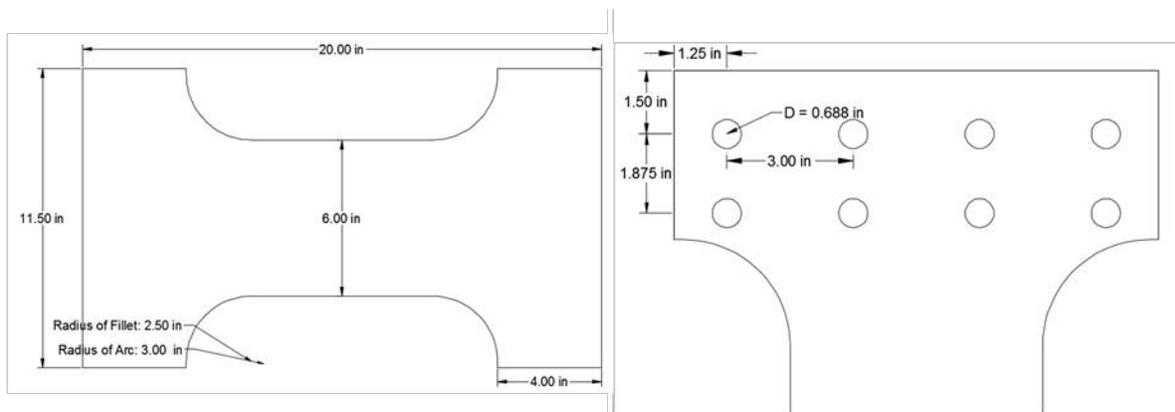
**Figure 8: Overall dimensions of the non-load carrying fillet welded connection along with the edge and spacing distances for the proposed bolt pattern.**
