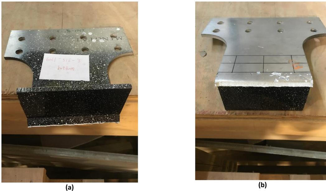
Figure 61: Specimen F3 Showing Failure at the Weld Toe
