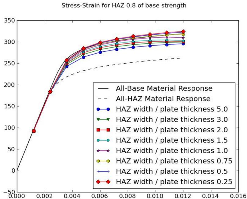
Figure 4: 6082 Material (n=32) HAZ 80% of Base Strength
