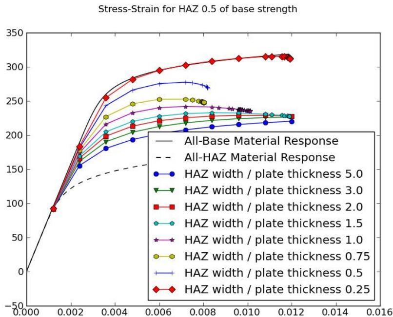
Figure 2: 5083 Material (n=16), HAZ 50% of Base Strength
