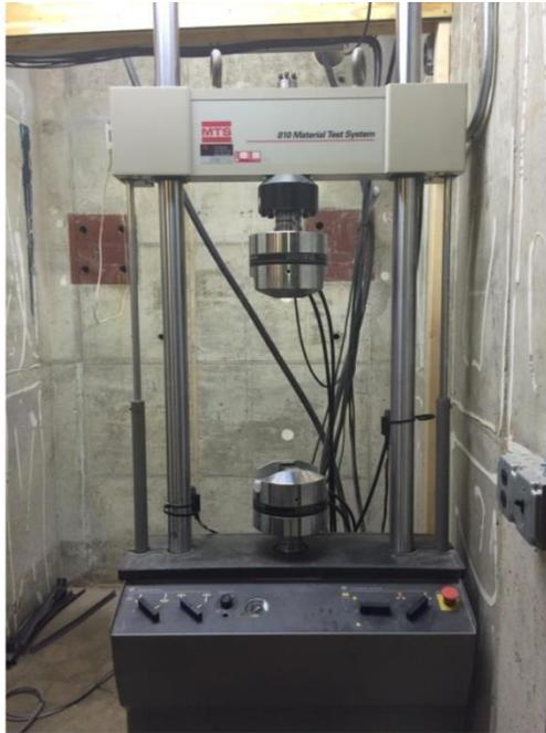
Figure 15: MTS 810 Machine Used for Material Coupon Testing
