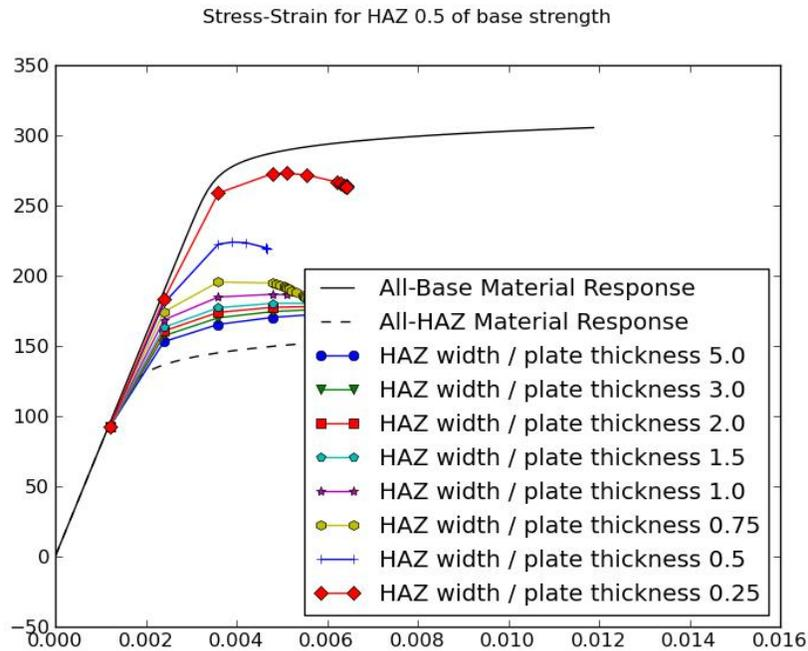
Figure 3: 6082 Material (n=32) HAZ 50% of Base Strength
