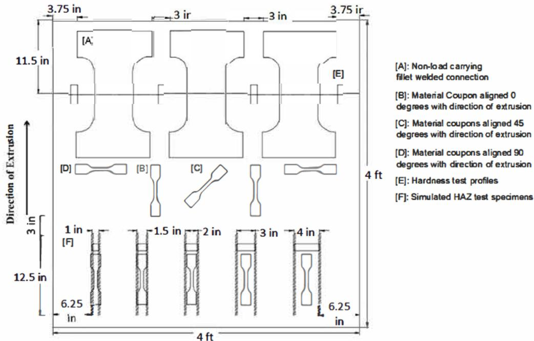
**Figure 10: Sample specimen layout on square specimen showing three large NLCFWC specimens and supporting specimens. Note that the distribution of specimen types B, C, D vary plate-to-plate to produce five specimens of each type.**
