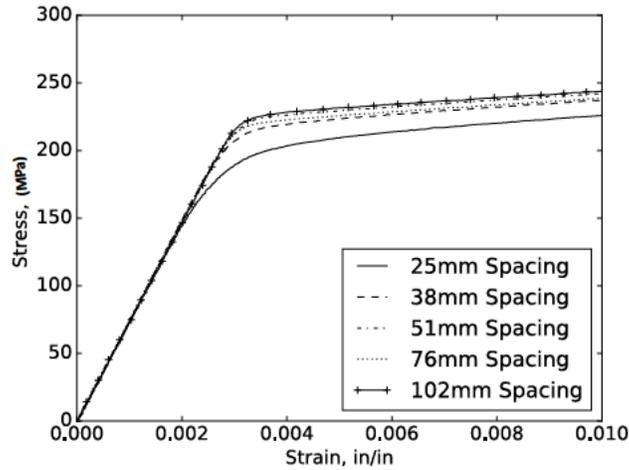
Figure 27: HAZ Tensile Coupons of 5086 Plate
