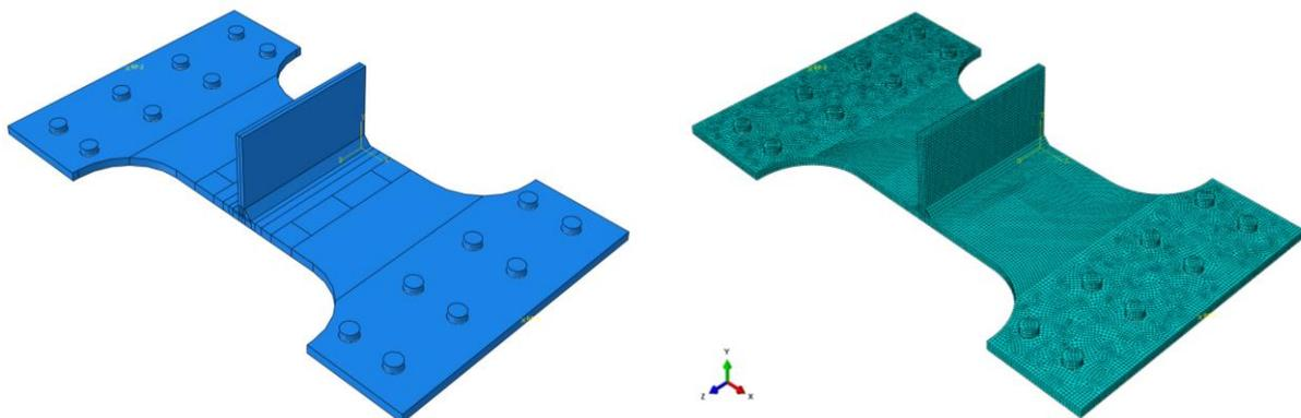
Figure 62: Abaqus FEA Model and Model Mesh
