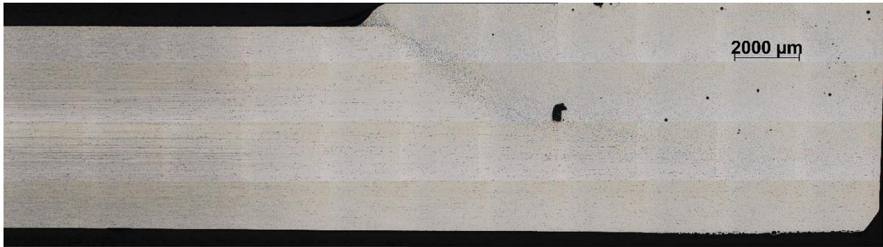
**Figure 8.** Porosity and large voids in a corrosion repair simulant plate.
