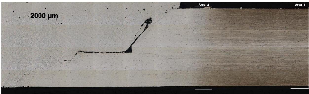
**Figure 7.** Cross section of corrosion repair plate showing a large lack of fusion defect.
