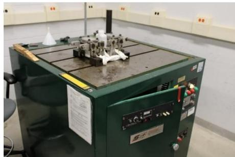
**Figure 2.** Sonntag SF-1U unit with seawater specimen loaded into machine.
