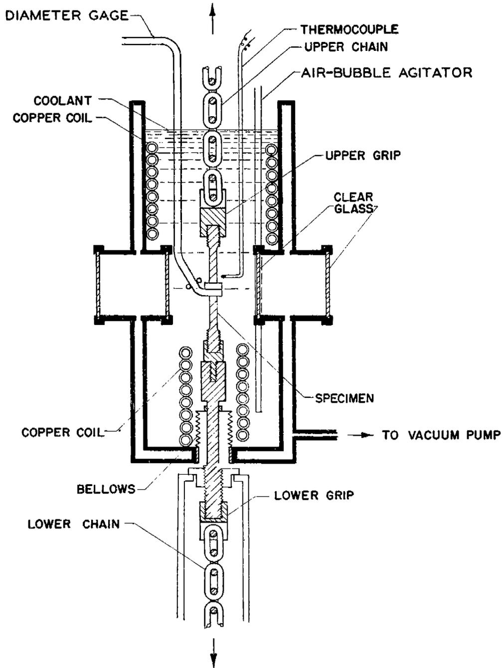
FIG. 3 SCHEMATIC DIAGRAM OF TENSILE TEST APPARATUS
