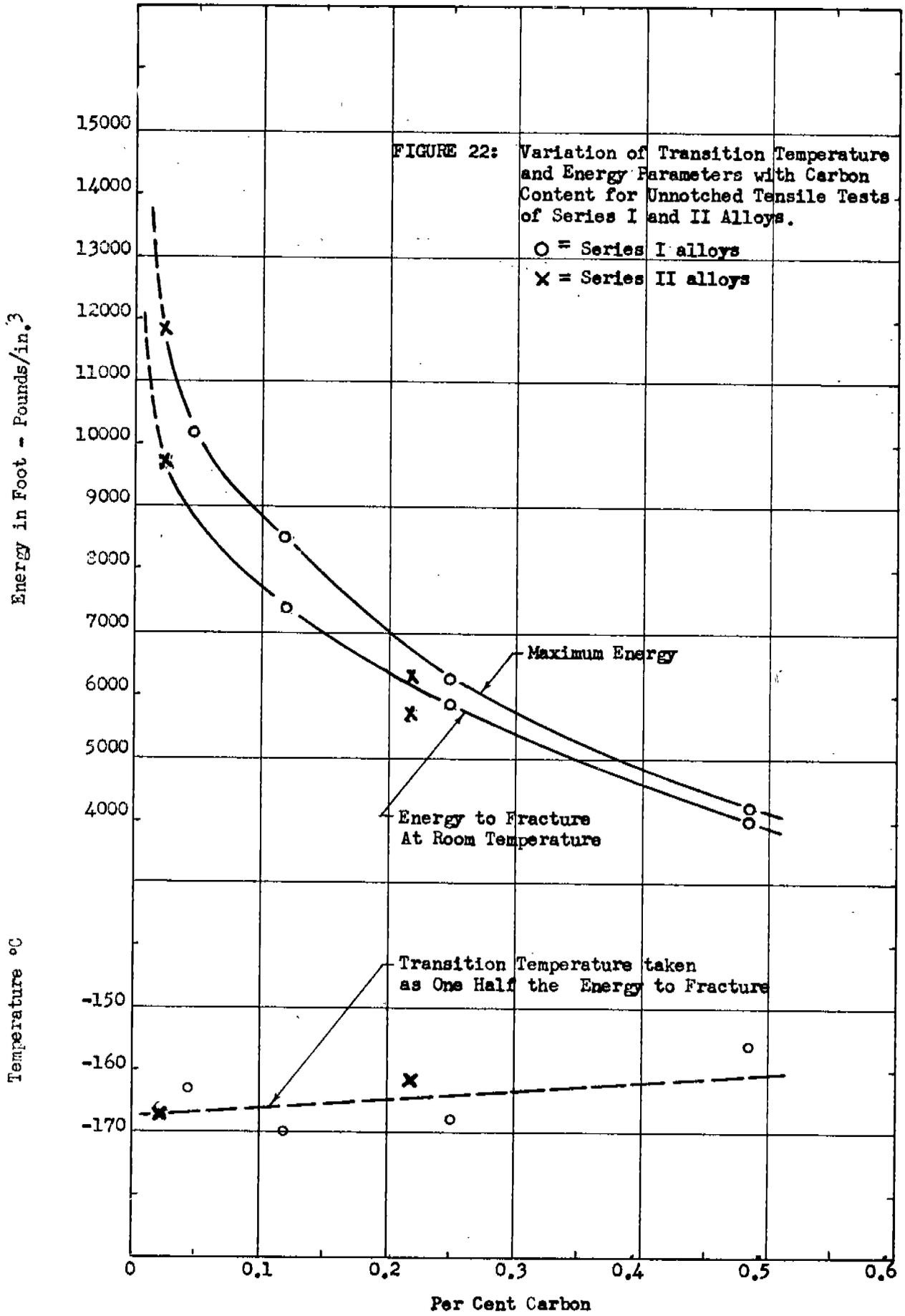
FIGURE 22: Variation of Transition Temperature and Energy Parameters with Carbon Content for Unnotched Tensile Tests of Series I and II Alloys.
