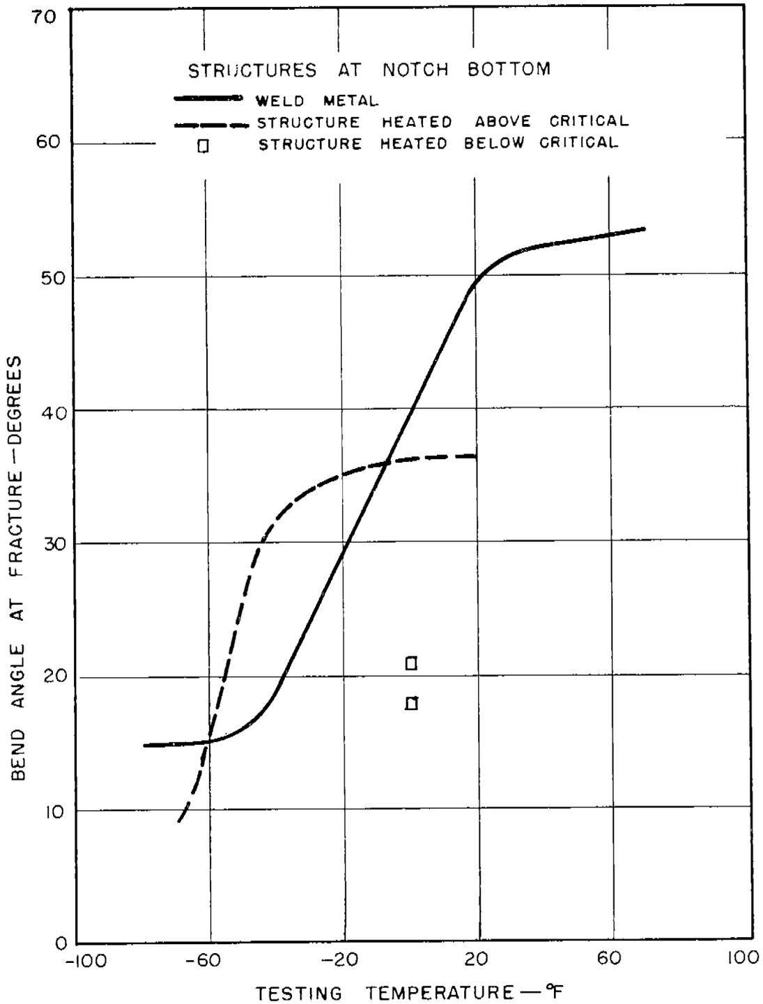
FIG. 14: EFFECT OF TEMPERATURE ON DUCTILITY OF SINGLE BEAD-ON-PLATE SPECIMEN (FOUNTAIN AND STOUT)
