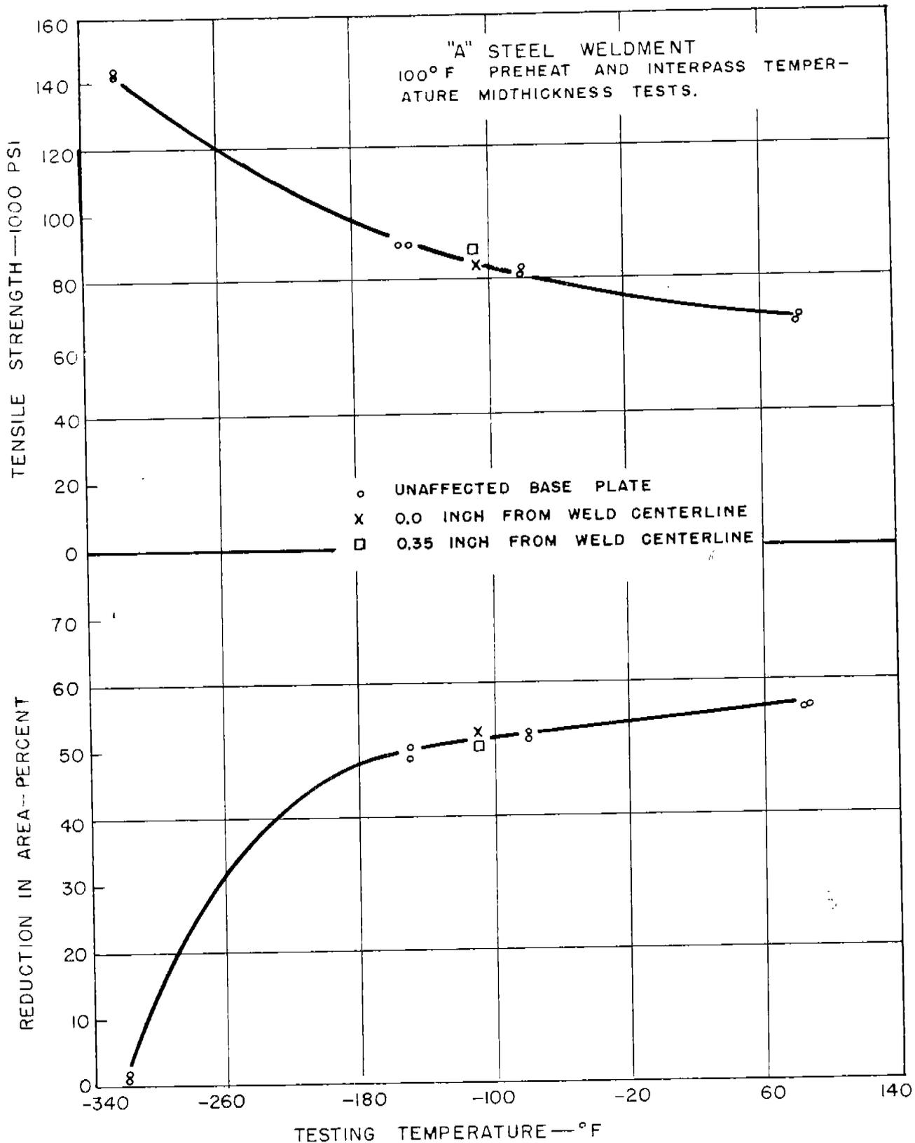
FIG. 12: REGULAR TENSILE PROPERTIES OF "A" STEEL AS A FUNCTION OF TESTING TEMPERATURE.
