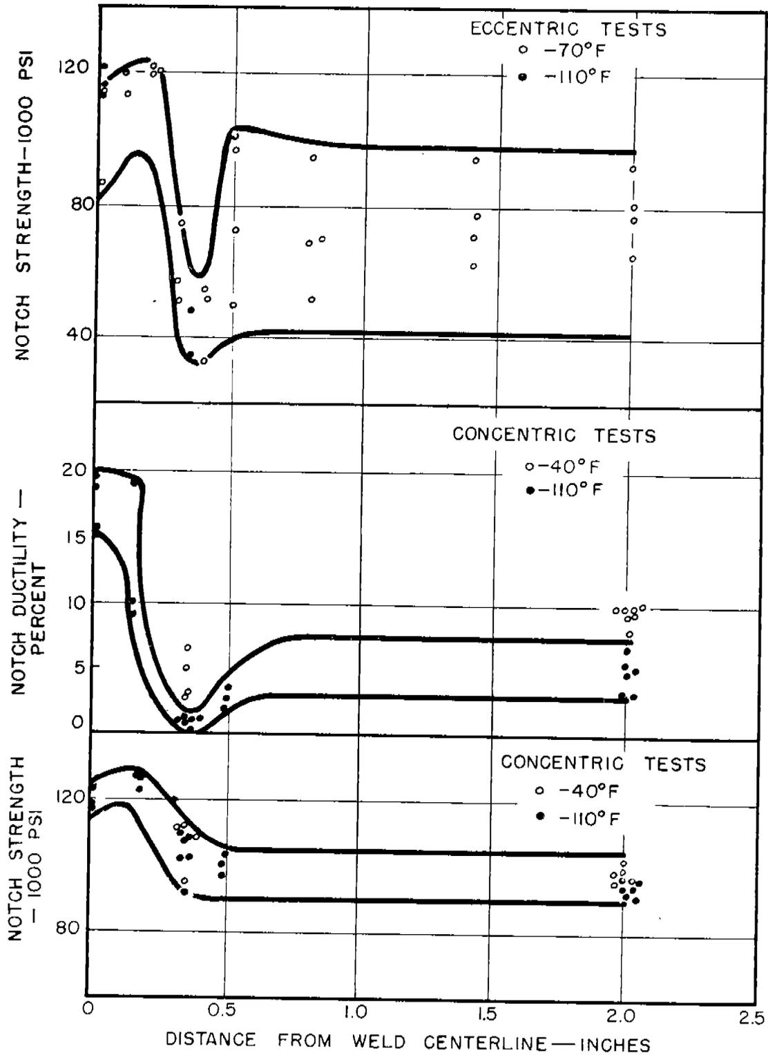
FIG. 13: DISTRIBUTION OF CONCENTRIC AND ECCENTRIC NOTCH PROPERTIES AT VARIOUS LOW TEMPERATURES—MIDTHICKNESS TESTS OF "A" STEEL WELDMENTS, (100°F PREHEAT AND INTERPASS TEMPERATURES)
