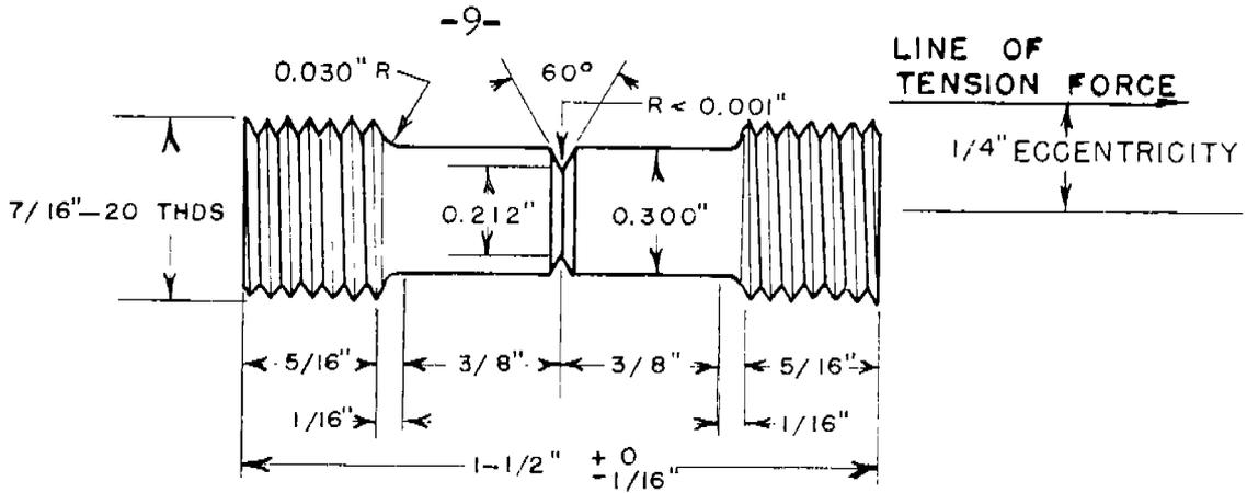
ECCENTRIC NOTCH TENSILE SPECIMEN
