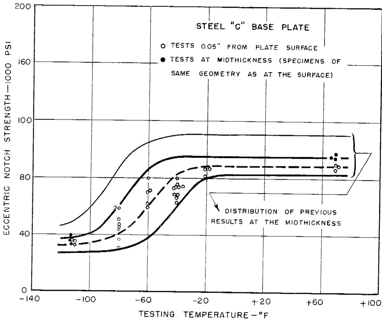
FIG. 8: ECCENTRIC NOTCH STRENGTH OF THE UNAFFECTED BASE PLATE AS A FUNCTION OF TESTING TEMPERATURE.
