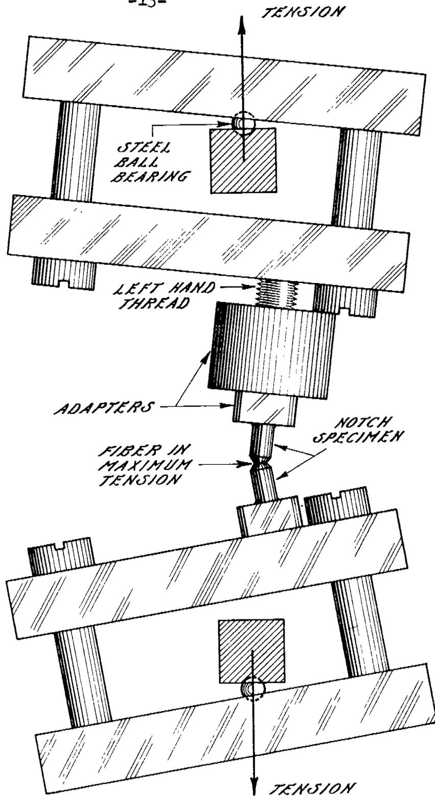
FIG. 6: METHOD OF LOADING TO OBTAIN 1/4 INCH ECCENTRICITY (ECCENTRICITY AND THE POSITION OF FIXTURES ARE EXAGGERATED).
