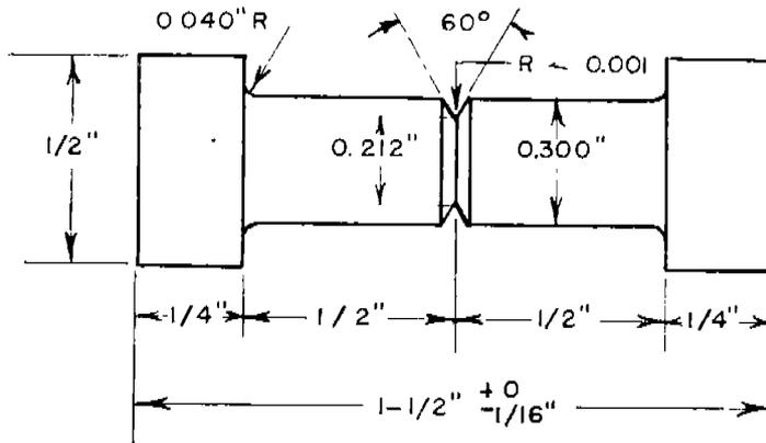
CONCENTRIC NOTCH TENSILE SPECIMEN
