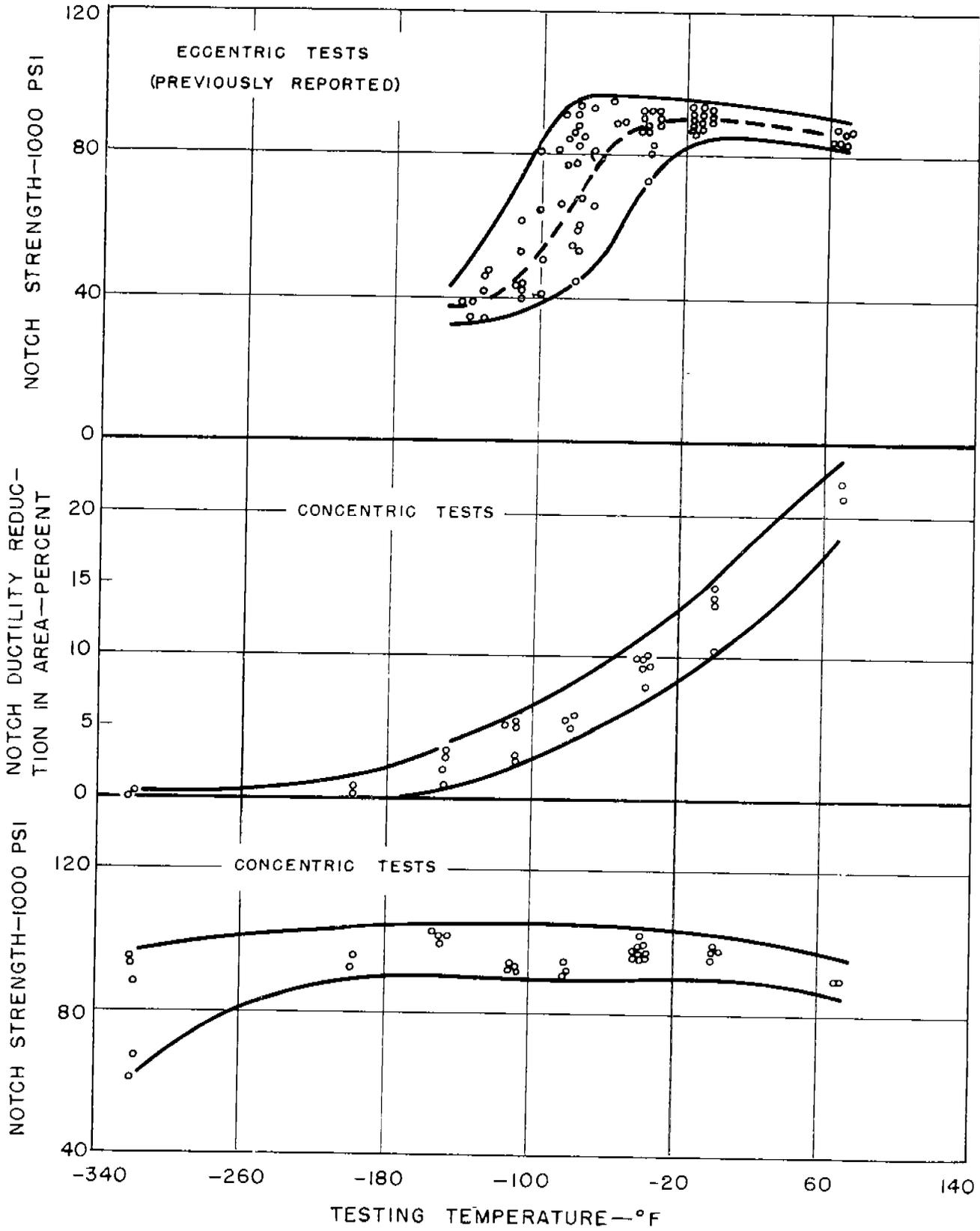
FIG. II: COMPARISON OF THE ECCENTRIC AND CONCENTRIC NOTCH PROPERTIES AS A FUNCTION OF TESTING TEMPERATURE. MIDTHICKNESS TESTS OF "A" STEEL BASE PLATE.
