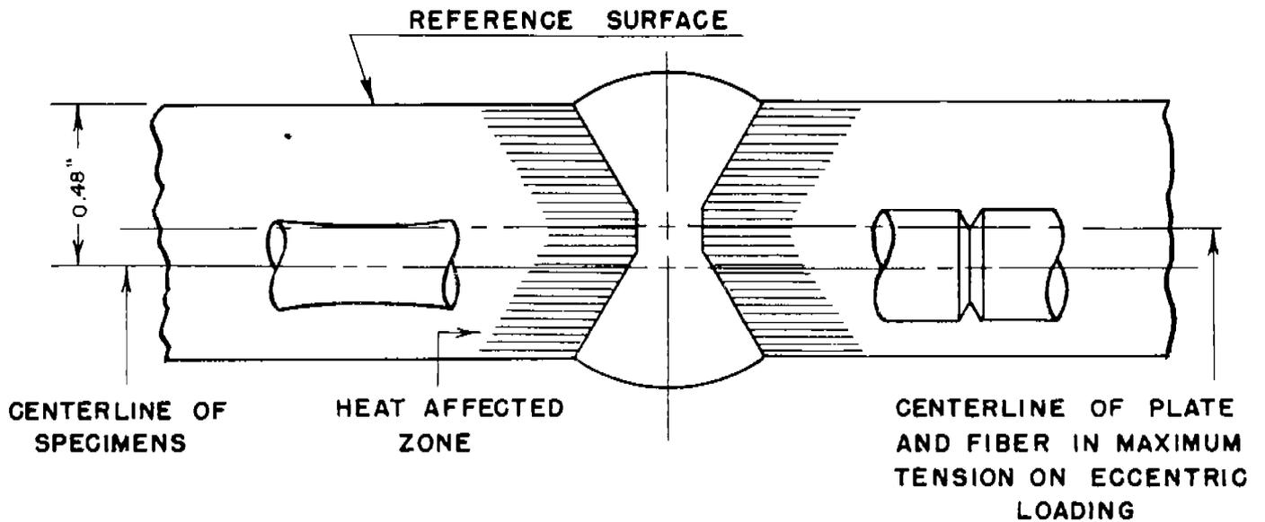
FIG. 5: LOCATION OF UNNOTCHED AND NOTCHED SPECIMENS AT THE MIDTHICKNESS OF WELDMENT
