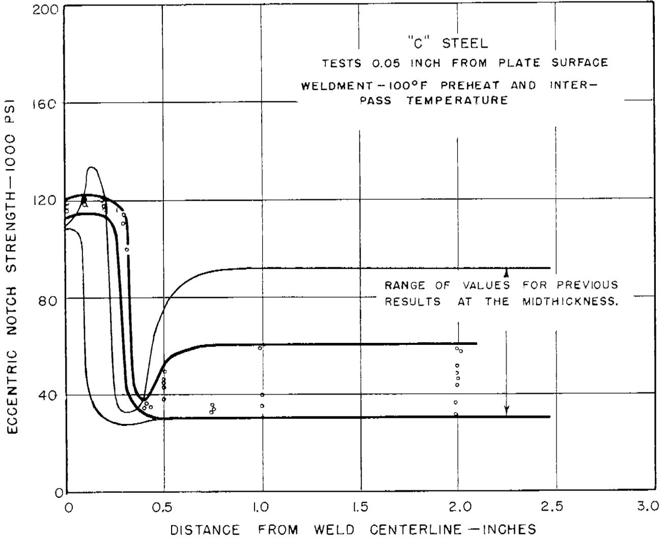
FIG. 9: DISTRIBUTION OF ECCENTRIC NOTCH STRENGTH AT -80°F
