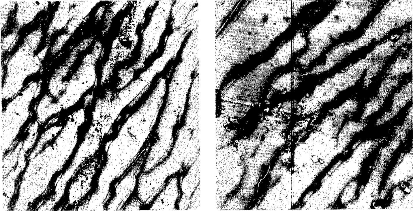
Figure 2. The Fractured Surfaces of a Tear Test A Steel Specimen Broken at 10 F Were Micrographed in the Brittle Region, the Left Micrograph First and the Right at a Later Date, to Indicate the Reliability of the Replica Technique. (X5000)
