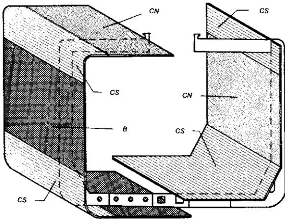
Fig. III. STRUCTURAL MATERIALS ARRANGEMENT CONCH CONTAINMENT SYSTEM
