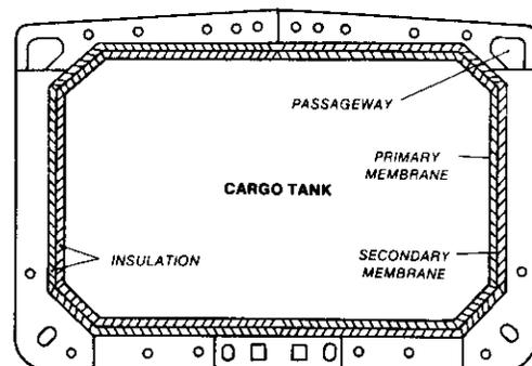
Fig. IV TYPICAL SECTION OF GAZ TRANSPORT MEMBRANE TANK DESIGN
