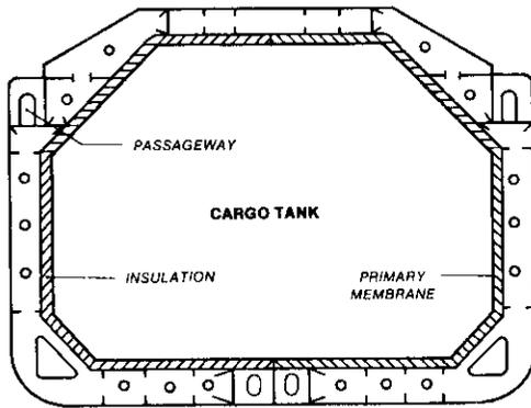
Fig. V. TYPICAL SECTION OF TECHNIGAZ MEMBRANE TANK DESIGN
