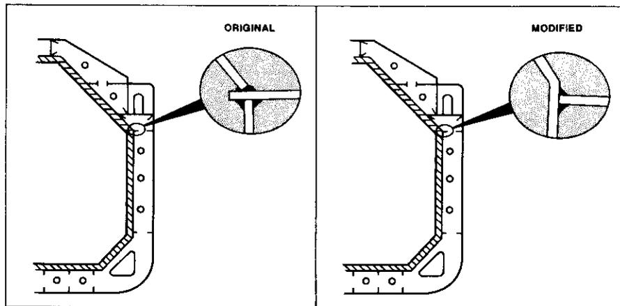
Fig. VII. STRUCTURAL DETAIL, WELDING DESIGN
