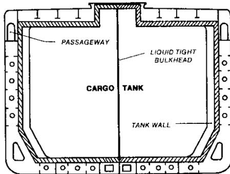
Fig. VI. TYPICAL SECTION OF CONCH FREE-STANDING TANK DESIGN
