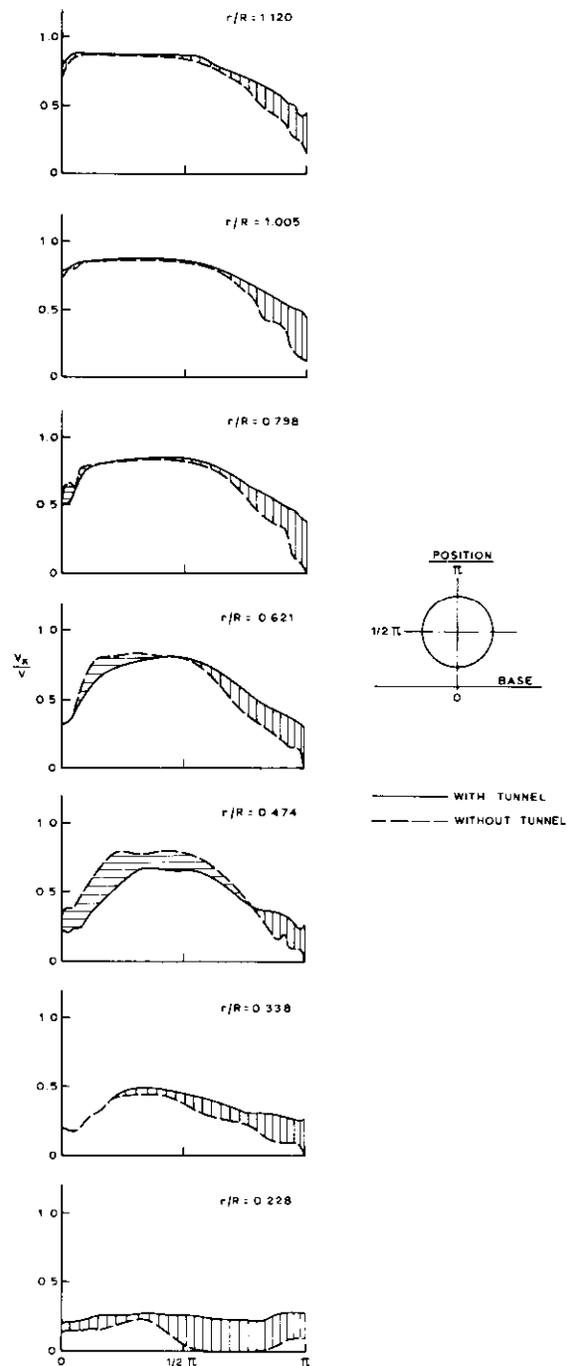
Fig. 3. Effect of partial stern tunnel on gradient in nominal wake field at top position (axial wake velocity only) for container ship B of Figure 4 /12/.
