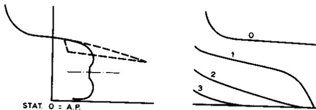
Fig. 4. Partial body plans of various second generation container ships.
