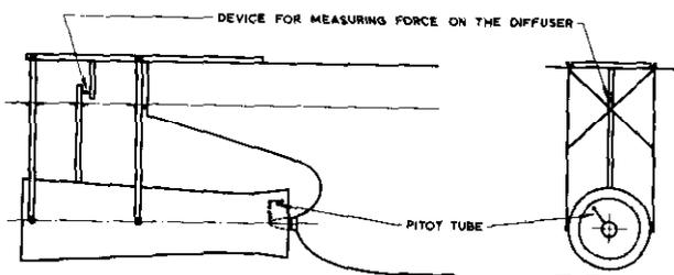
Fig. 11. Test set-up adopted to measure simulated effective wake field /9/.
