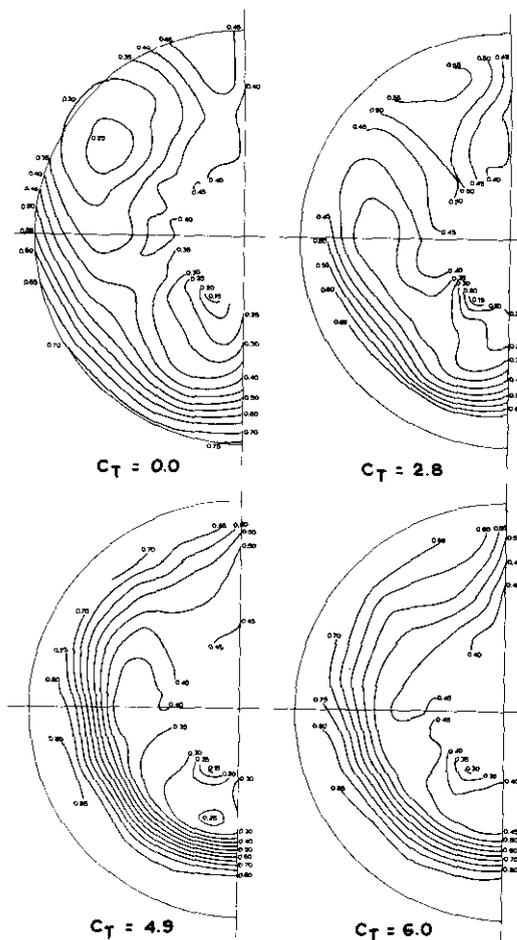
Fig. 12. Axial velocity distributions of nominal ( $C_T = 0.0$ ) and simulated effective wake fields ( $C_T = 2.8, 4.9$  and  $6.0$ ) /9/.
