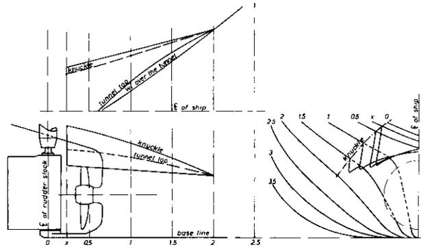
Fig. 9. Tunnel construction adopted to improve wake field of a dredger to reduce hull vibrations /12/.
