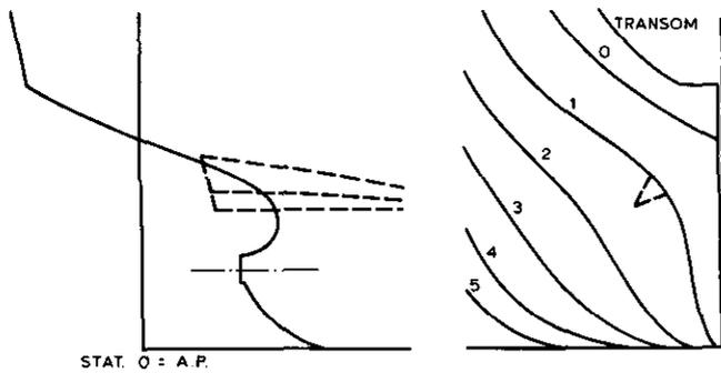
Fig. 17. Partial body plan of a 80,000 DWT bulk carrier.
