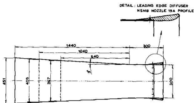
Fig. 10. Geometry of diffusers used to simulate flow-sucking action of propeller /9/.
