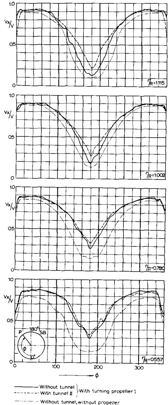
Fig. 16. Circumferential distribution of axial velocity components behind model of Great Lakes carrier /8/.
