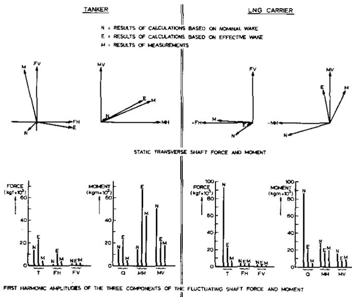
Fig. 14. Comparison of calculated and measured components of the shaft forces and moments /9/.
