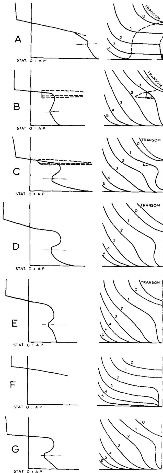
Fig. 2. Partial body plans of various 120.000 m<sup>3</sup> LNG carriers
