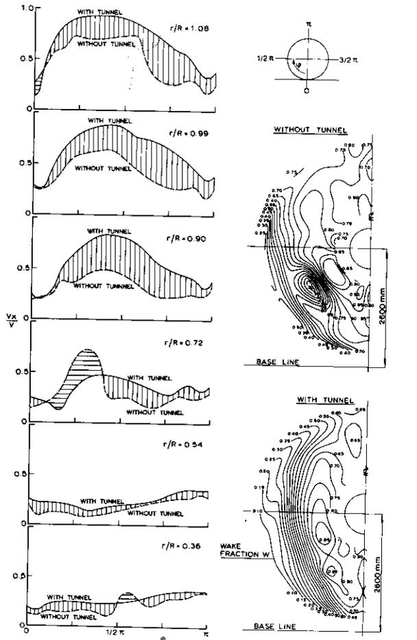
Fig. 8. Effect of partial stern tunnel on homogeneity of the nominal wake field (axial wake velocity only) of the dredger of Figure 7 /12/.
