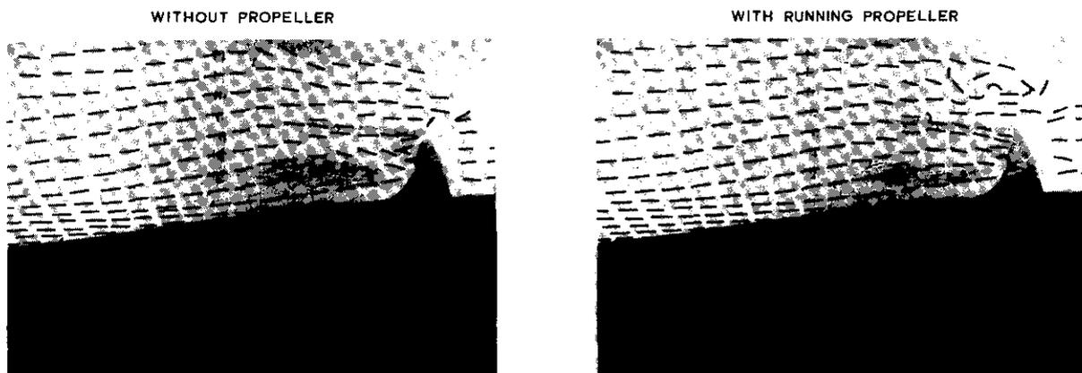
Fig. 19. Results of flow visualization tests on model of 80,000 DWT bulk carrier with and without running propeller (with partial stern tunnel) - for reasons of clarity, the tuft positions have been retouched.
