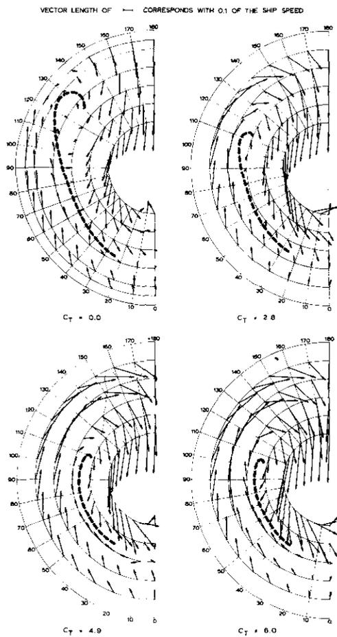
Fig. 13. Transverse velocity components in nominal ( $C_T = 0.0$ ) and simulated effective wake fields ( $C_T = 2.8, 4.9$  and  $6.0$ ) /9/.
