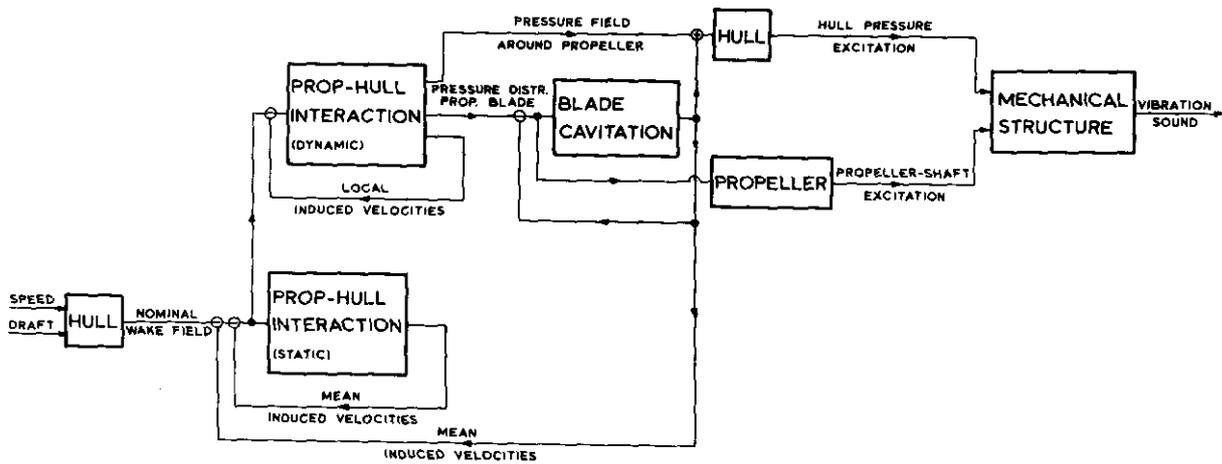
Fig. 1. Block diagram showing the interrelationship between the parameters affecting propeller-generated vibrations and sound on board of ships
