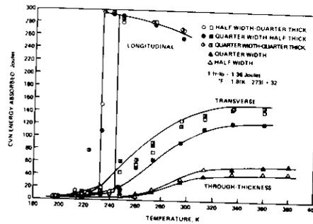
Fig. 6A-2 Charpy V-Notch Impact Energy Curves of Longitudinal, Transverse, and Through-Thickness Specimens of Steel 8 (0.11C, 0.013S).
