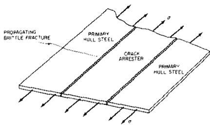
Fig. 2A Typical Geometry of In-Plane Crack Arrester
