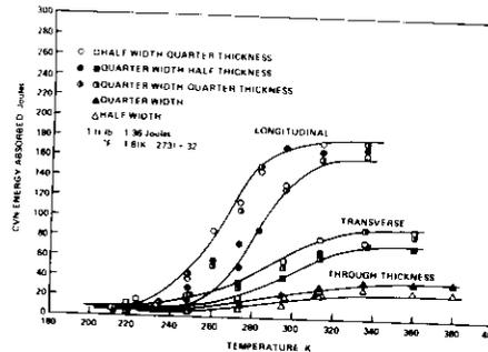
Fig. 6B-2 Charpy V-Notch Energy Curves of Longitudinal, Transverse, and Through-Thickness Specimens of Steel 9 (0.21C, 0.012S).
