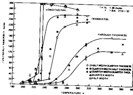
Fig. 6A-1 Charpy V-Notch Impact Energy Curves of Longitudinal, Transverse, and Through-Thickness Specimens of Steel 6 (0.10C, 0.013S, RE).
