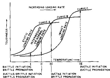
**Fig. 1 Schematic Representation of Various Types of Initiation and Propagation Fracture-Toughness Behavior for Normal Loading Rates.**
