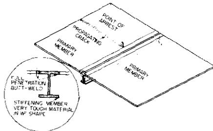
Fig. 2B Schematic showing Out-Of-Plane Crack Arrester
