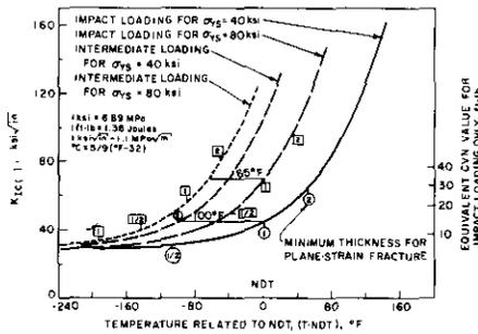
Fig. 4 Estimates of Fracture Toughness for Normal and Extremely High Loading Rates for Two Steels Based Upon ASME  $K_{Ic}$  Reference Curve.
