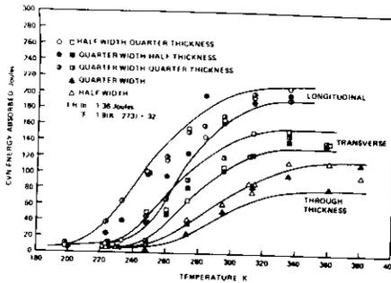
Fig. 6B-1 Charpy V-Notch Impact Energy Curves of Longitudinal, Transverse, and Through-Thickness Specimens of Steel 7 (0.20C, 0.013S, RE).
