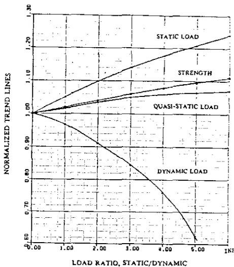
Figure 7 Trends of Partial Safety Factors with the Ratio of Static to Dynamic Loads in TLP Flat Plate Structures.
