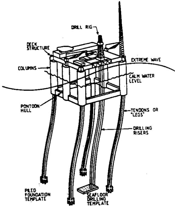
Figure 8 The Tension Leg Platform, the Focus of a Recent Reliability Based Code Development Effort.
