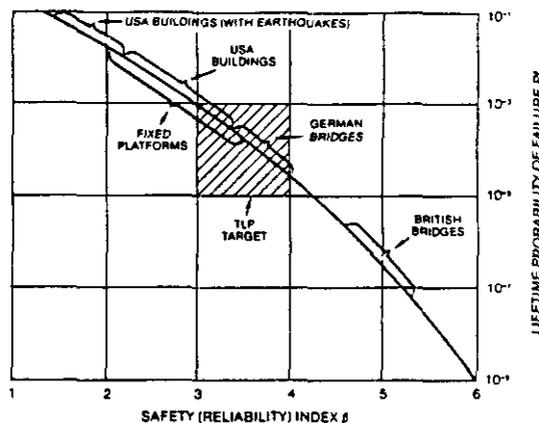
Figure 6 Safety Indices for Various Marine and Land Based Structures.
