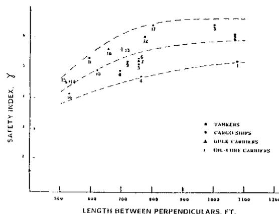
Figure 2 Safety Index for the Hull Girder Strength of 18 Vessels, from an early study by Mansour.
