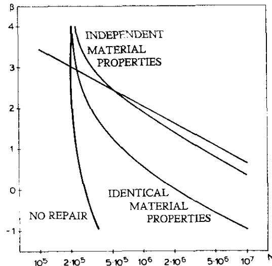
Figure 10. Updated first-order reliability index after repair of an 8 mm crack at  $N=2 \cdot 10^5$  stress cycles.
