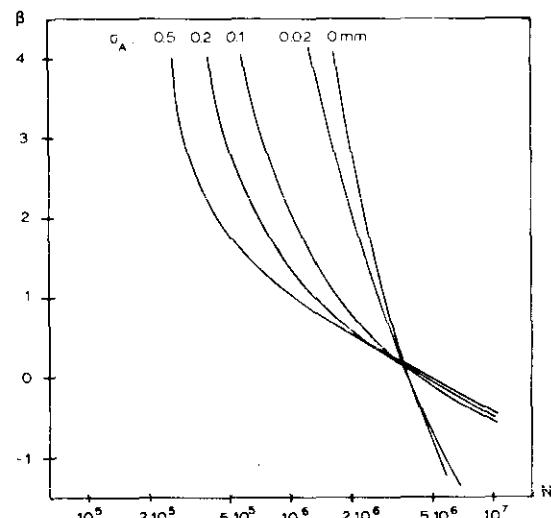
Figure 3. Updated first-order reliability index after second inspection with crack measurements 3.9 mm and 4.0 mm.
