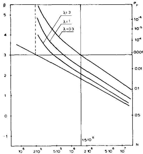
Figure 7. Updated first-order reliability index after first inspection with no crack detection.
