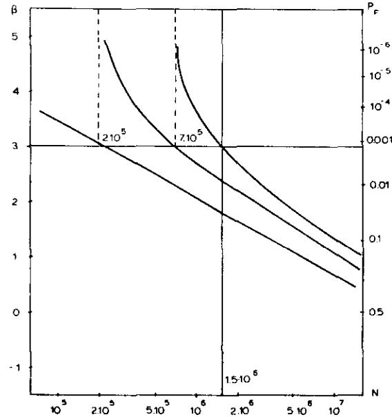
Figure 8. Updated first-order reliability index after inspections with no crack detection, mean size of non-detected cracks 1 mm.
