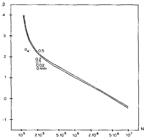
Figure 2. Updated first-order reliability index after first inspection with crack measurement 3.9 mm.
