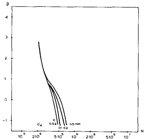
Figure 5. Updated first-order reliability index after second inspection with crack measurements 3.9 mm and 5.0 mm.
