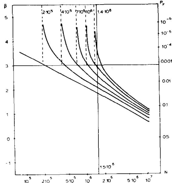
Figure 9. Updated first-order reliability index after inspections with no crack detection, mean size of non-detected cracks 3 mm.
