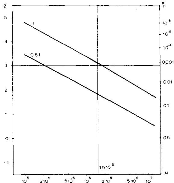
Figure 6. First-order reliability index for two plate thicknesses.
