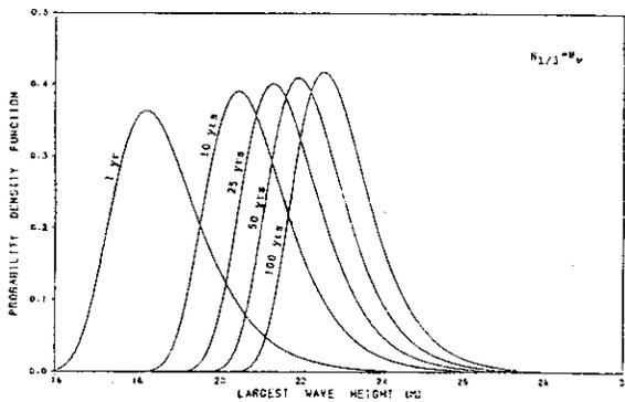
Fig. 9 Probability density function of the largest value of wave height
