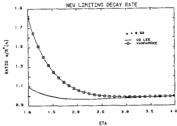
Fig. 4 Comparison of new limiting decay rate and Vanmarcke's at  $q = 0.5$
