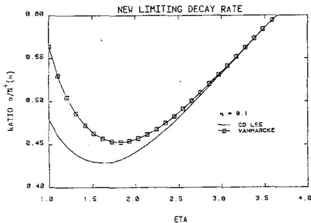
Fig. 3 Comparison of new limiting decay rate and Vanmarcke's at  $q = 0.1$
