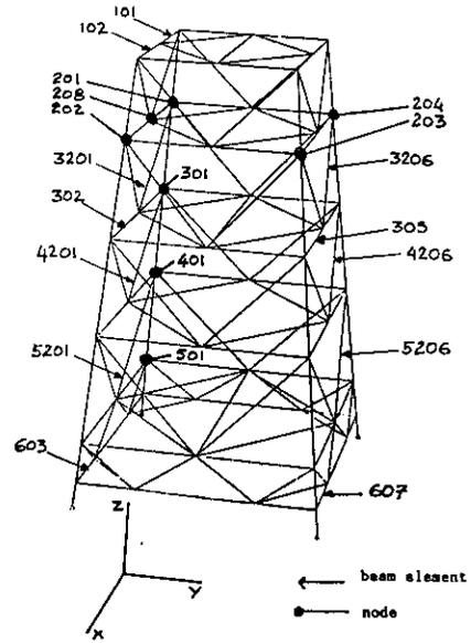
Figure 4 - Simplified finite element model of a small steel-jacket platform
