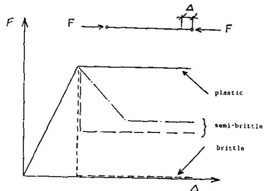
Figure 1 - Possible models of component post failure behaviour
