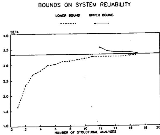
Figure 3 - System reliability bounds versus number of structural reanalyses
