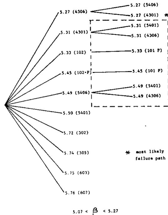
(102 P) : failure of member 102 by plastification
