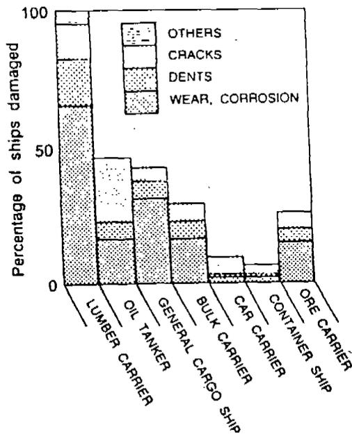
Fig. 1 - Structural damages to ships in 1976-84 (excl. casualties) (taken from [2])
