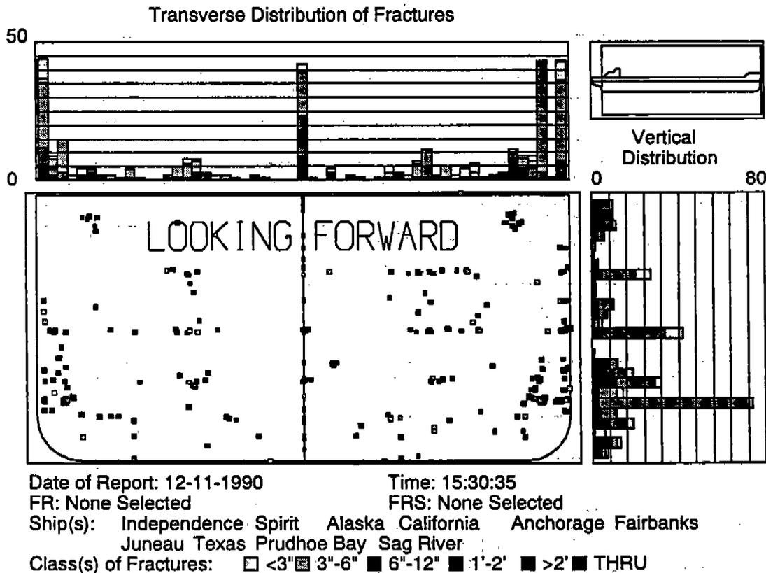
Fig. 6. Transverse distribution of fractures of Alaska Class ships.
