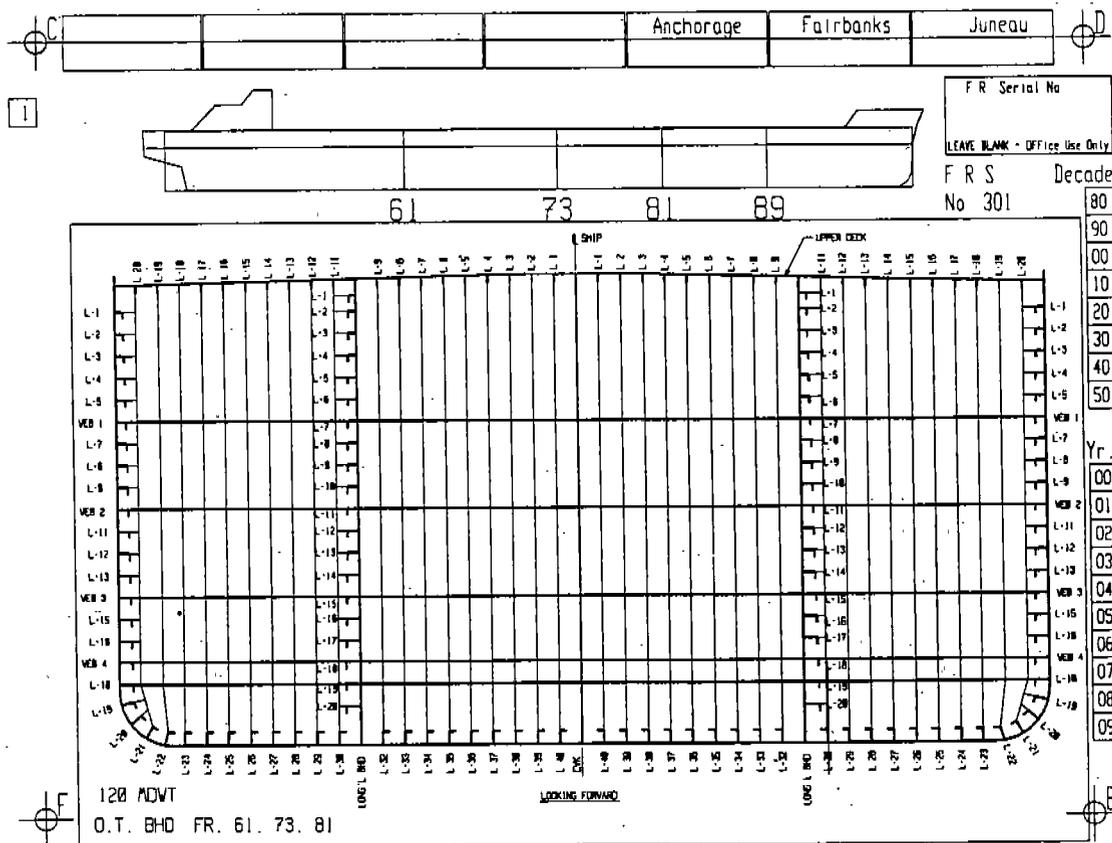
Fig. 1. A generic bulkhead fracture report sheet with a profile auxiliary view.
