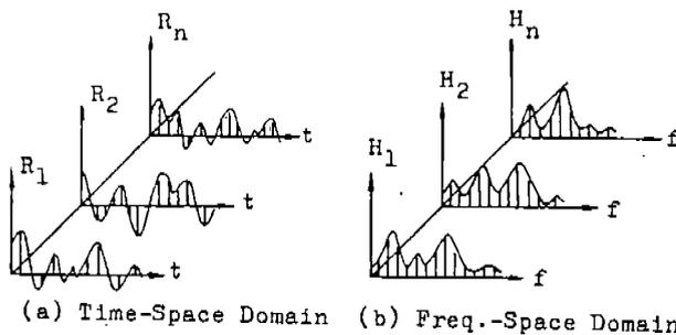
Fig. 3 Feature Vectors From Vibration Signals
