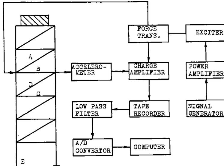
Fig.8 Scheme of the Model and Testing System
