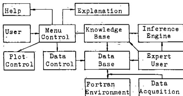
Fig.10 The Structure of Expert System For Damage Detection
