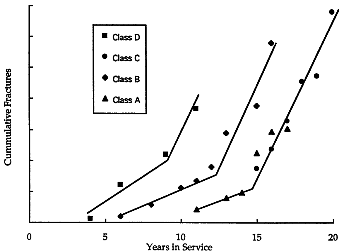
FIGURE 6 Cumulative fractures versus service life for classes A—D.
